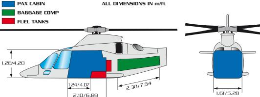
Pilot and passenger cabin 5.10 m<sup>3</sup> Baggage compartment  $0.95 \text{ m}^3$
