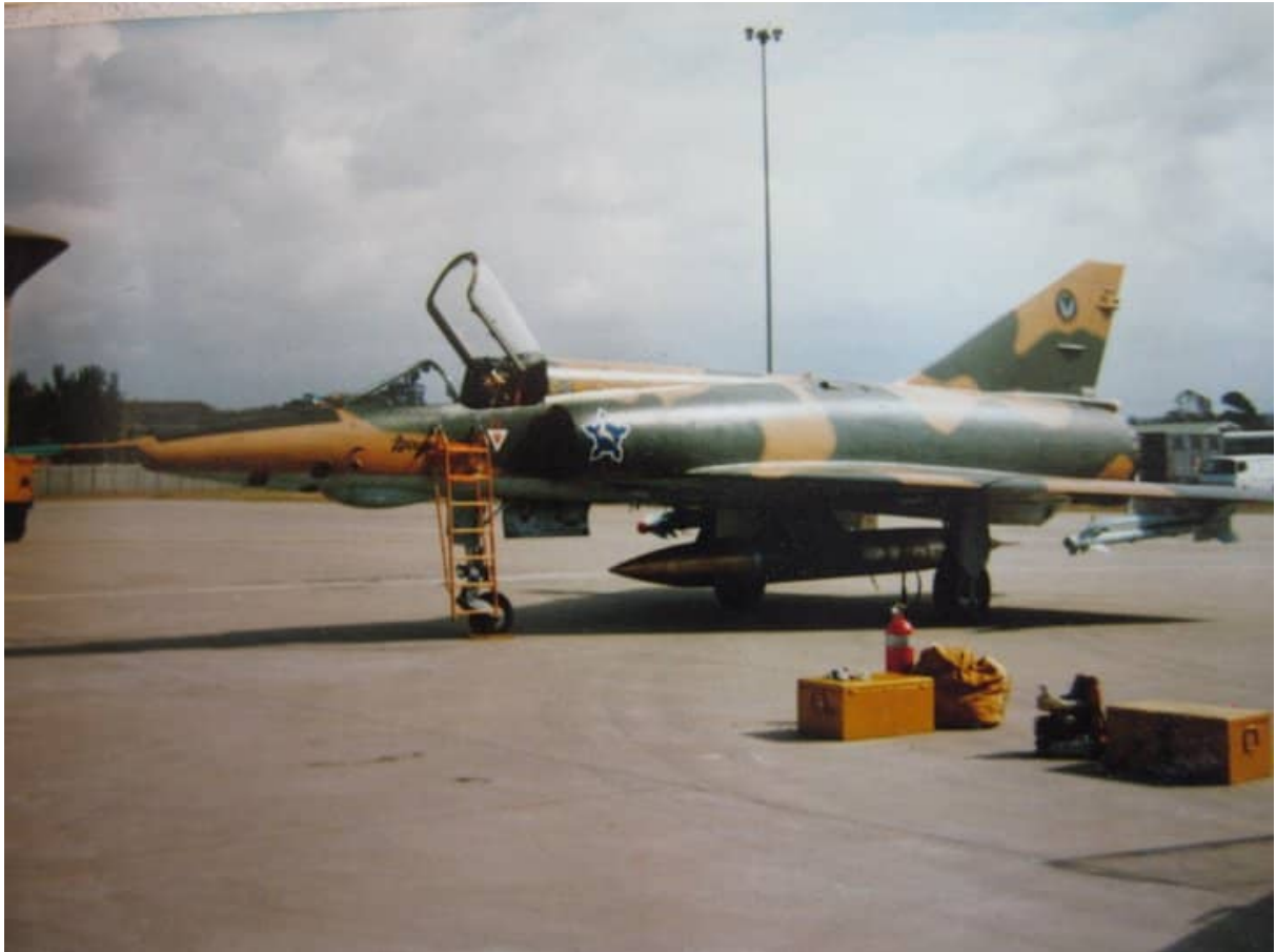
Image RZ-2 – this RZ is carrying an RP825(1) 88- liter fuel tank on the centerline. The missiles are practice V3B items.
