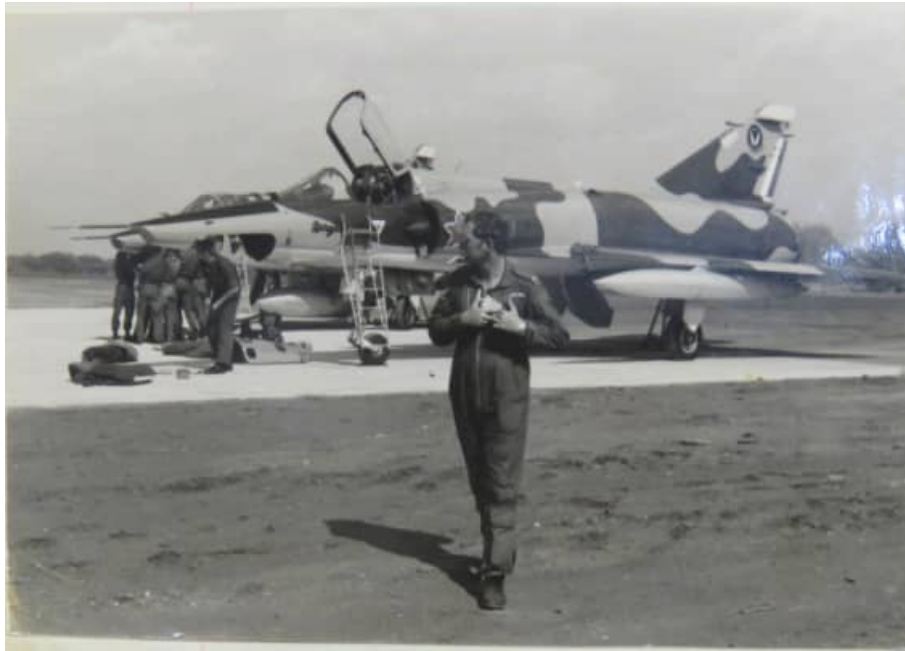
Image R2Z-1 (above) – RZ carrying two of the original French RP18R 500 liter fuel tanks
