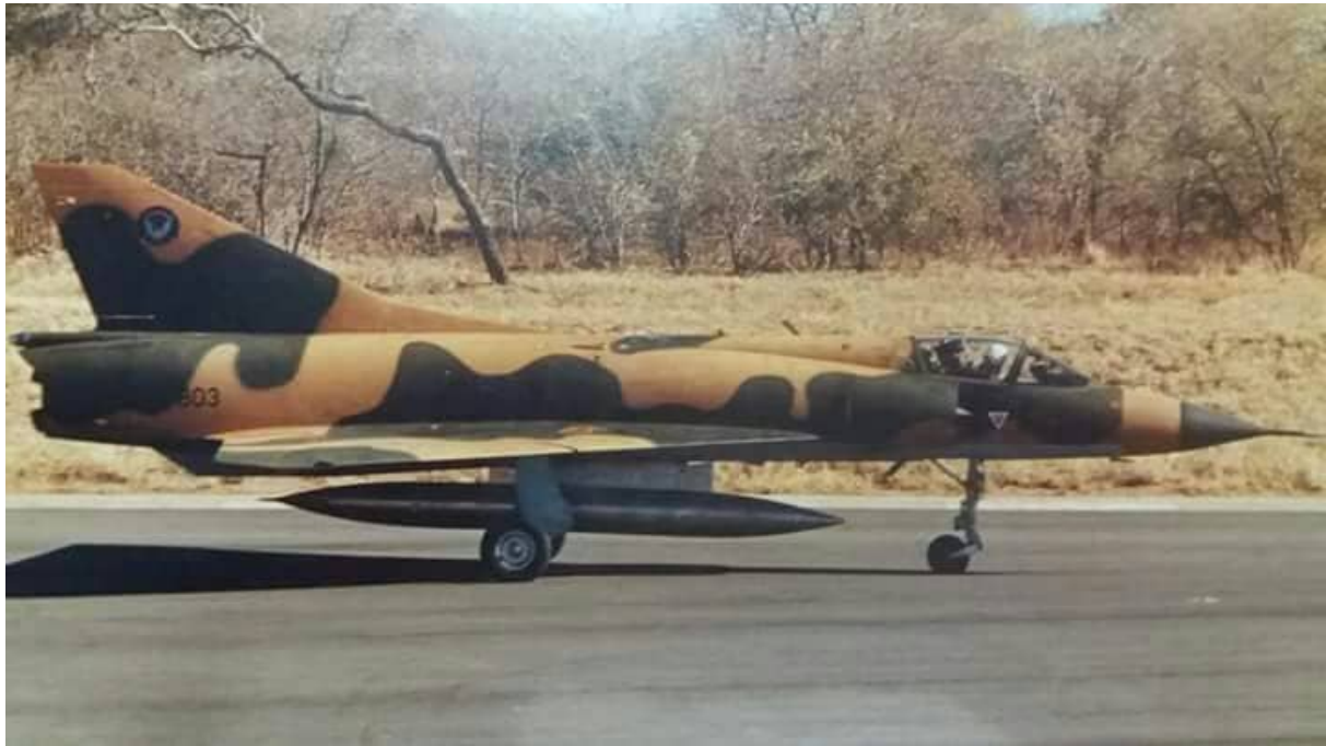
Image CZ-2 - Mirage IIICZ #803 carrying the Israeli designed RP825 825 liter tank on the centerline. Note the distinct downward angle of the tank in relation to the aircraft. Note also the horizontal fins at the rear of the tank. The angle of the leading edge of the tank CRP37 pylon is at right angles to the aircraft underside.
