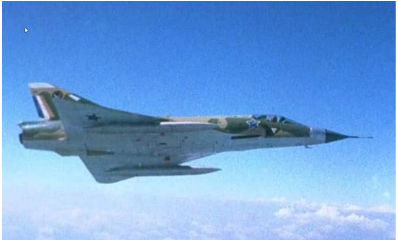
Image CZ-1 - Mirage IIICZ with original French RP18R 500 liter supersonic fuel tanks without fins. Note that the rear of the fuel tank is in line with the elevon hinge line.
