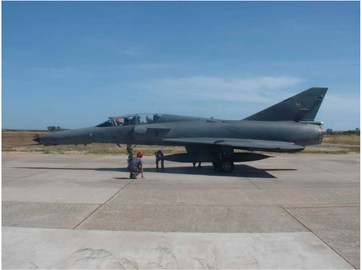
Image D-3 – Cheetah D #853 carrying a centerline RP825(2) 825 liter supersonic fuel tank. Note the raked back leading edge of the CRP-312 tank pylon. These were Israeli designed pylons originally for the Kfir.
