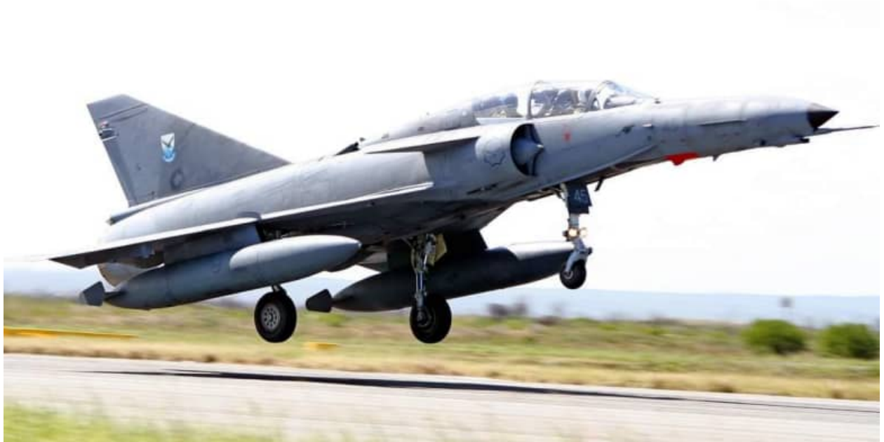
Image D-4 – Cheetah D #845 carrying two RP62 1,300 liter tanks beneath the wings. These are mounted on CRP186 pylons.
