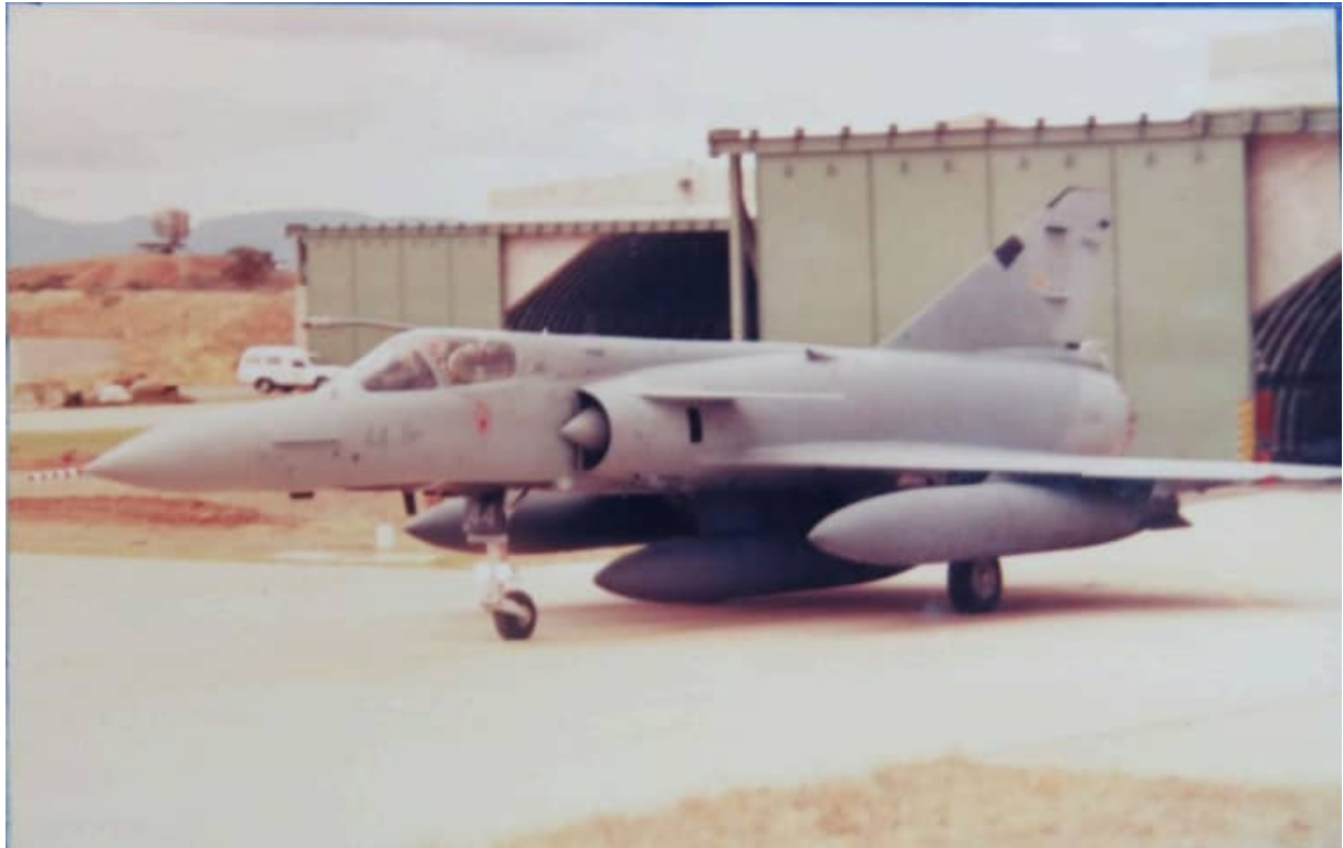
Image C-9 – in this image taken from the 2 Squadron Lines Book, a very substantial external fuel tank fit is seen consisting of two x 1,700 liter wing tanks and a centerline RP62 1,300 liter wing tank. It is unlikely that the Cheetah C could've lifted off with this configuration with full fuel; it's more likely that they would be refueled in air.
