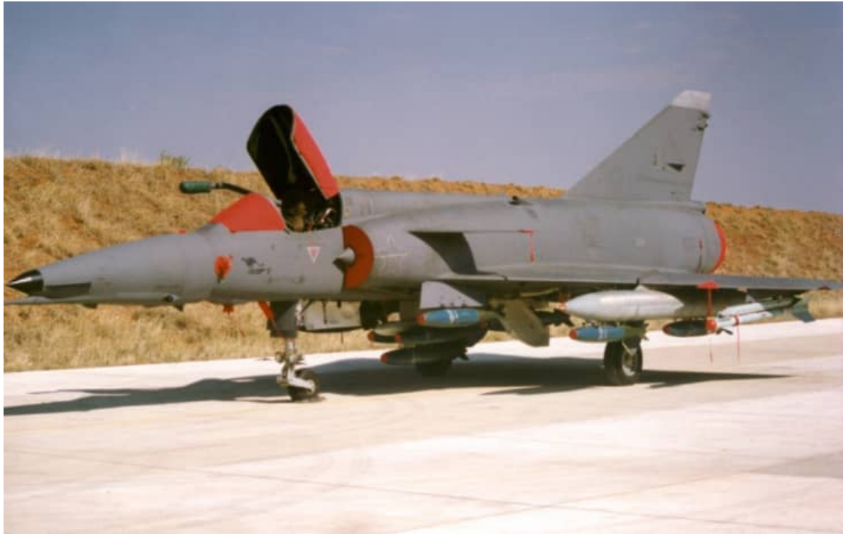
Image E-8 – Another image of Cheetah E #823 carrying two BZ combined fuel tank / bomb carriers. The Triple Ejector Rack on the centerline was not used. The bombs are Mk. 81 250lb (125kg) GP bombs. The missiles are inert V3Bs.
