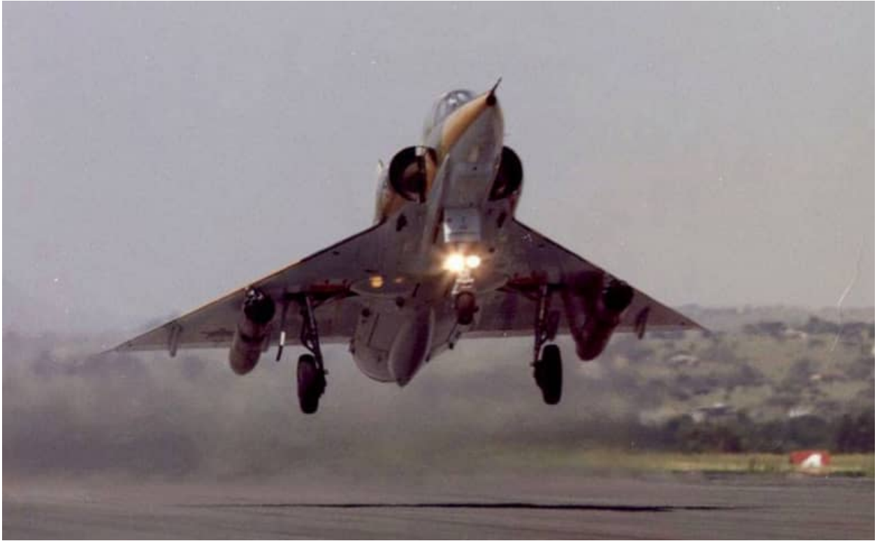
Image DZ-5 – This Mirage IIIDZ is carrying two JL-100 combined fuel tank / rocket pods on the inboard wing stations.
