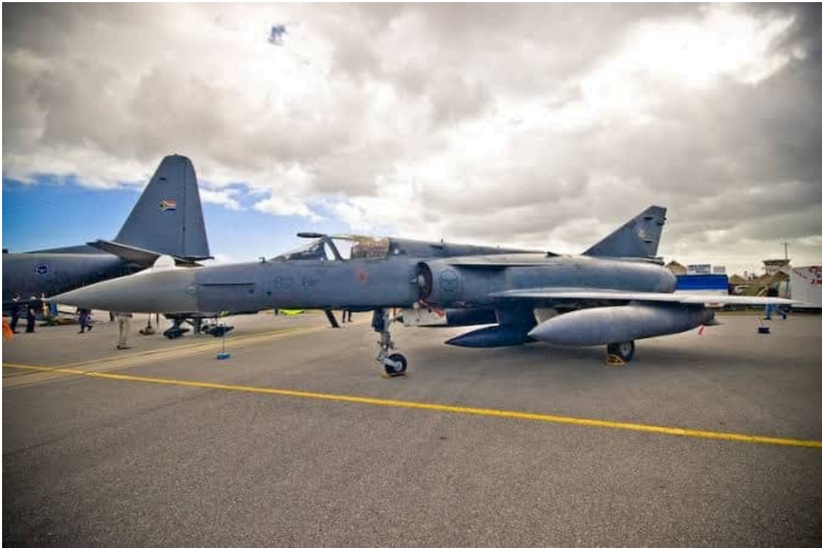
Image C-8 – Cheetah C #382 carrying an RP825(2) 825 liter tank on the centerline and two RP30 1,700 liter tanks on the wings.
