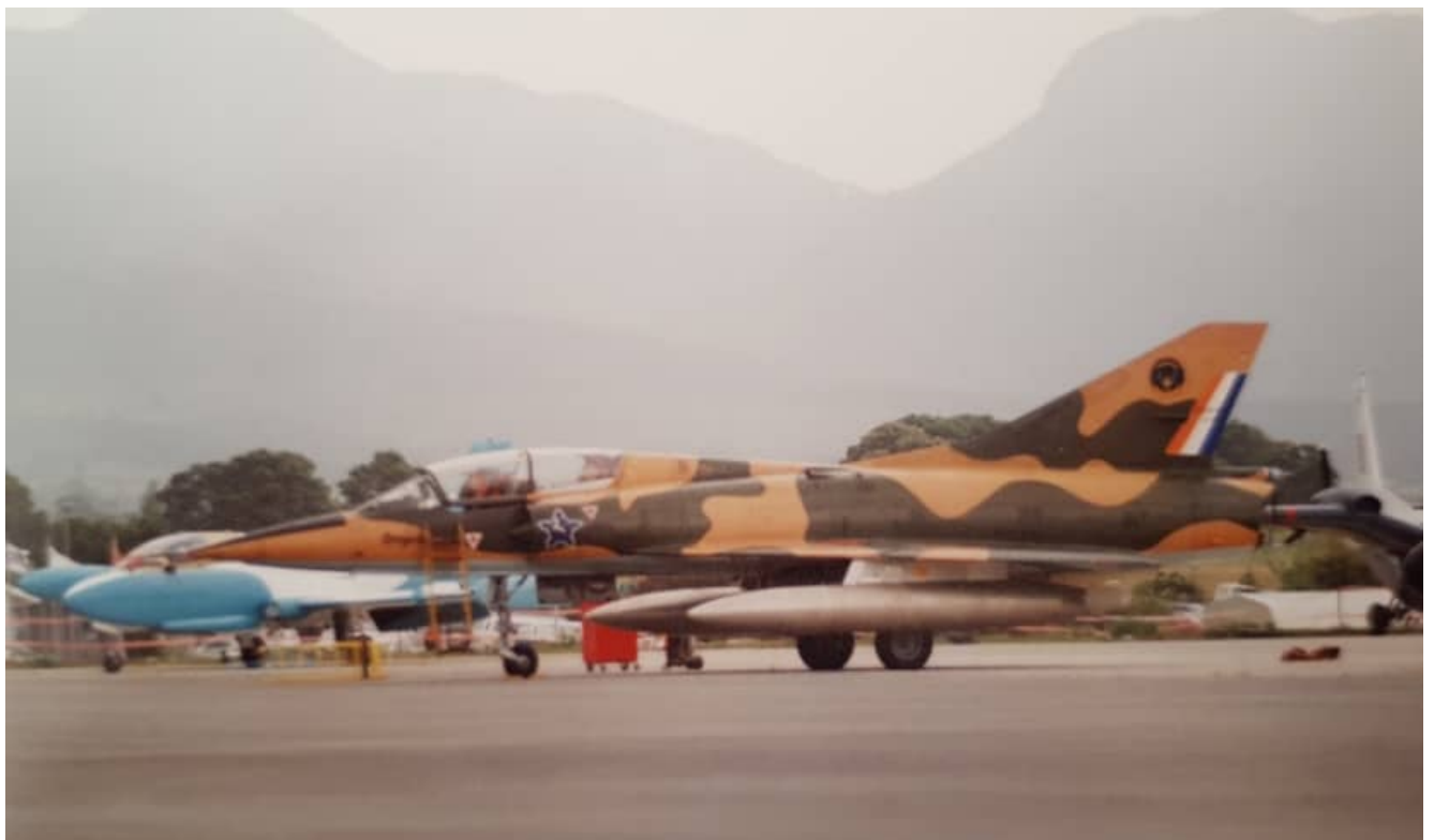
Image BZ-4 - Mirage III BZ #817 carrying two RP62 1,300 liter subsonic fuel tanks on the inboard wing stations.
