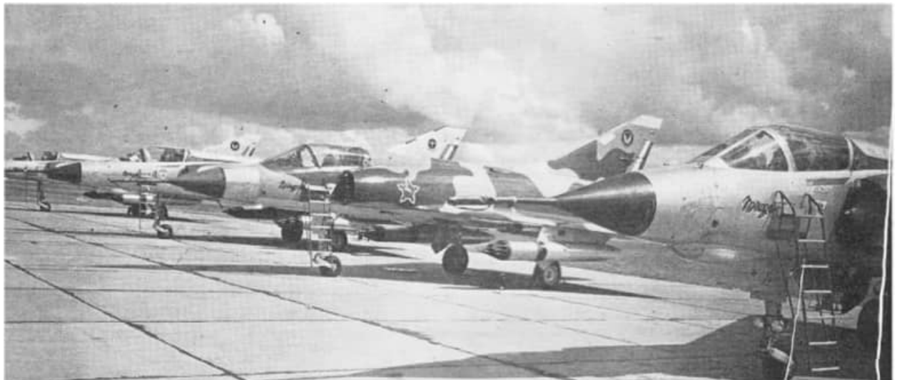
Image CZ-11 – The second Mirage is a CZ and is carrying two JL-100 combined fuel tank / and rocket pods on the inboard wing stations.
