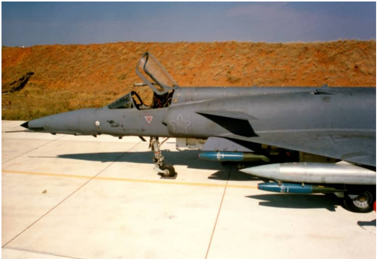
Image E-7 – Cheetah E #823 carrying two BZ combined fuel tank / bomb carriers beneath the wings.
