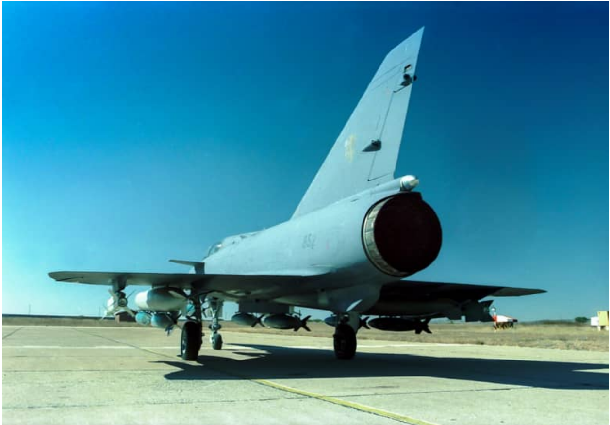
Image D-7 and D-8 – Cheetah Ds (#852 above) carrying two RPK combined fuel tank / bomb carriers on the inboard wing stations.
