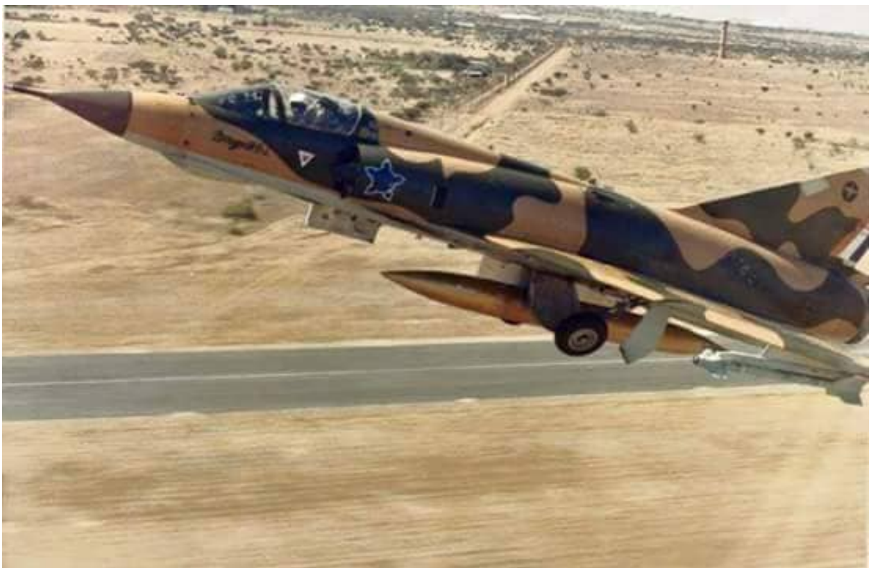
Image EZ-3 – This EZ is carrying a single RP825(1) 880 liter tank on the centerline station. The missiles are practice V3B air to air missiles.
