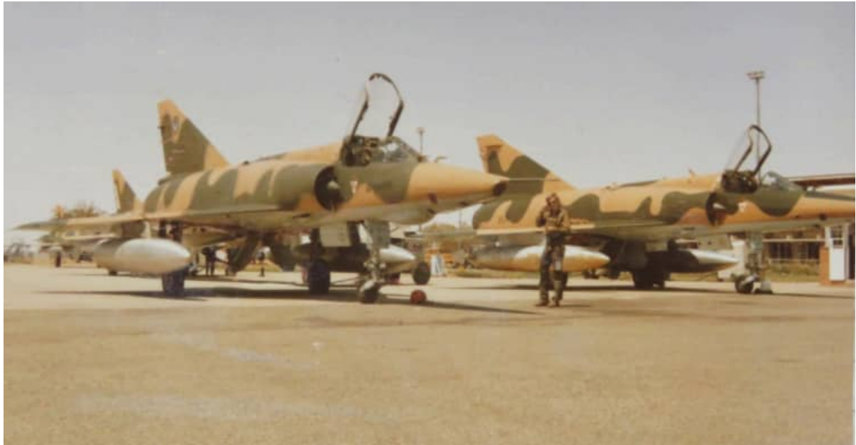
Image RZ-4 – the RZ on the left is carrying two of the French RP62 1,300 liter subsonic fuel tanks. The R2Z on the right is carrying a similar load.
