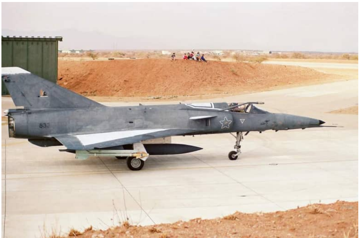
Image E-2 and E-3 – Cheetah Es carrying centerline RP825(1) 880 liter fuel tanks. Note in the image below that this is the original CRP37 centerline pylon as used on Mirage IIIs which has a vertical leading edge. The missiles are practice V3Bs.
