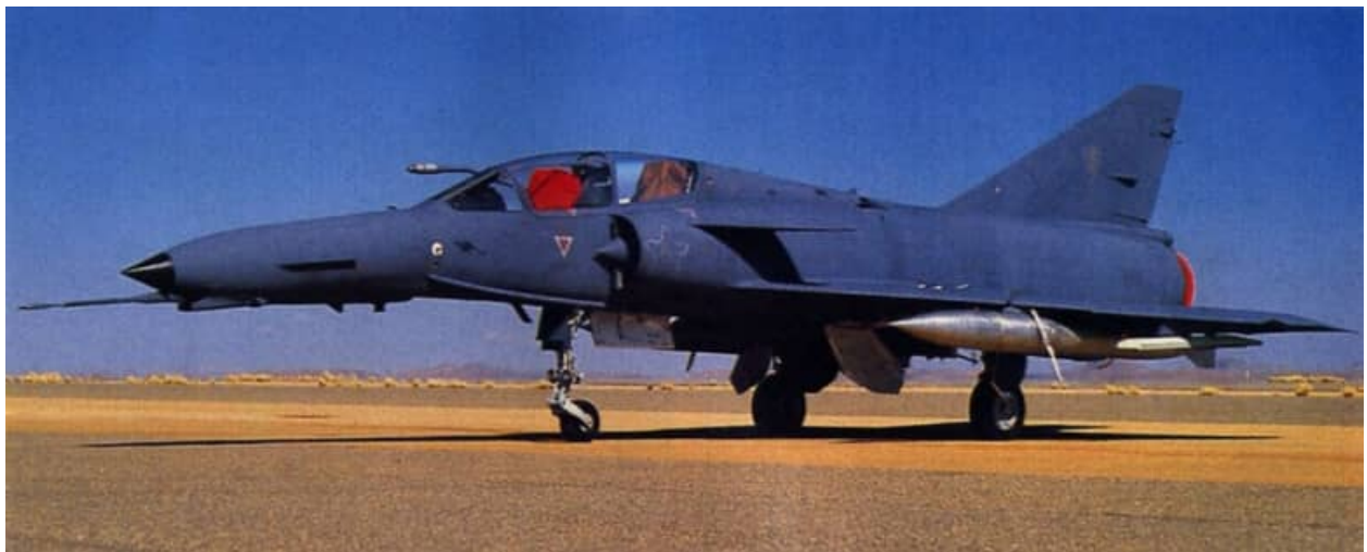
Image D-1 and D-2 – Cheetah D #853 (above) and another (below) carrying two finned AZ 500 liter fuel tanks
