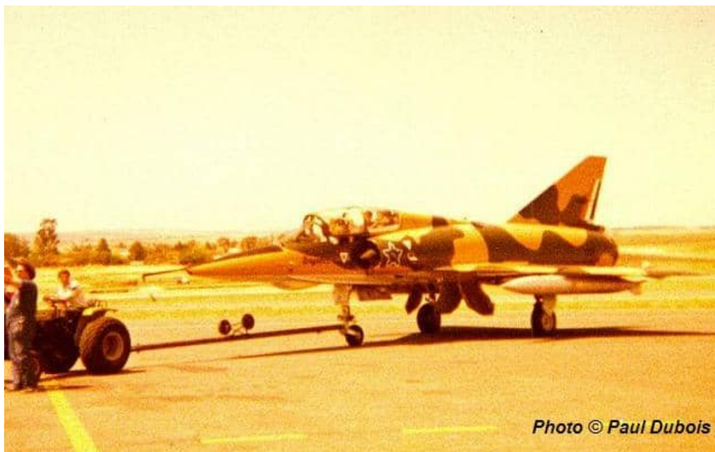
Image DZ-2 – This Mirage IIIDZ is carrying two of the Israeli finned AZ 500 liter fuel tanks.
