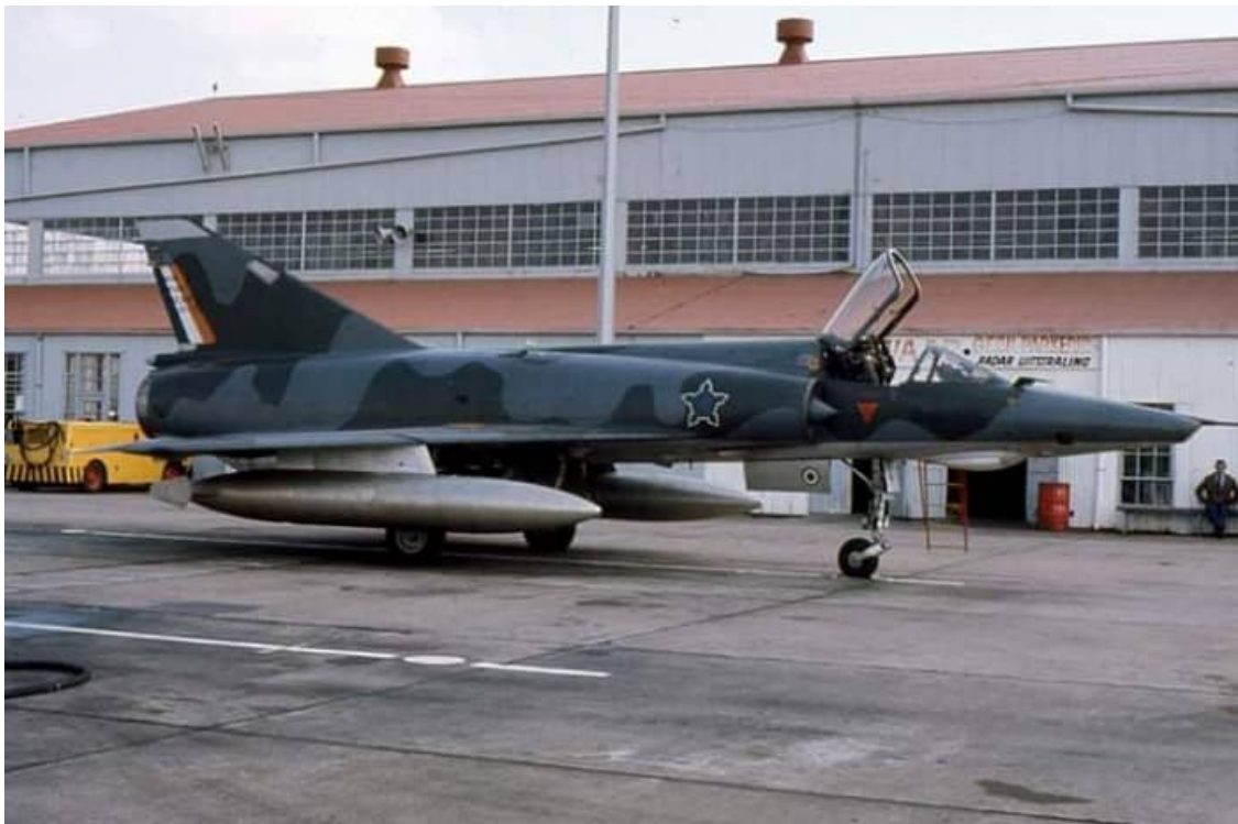
Image RZ-3 – this RZ is carrying two of the French RP62 1,300 liter subsonic fuel tanks under the wings.
