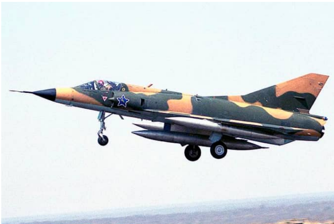
Image CZ-5 - Mirage IIICZ #806 is carrying two AZ fuel tanks on the wing stations and one centerline RP825(1) 880 liter fuel tank. Both tank types could be used for supersonic flight, but it's unlikely that the CZ could achieve supersonic flight with all three installed.
