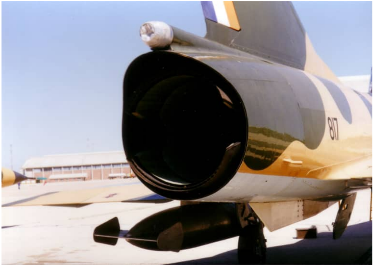
Image BZ-5 (below) – details of RP62 fuel tank fin arrangement (BZ #817).
