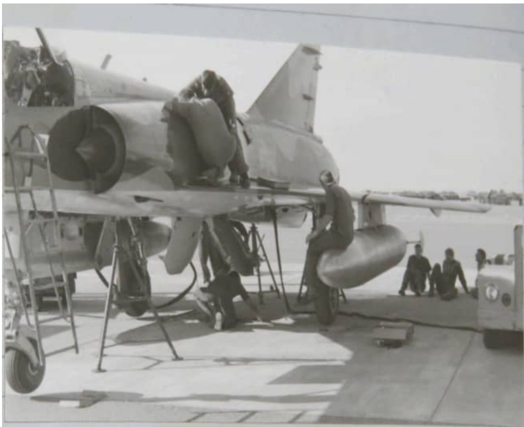
Image R2Z-4 – Another R2Z carrying two RP62 1,300 liter fuel tanks. This aircraft can be identified as an R2Z by the scalloped (curved) intake splitter plates.
