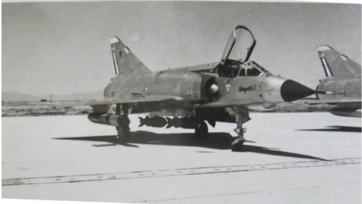
Image EZ-6 – This EZ is carrying two JL-100 combined fuel tank and rocket pods on the wings and two 400kg bombs in tandem on the centerline PM-3 bomb beam.
