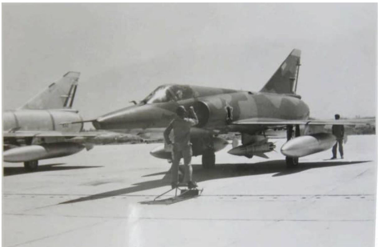
Image RZ-5 – this RZ is carrying two of the French RP62 1,300 liter subsonic fuel tanks under the wings and an AS-30 laser guided air to surface missile on the centerline. The centerline pylon looks like the standard CRP37 used to carry the RP825 fuel tank.
