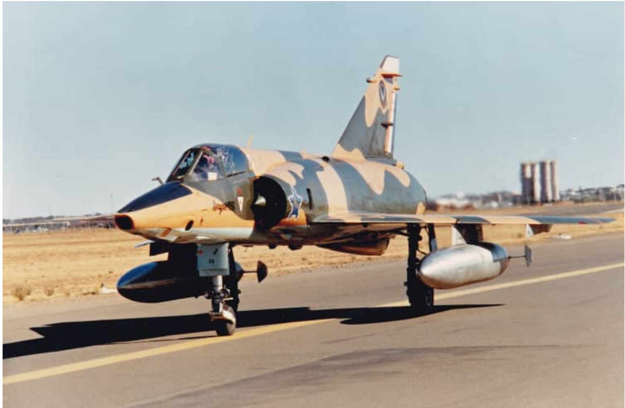
Image R2Z-3 – R2Z carrying two RP62 1,300 liter fuel tanks.
