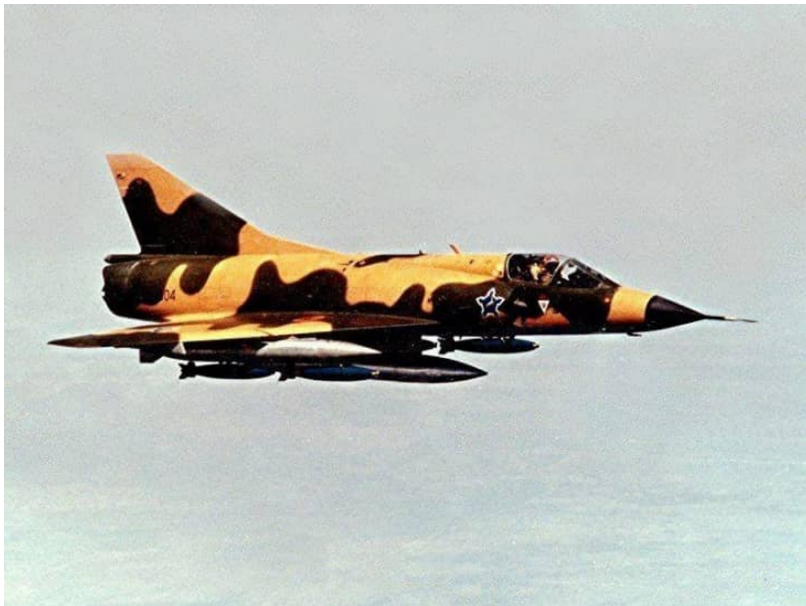
Image CZ-6 – Mirage IIICZ, #805 (above) and #804 (below) are carrying two BZ combination 500 liter tank / dual bomb carriers (with 2 bombs each) on the wing inboard stations and an RP825(1) 880 liter tank on the centerline. This was a typical combat load which saw operational service over Angola in the 1980s. These images were likely taken at AFB Hoedspruit. The bombs in the image below are blue indicating practice bombs, either Mk.81 (250lb) or Mk.82 (500lb).
