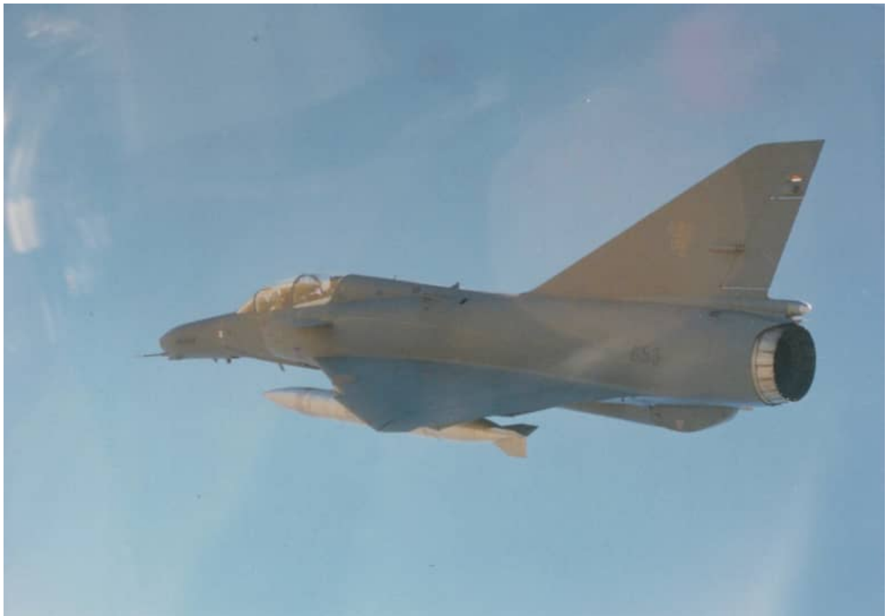
Image D-1 and D-2 – Cheetah D #853 (above) and another (below) carrying two finned AZ 500 liter fuel tanks
