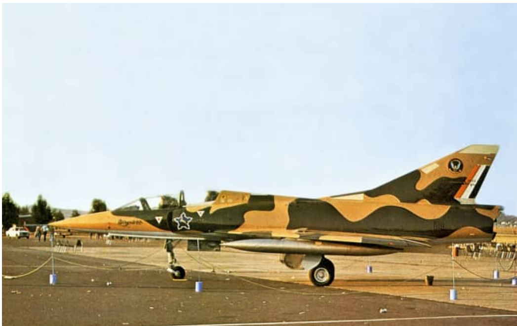
Image BZ-1 and BZ-2 – two images of Mirage IIIBZ #818 with original French RP18R 500 liter supersonic fuel tanks. These tanks do not have the rear fins.
