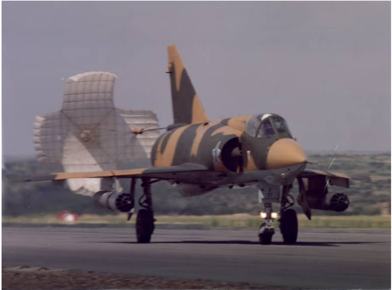
Image EZ-5 – EZ #827 is carrying two JL-100 combined fuel tank and rocket pods on the wings.
