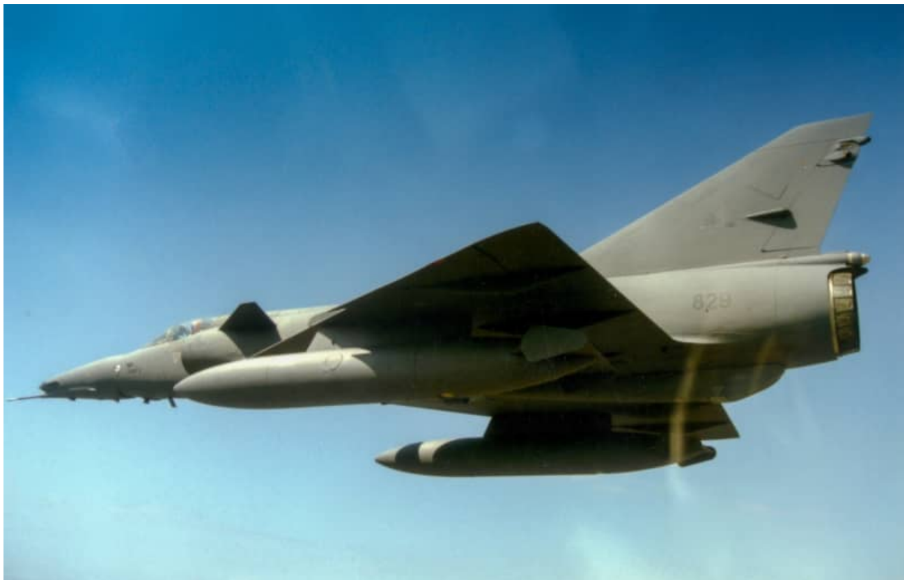
Image E-4 and E-5 – Cheetah Es carrying two RP62 1,300 liter subsonic wing tanks. Note the fins with end plates at the rear of the tanks.
