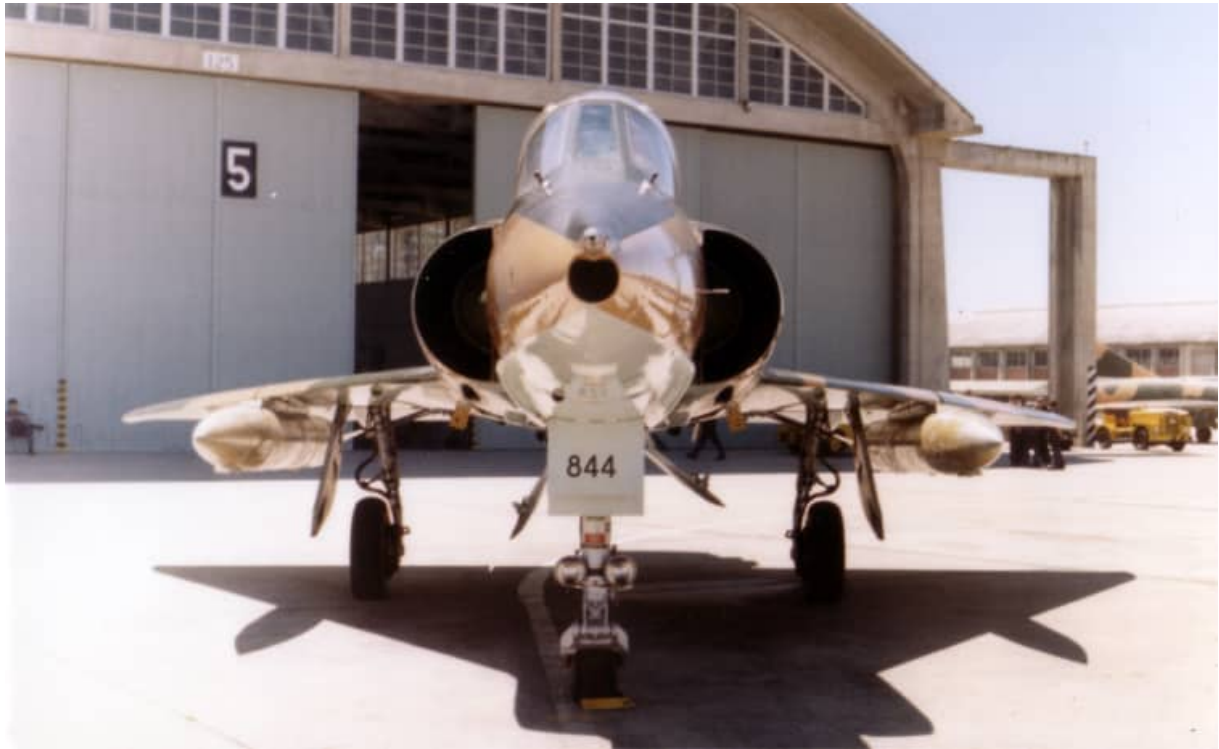
Image D2Z-3 – Mirage IIIDZ #844 is carrying two of the Israeli finned RPK18R 500 liter combined fuel tanks / bomb carrier – the shackles are just visible in the images above and below.
