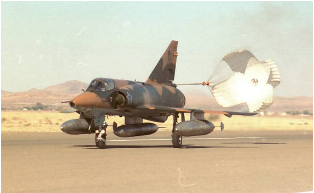
Image RZ-6 – this RZ is carrying an RP825(1) 880 liter centerline fuel tank as well as two RP62 1,300 liter tanks on the wings.
