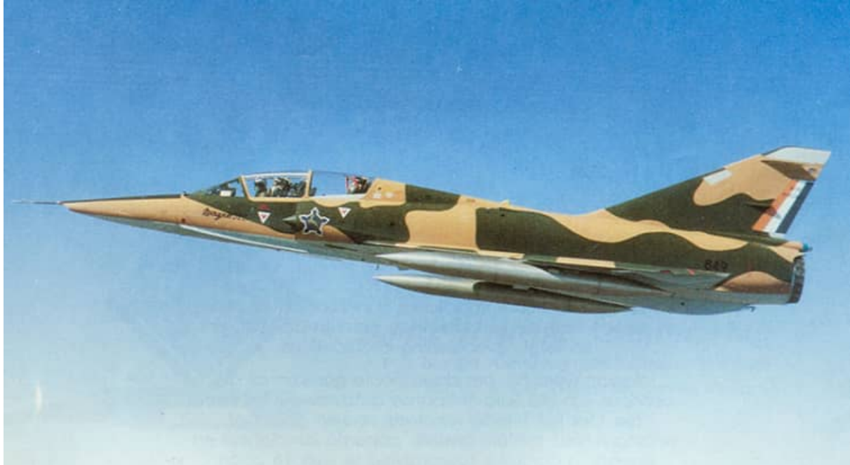
Image D2Z-1 – This Mirage IIID2Z #849 is carrying two of the original French finless RP18R 500 liter fuel tanks. The D2Z does not have the prominent doppler radar antennae fairing beneath the nose as is the case for the DZ.
