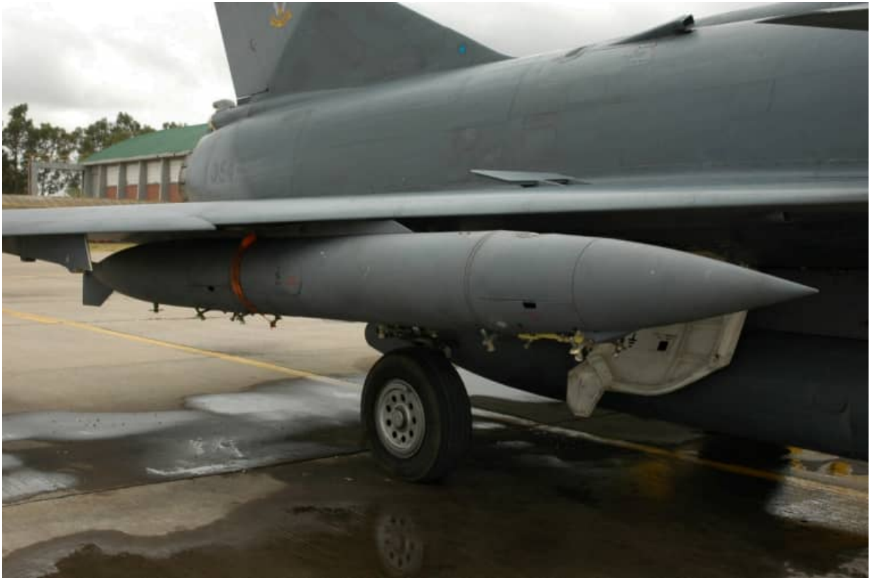
Image C-7 – Cheetah C #354 carrying an RP62 1,300 liter tank on the centerline station and two RPK combined fuel tank / bomb carriers beneath the wings.
