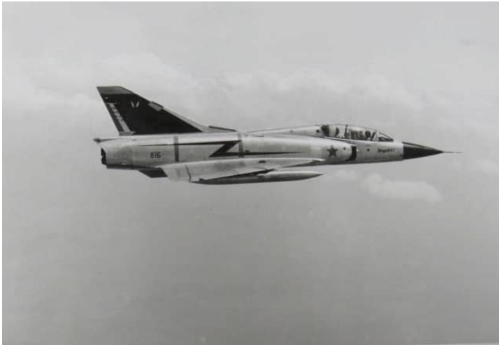
Image BZ-1 and BZ-2 – two images of Mirage IIIBZ #818 with original French RP18R 500 liter supersonic fuel tanks. These tanks do not have the rear fins.
