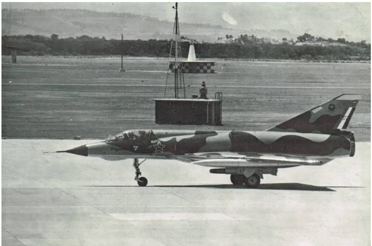
Image EZ-1 – This EZ is carrying two of the original French RP18R finless 500 liter fuel tanks on the wings.
