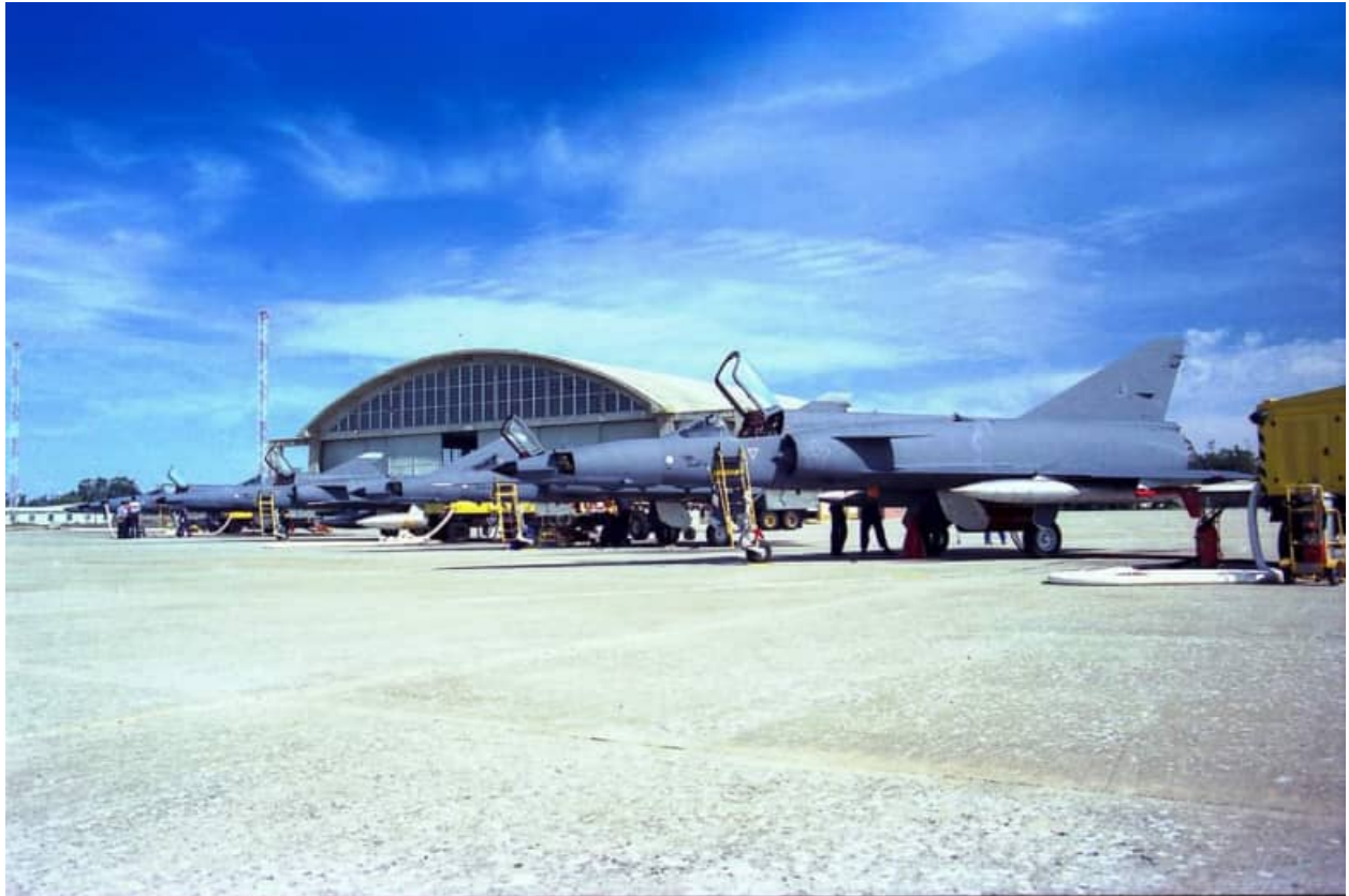
Image E-1 – Cheetah E in the foreground is carrying two Israeli designed finned AZ 500 liter supersonic fuel tanks on the wing stations. The third Cheetah E is carrying RP62 1,300 liter fuel tanks.
