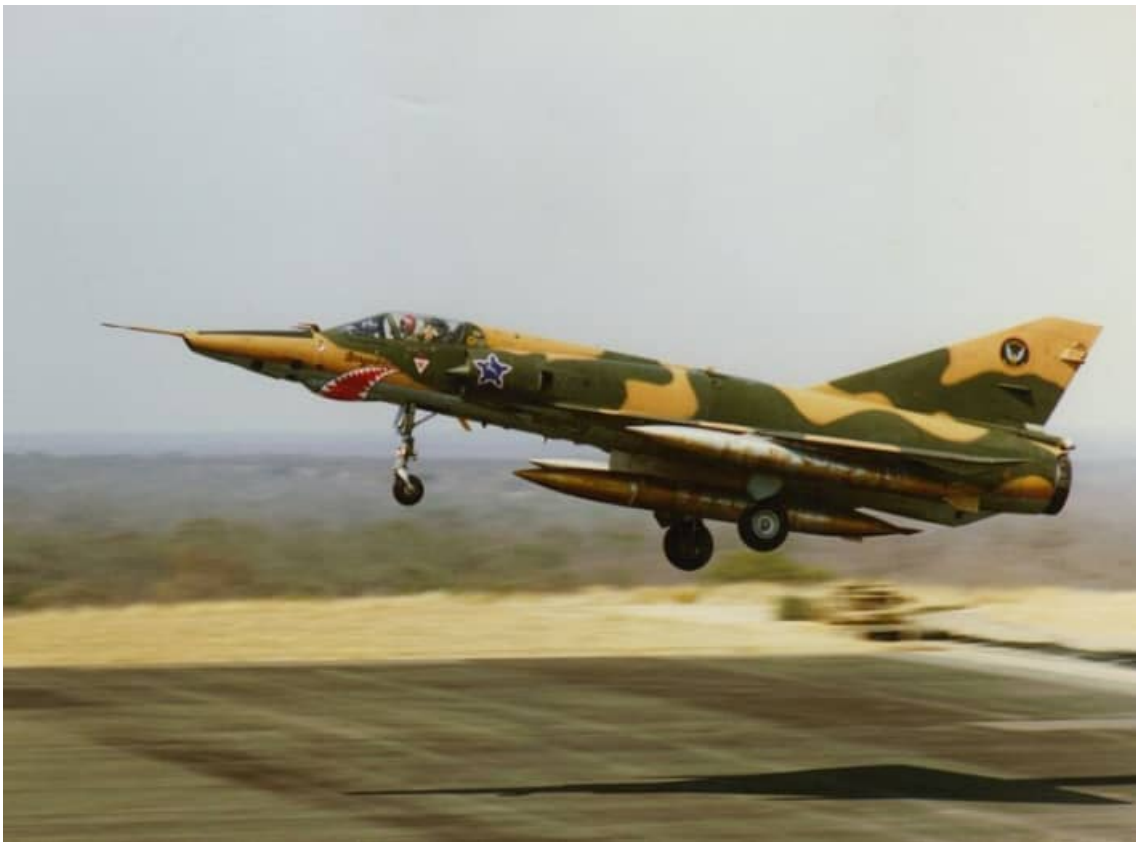
Image RZ-7 – this RZ is carrying an RP825(1) 880 liter centerline fuel tank as well as two of the Israeli designed finned AZ fuel tanks on the wing stations. Note the weathered orange coating on two of the tanks.
