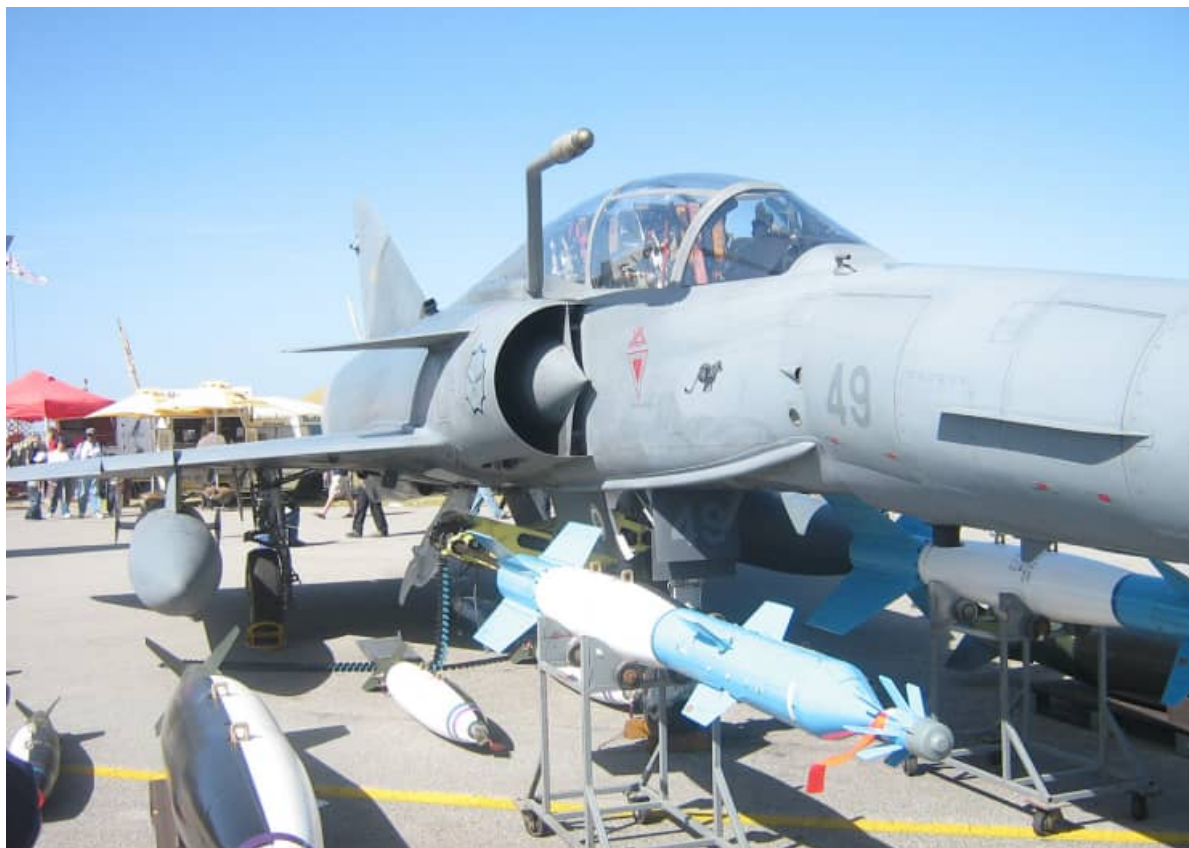
Image D-5 – Cheetah D #849 carrying two RP62 1,300 liter wing tanks. Note that the tanks and pylons are canted outwards away from the main landing gear. This is typical for all Mirage and Cheetah aircraft carrying the RP62.
