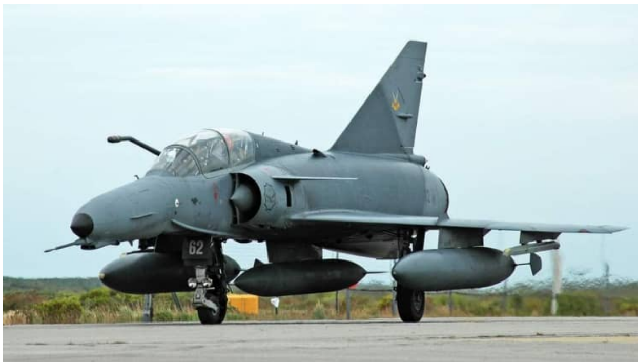
Image D-6 – Cheetah D #862 carrying an RP825(2) 825 liter fuel tank on the centerline and two RP62 1,300 liter tanks on the inboard wing stations.
