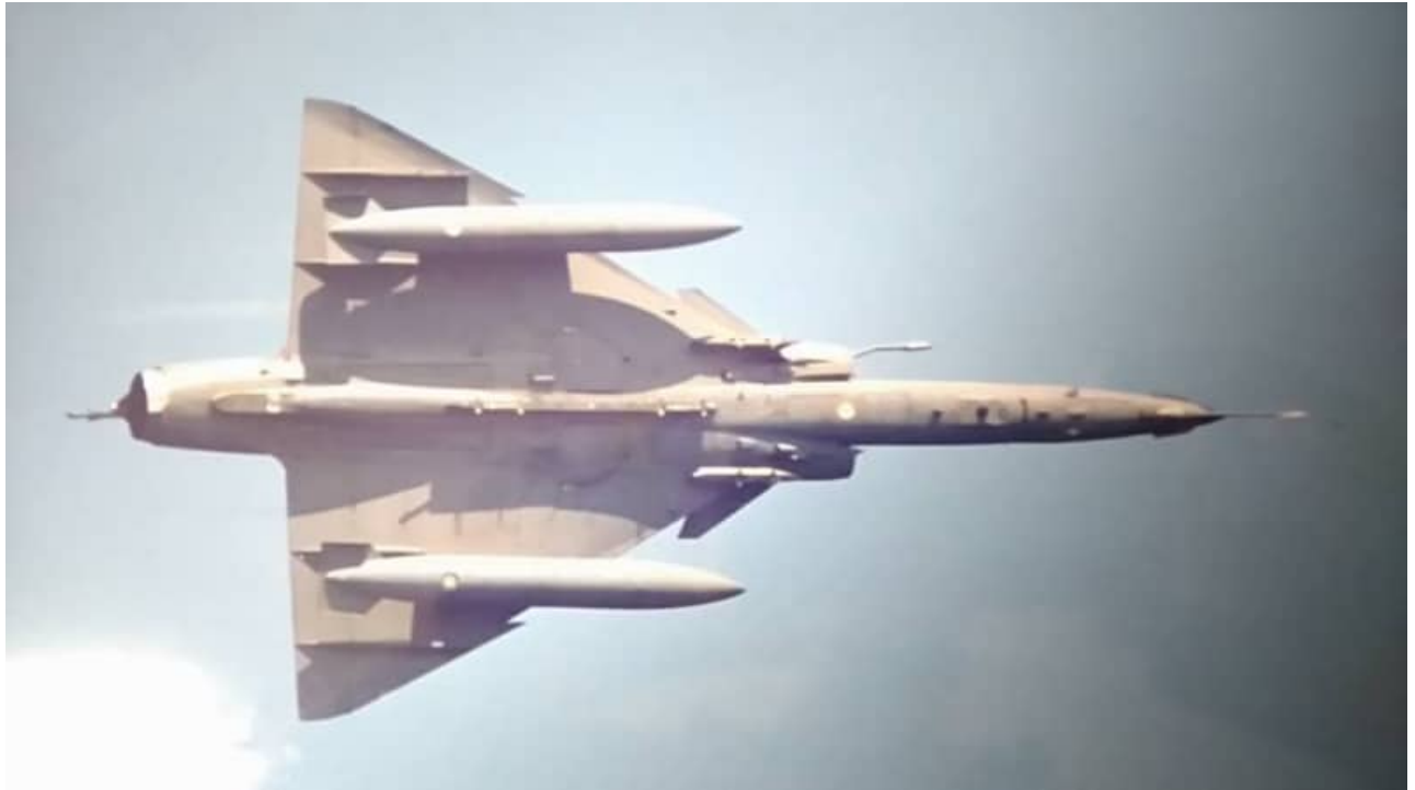
Image E-4 and E-5 – Cheetah Es carrying two RP62 1,300 liter subsonic wing tanks. Note the fins with end plates at the rear of the tanks.
