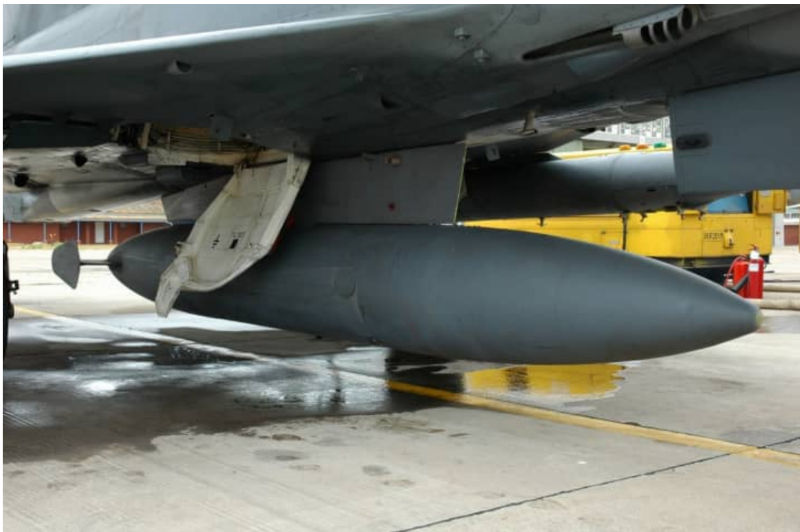
Image C-10 – close up view of RP62 1,300 liter tank on Cheetah C centerline. Note swept back leading edge of the CRP-372 pylon.
