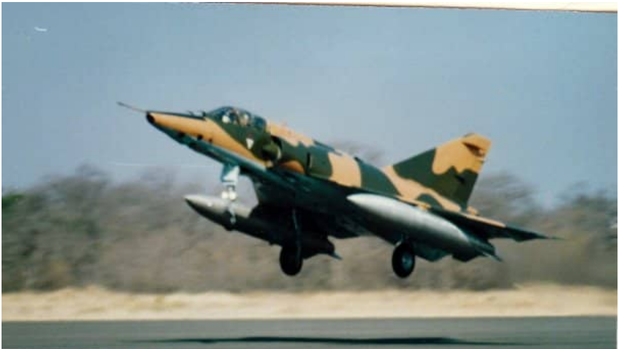
Image R2Z-6 – Another unidentified R2Z (possibly #857), this time carrying two RP30 1,700 liter fuel tank under the wings. Note the downward slant of the tank fins.
