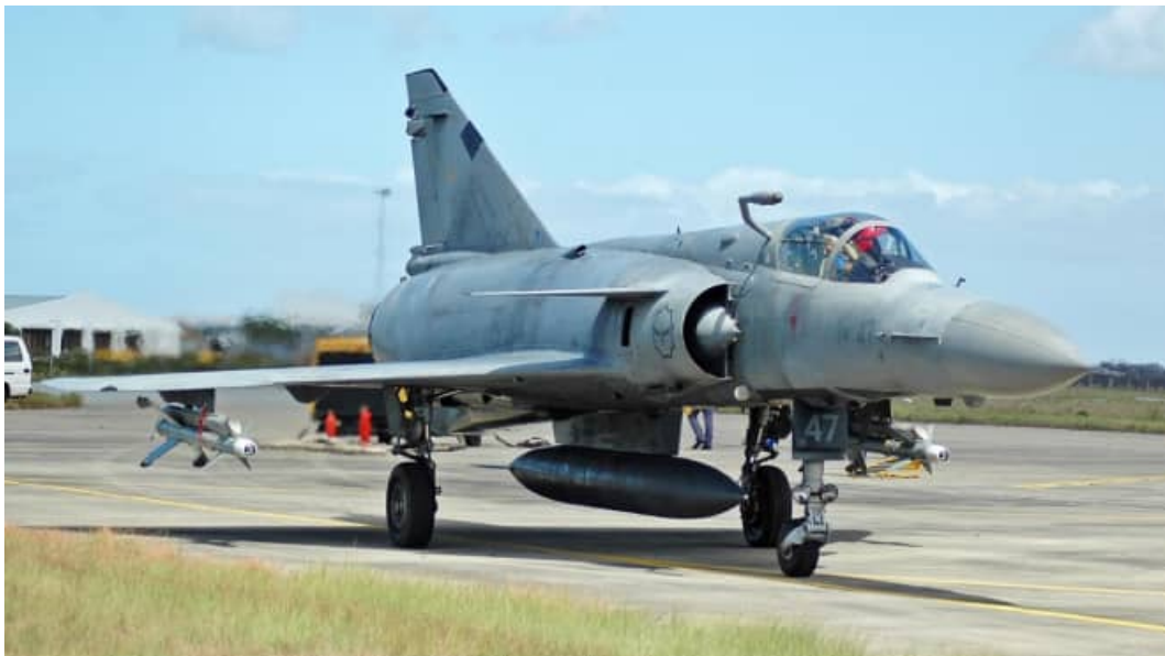
Image C-1 and C-2 – Cheetah Cs (#359 above and #347 below) carrying an RP825(2) 825 liter tank on the centerline station. The pylon for this tank was designated CRP-312. The missiles in the image above are the V4 Derby and in the image below are the V3S Python.
