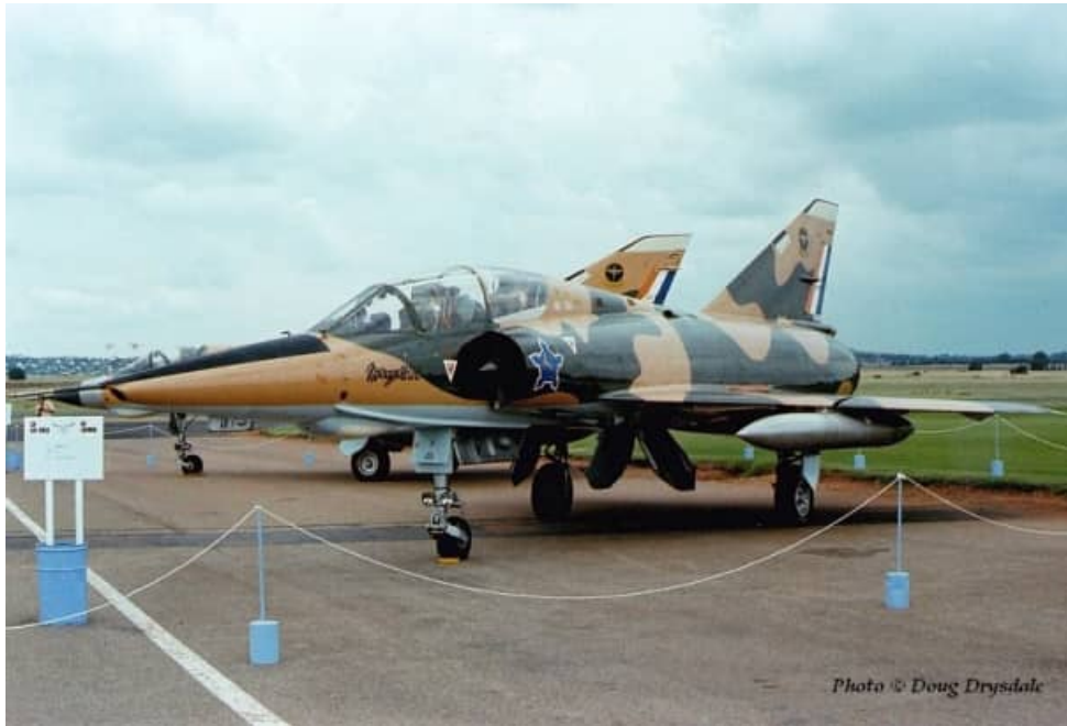
Image DZ-1 – Mirage IIIDZ #840 is carrying two of the original French finless RP18R 500 liter fuel tanks. The DZ can be distinguished from the similar D2Z by the prominent doppler radar antennae fairing beneath the cockpit just ahead of the nose landing gear.
