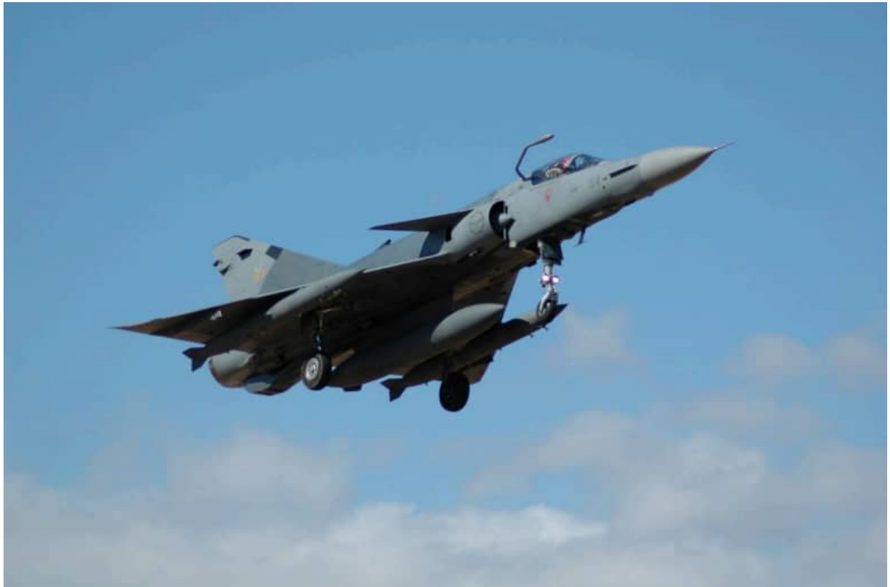
Image C-5 – Cheetah C #354 carrying an RP62 1,300 liter tank on the centerline and two RPK combined fuel tank / bomb carriers beneath the wings. Note the bomb shackles on the BZ tanks.
