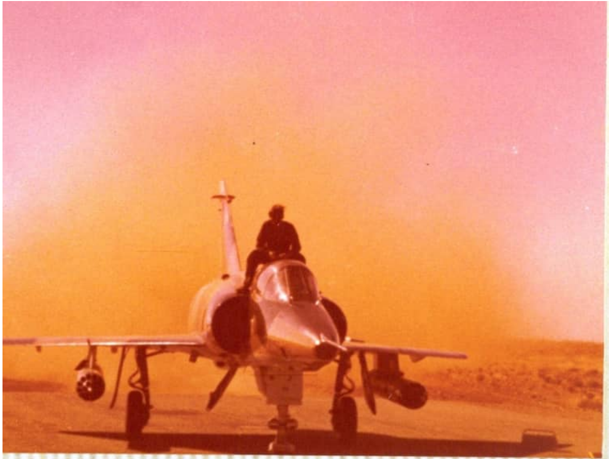
Image R2Z-7 – R2Z carrying two JL-100 rocket pods beneath the wings. This would likely not be a common load for a reconnaissance Mirage.
