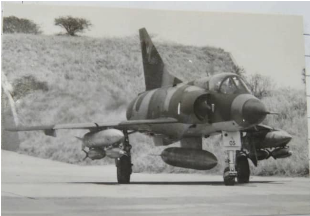
Image CZ-6 – Mirage IIICZ, #805 (above) and #804 (below) are carrying two BZ combination 500 liter tank / dual bomb carriers (with 2 bombs each) on the wing inboard stations and an RP825(1) 880 liter tank on the centerline. This was a typical combat load which saw operational service over Angola in the 1980s. These images were likely taken at AFB Hoedspruit. The bombs in the image below are blue indicating practice bombs, either Mk.81 (250lb) or Mk.82 (500lb).
