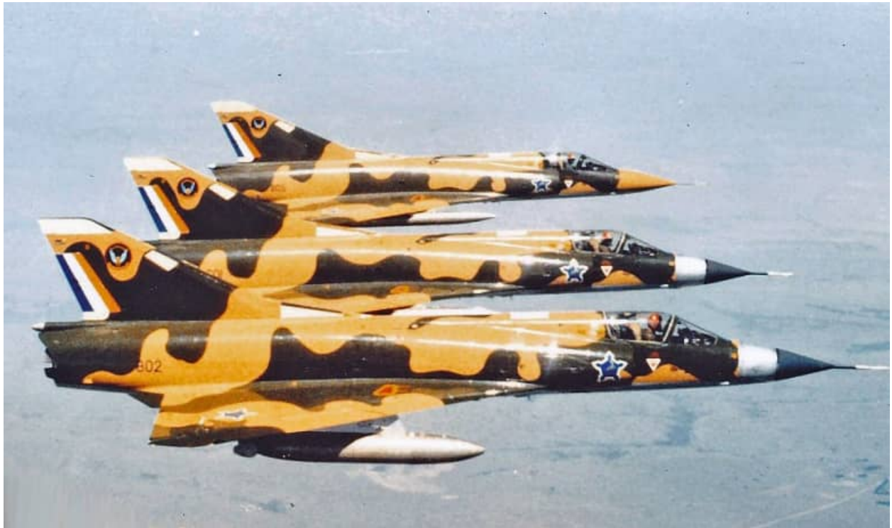
Image CZ-10 –Mirage IIICZ #802 in the foreground is carrying the early French subsonic 600 liter wing tanks. They appear similar in configuration to the RP62 tanks, but are significantly shorter and smaller in diameter. Compare these to the RP62s in the previous image. The third aircraft is carrying RP18Rs.
