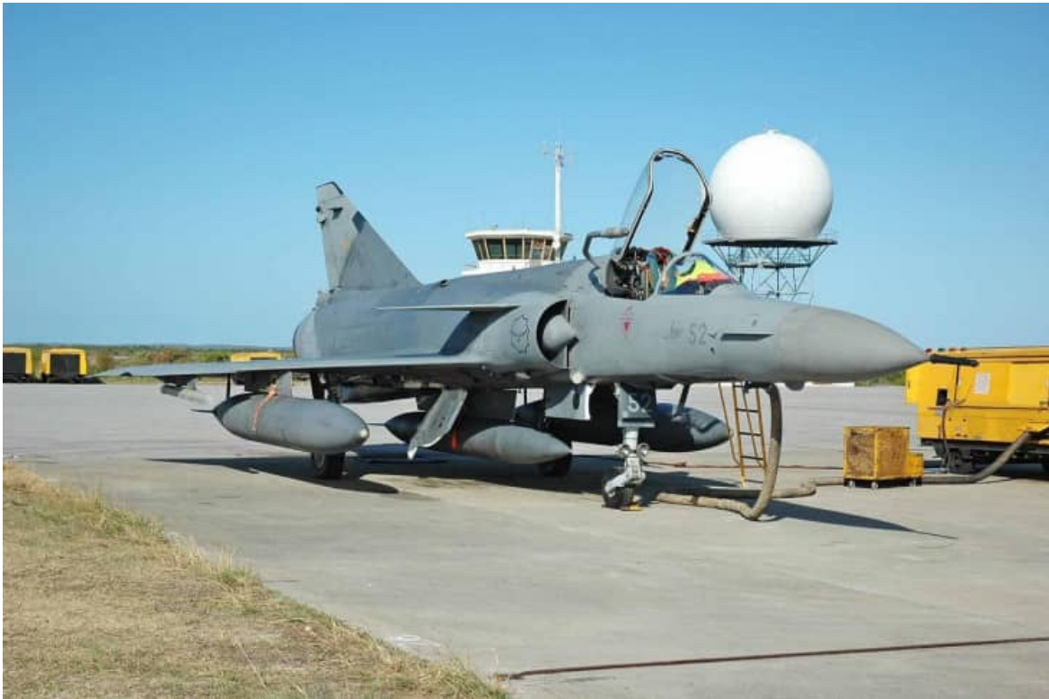
Image C-3 – Cheetah C #352 with an RP825(2) 825 liter tank on the centerline and two 1302 1,300 liter tanks beneath the wings. The pylon for the 1302 tanks was designated CRP-186.
