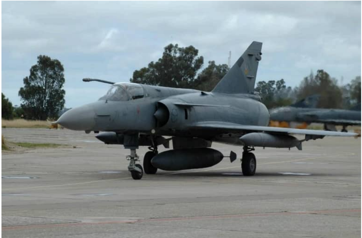
Image C-6 – Cheetah C #371 carrying an RP62 1,300 liter tank on the centerline and two RPK combined fuel tank / bomb carriers beneath the wings.
