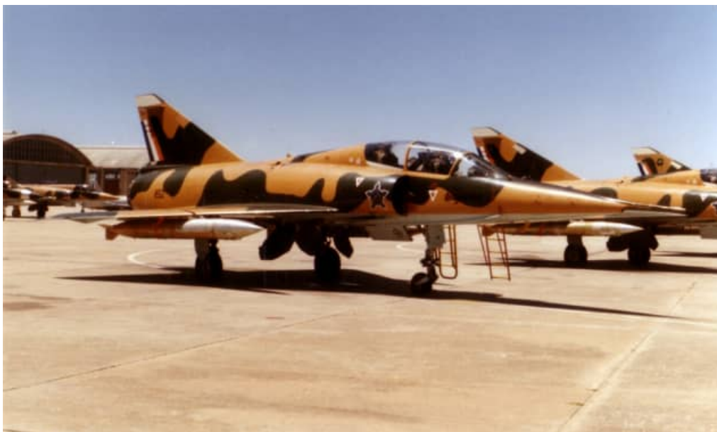
Image D2Z-2 – These Mirage IIID2Zs are carrying two of the Israeli designed finned AZ 500 liter fuel tanks.
