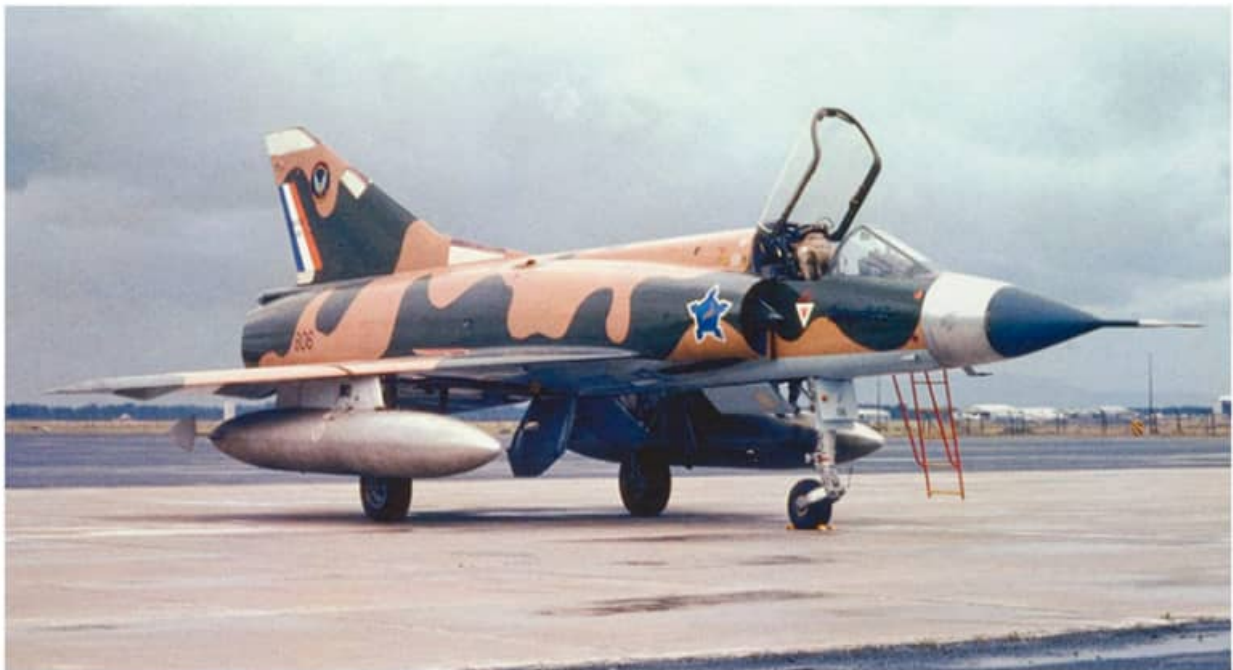
Image CZ-9 (above) – Mirage IIICZ #806 is carrying two French designed RP62 1,300 liter subsonic fuel tanks on CRP37 pylons. Note the nose down angle of the tanks relative to the aircraft. These tanks were equipped with horizontal fins and vertical end plates.
