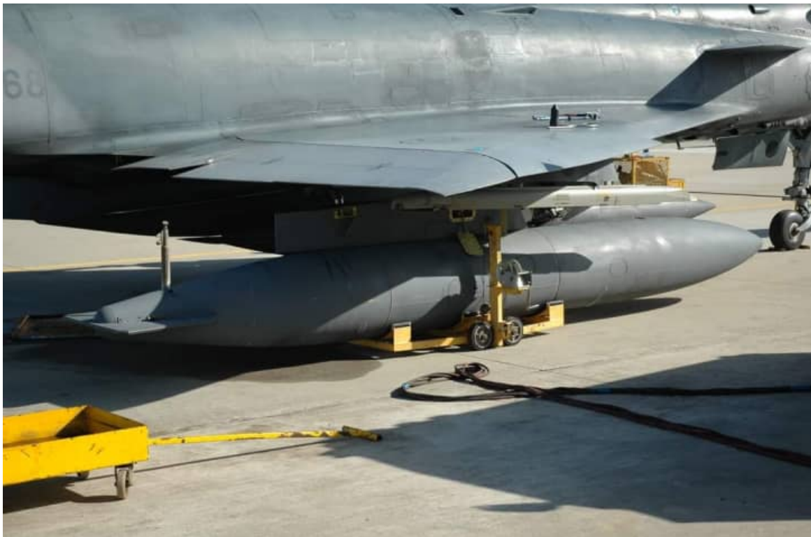
Image C-4 – Cheetah C #368 with a 1302 1,300 liter tank prior to mounting onto the inboard wing station. This tank is different to the RP62 in that it is more slender in shape and does not have the end plates on the horizontal fins. The reinforcing post which supports the rear of the tank is visible in this image and is unique to this tank as used by the SAAF. This is an Israeli origin as designed for the Kfir series of aircraft.
