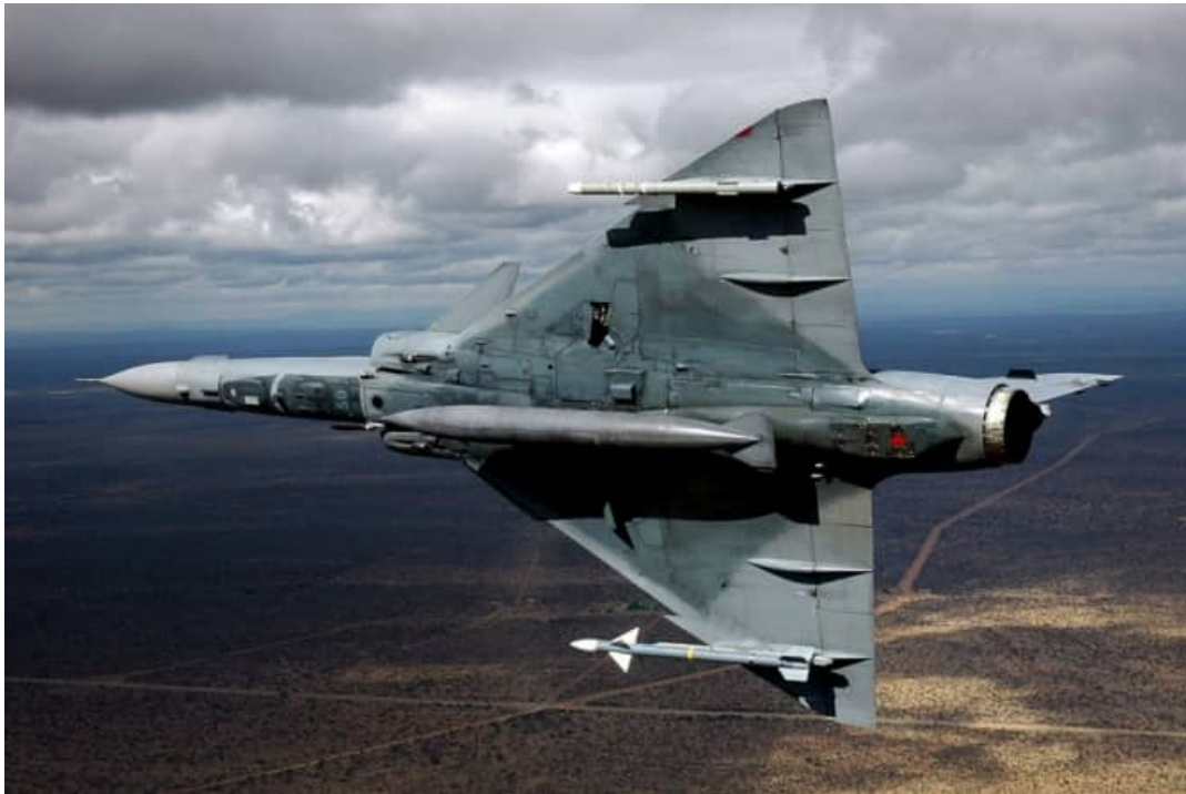
Image C-1 and C-2 – Cheetah Cs (#359 above and #347 below) carrying an RP825(2) 825 liter tank on the centerline station. The pylon for this tank was designated CRP-312. The missiles in the image above are the V4 Derby and in the image below are the V3S Python.
