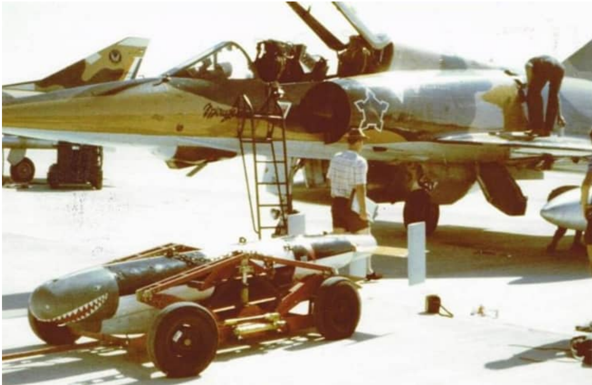
Image DZ-3 (above) – This Mirage IIIDZ is carrying two RP62 1,300 liter subsonic fuel tanks on the wing pylons. The object on the ground is a test article for the H2 glide bomb.
