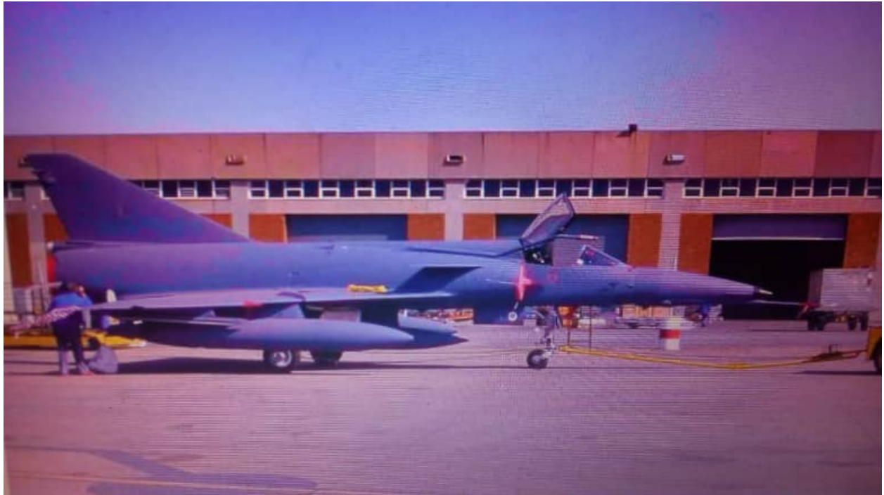
Image E-6 – Cheetah E carrying a centerline RP825(1) 880 liter fuel tank on the centerline station and two RP62 tanks 1,300 liter tanks (note end plates on the fins at the rear of the tank) beneath the wings.
