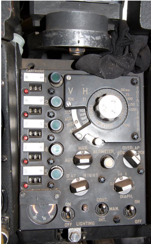
Camera control panel at the center of the instrument panel
