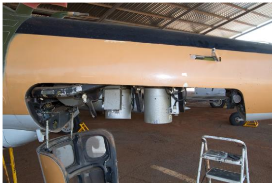
600mm focal length cameras in RZ #838s nose.
