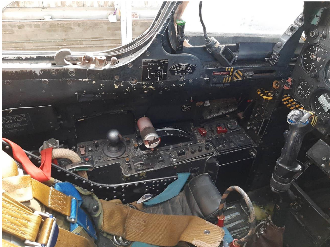
Left side of cockpit showing the throttle lever and the camera selector knob. Note the camera selector chart above the throttle lever.
