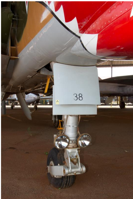
Nose wheel on RZ #838. The right hand landing light and the two front opening doors with their linkages can be seen. The main nose gear door is in the closed position. The steering mechanism is located above the nose wheel.
