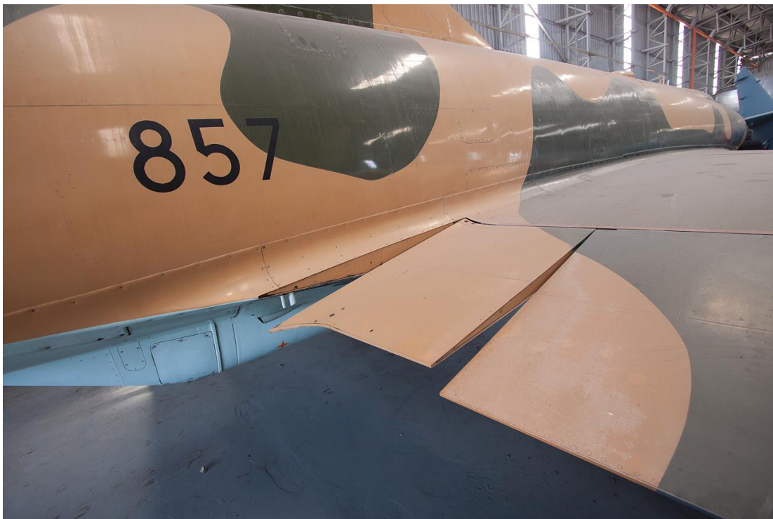
Position of the inboard pitch control surface relative to the elevon. There were two elevons on each wing which operated in unison. As was typical for all Mirage III variants, all control surfaces on the wing drooped with hydraulic power off.
