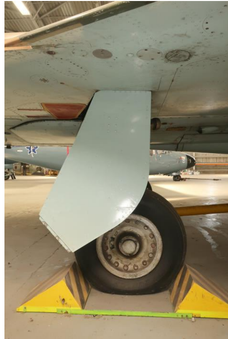
Port (left) landing gear leg and cover.
