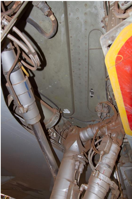
Left side main undercarriage leg details. The wheel brakes and leg forward stabilization arm are as for the EZ but different to the BZ/CZ as explained in Part 4.
