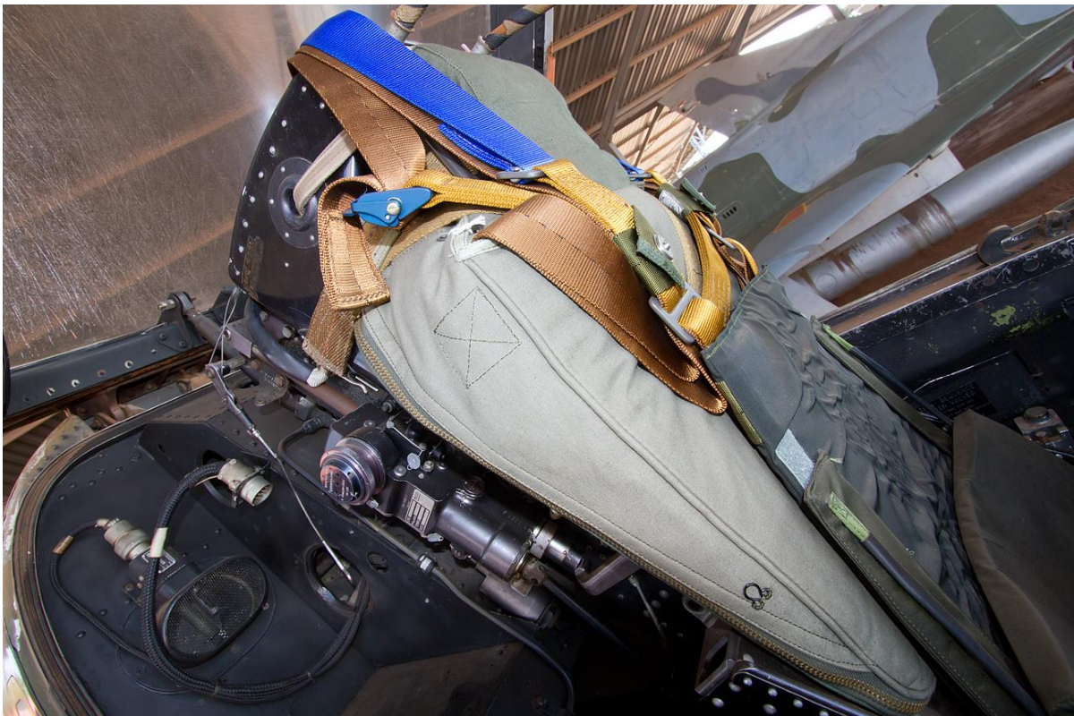
Upper right side of Martin Baker MB.MK.4 ejection seat and rear bulkhead.
