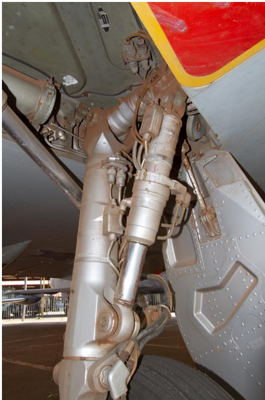
Left side main undercarriage leg details. The wheel brakes and leg forward stabilization arm are as for the EZ but different to the BZ/CZ as explained in Part 4.
