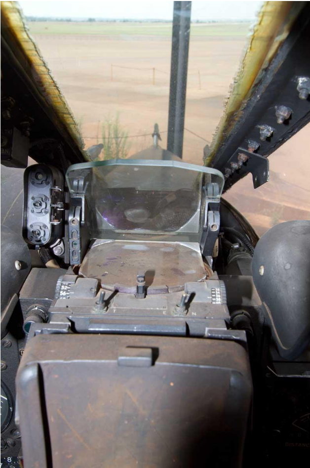
Gyro gun sight assembly and Head Up Display (HUD) details – the oblique mounted glass is the Combining Glass or HUD reflector and the round glass is part of the projector.
