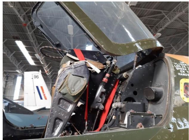
Martin Baker Mk.IV ejection seat.
