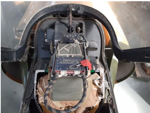
Martin Baker Mk.IV ejection seat.
