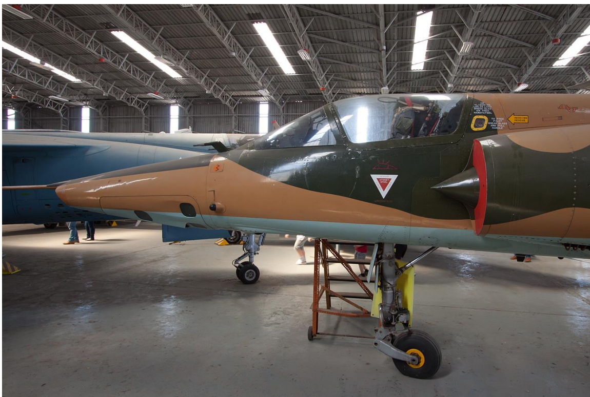
Ejection seat warning triangle, displayed both sides of the fuselage. Note yellow surround to the emergency canopy release window aft of cockpit.
