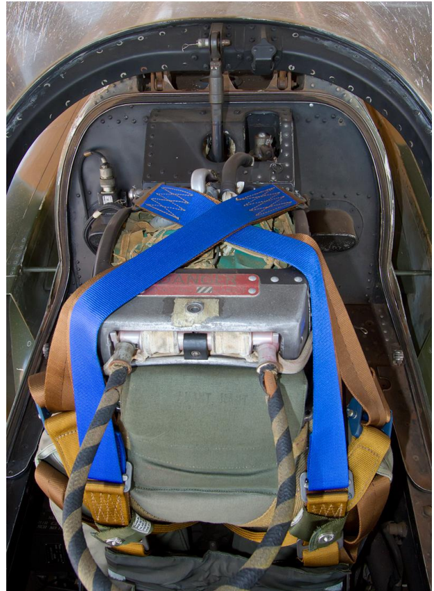
Martin Baker MB.MK.4 ejection seat.
