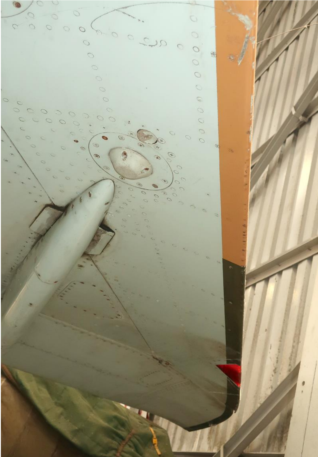
Underside of port wing. Note wrap around of upper surface colours (characteristic of all camouflaged SAAF Mirages). The wing curves towards the tip. The ejection seat is covered with an aerodynamic fairing. This would be removed and replaced with a weapon pylon when the air-to-air missiles were fitted.
