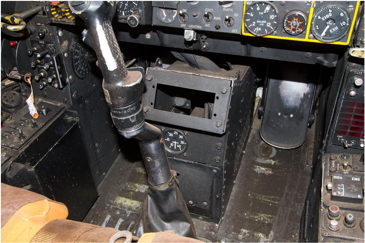
The small dial just ahead of the control column is the cabin altimeter.
