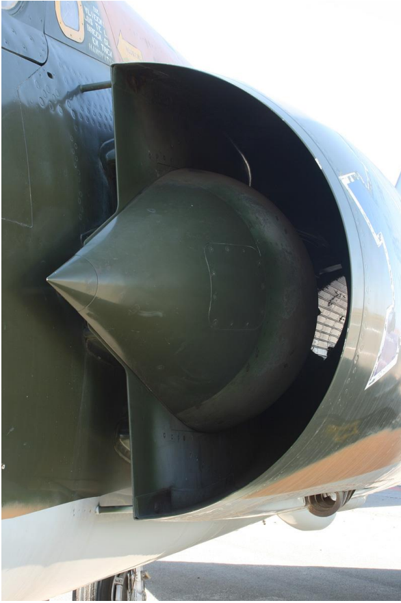
Intake detail on RZ #838. This would be typical for the DZ, D2Z, EZ and RZ. The R2Z has a more prominent scalloped intake splitter plate – see next page. Note the two support rods between the intake and the fuselage. This is different to the BZ and CZ which had a plate strengthening plate (refer to Part 4).
