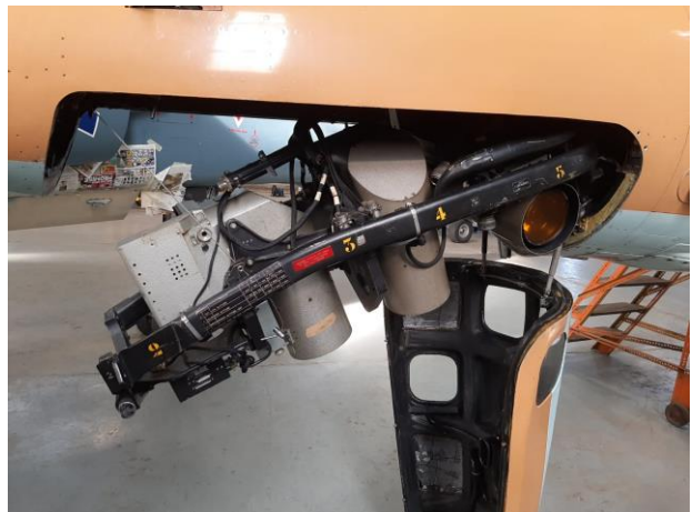
The box shaped object in the image below appears to be the forward facing camera.
