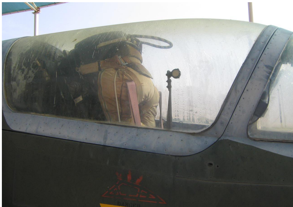
Camera sighting aid which is raised by the pilot and used to align the side looking cameras to the target. There is one each side of the cockpit.
