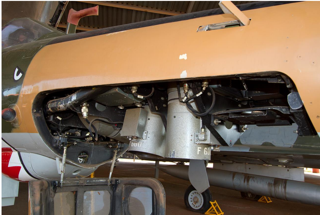
The camera bay window release latch is in the open position. The cameras were mounted on a frame which could drop down supported by cables for access to the camera.
