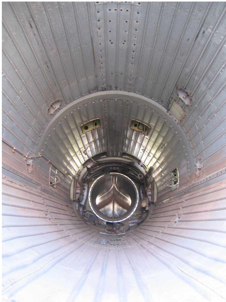
Engine bay looking forward towards the bifurcated intake trunking.
