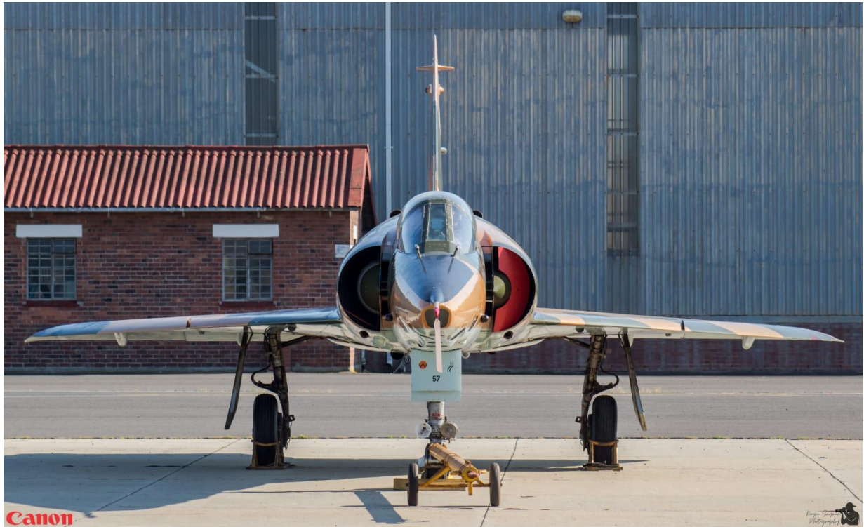
Head-on images of R2Z #857 (above) and RZ #818 (below). Note the distinct angles of the main landing gear legs. Wing anhedral is apparent as is the curvature of the leading edges.
