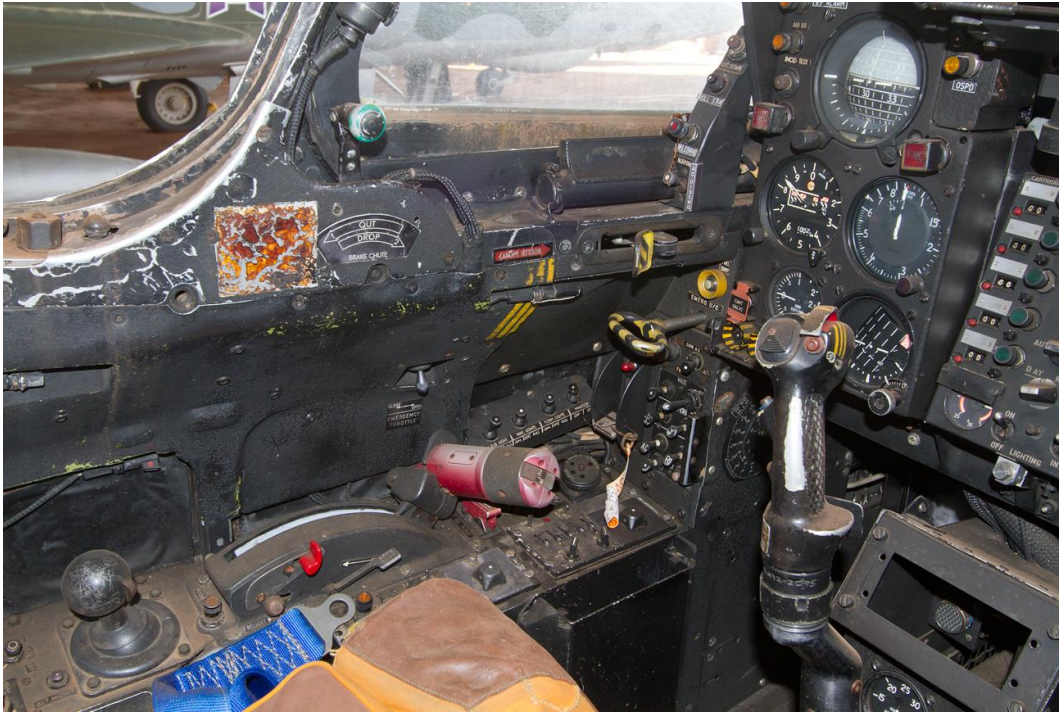
Left side of the cockpit. The red cylindrical object is the throttle lever. The round black control knob at bottom left is the camera selector knob.
