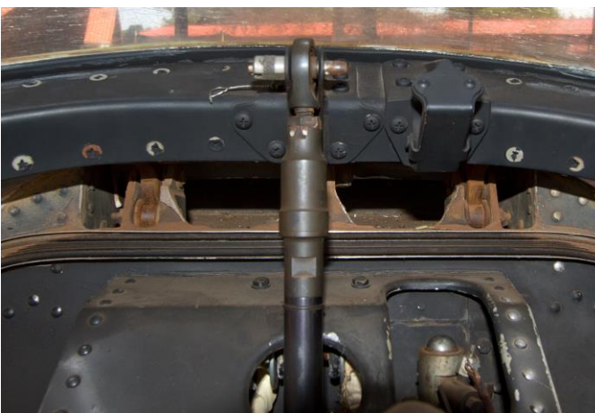
Canopy actuator piston at cockpit rear bulkhead.
