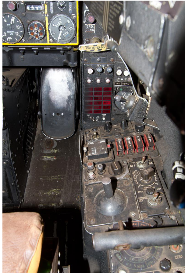
The panel with red rectangles is the systems warning panel. The four red switches are for the stores selector switches.
