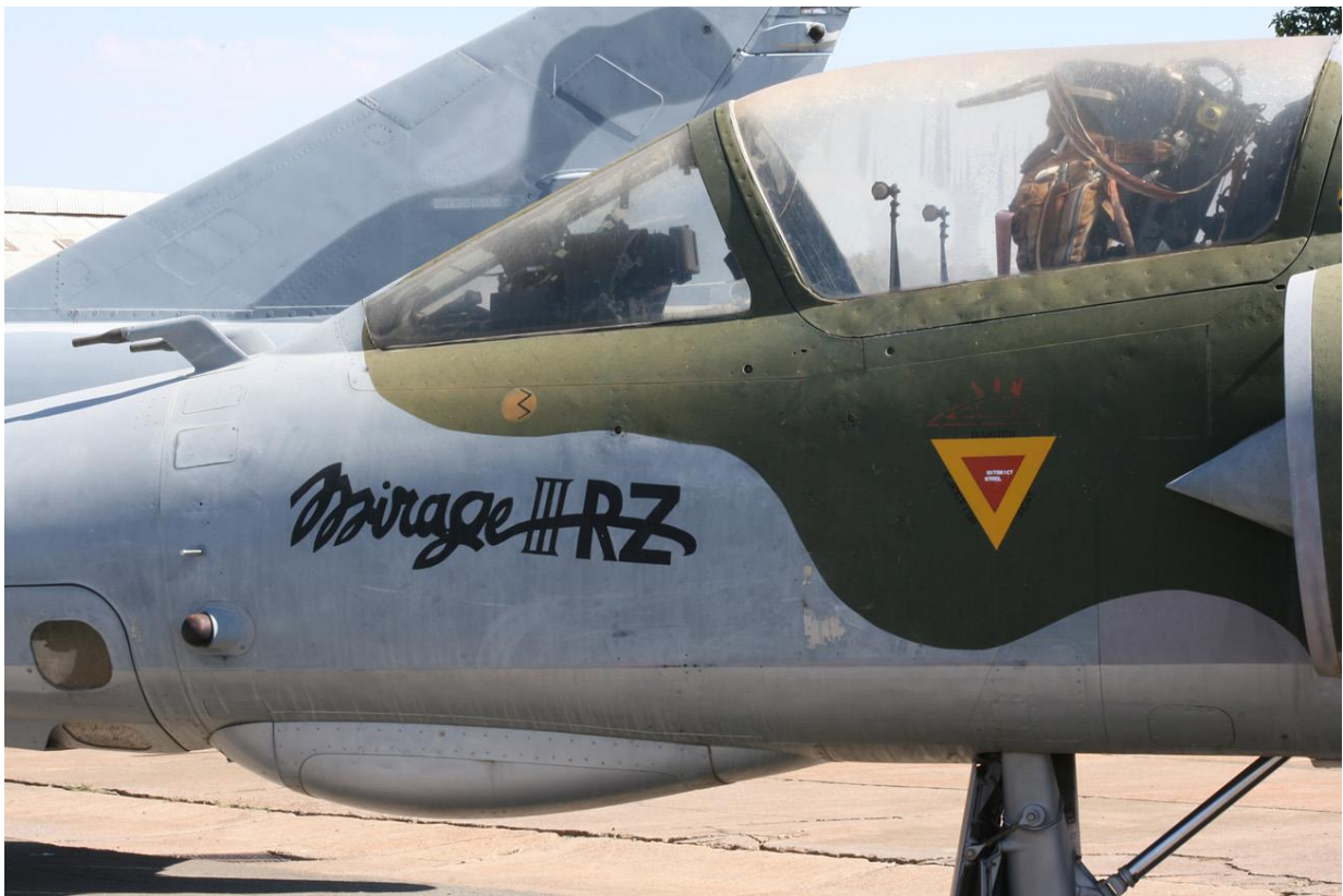
Doppler antenna. Above this is the black CRWS antenna and the small straight incidence probe above that. The ejection seat triangle is not the same as for other SAAF Mirage III variants. This is how the RZs were delivered.
