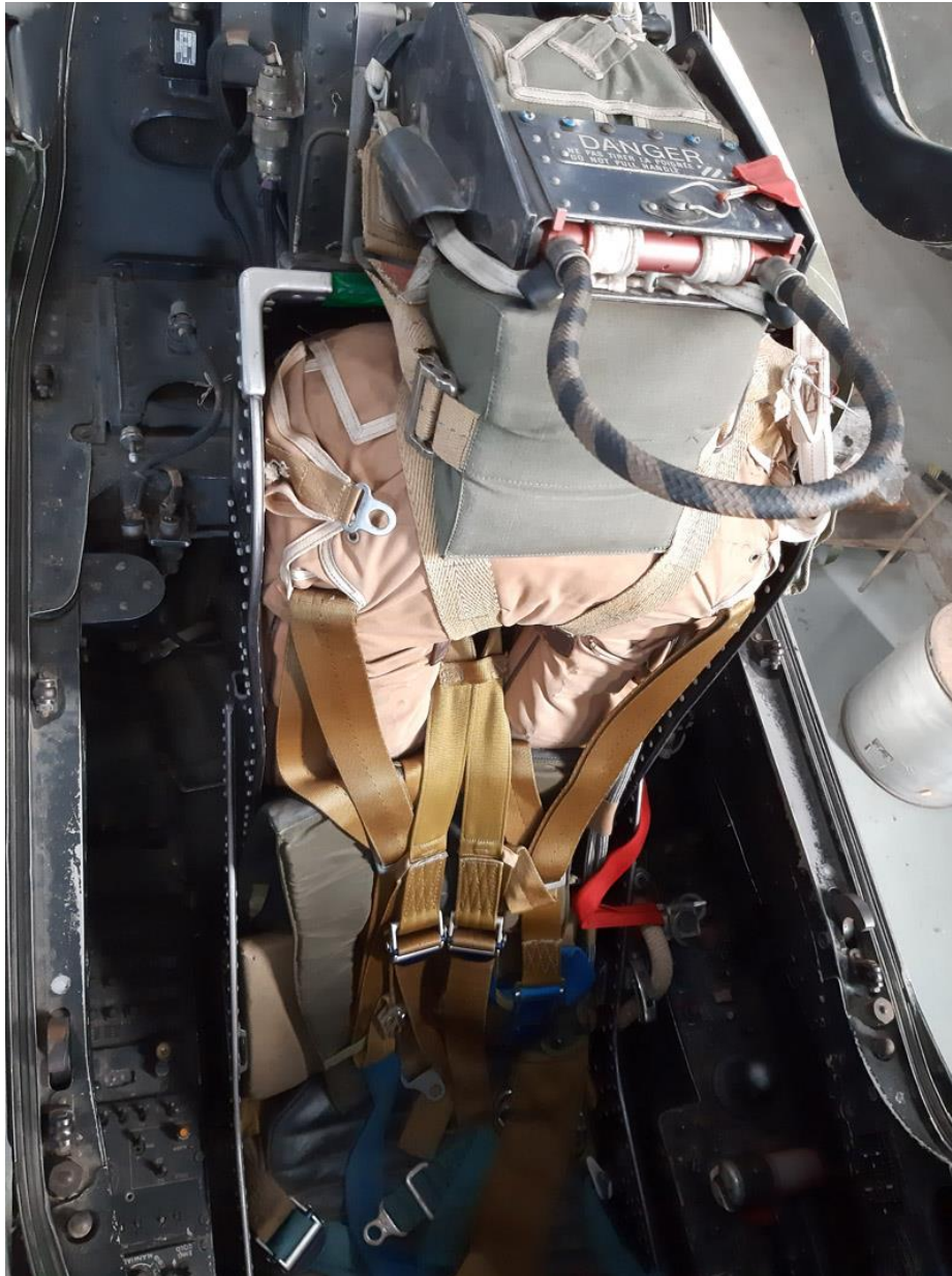
Martin Baker Mk.IV ejection seat.
