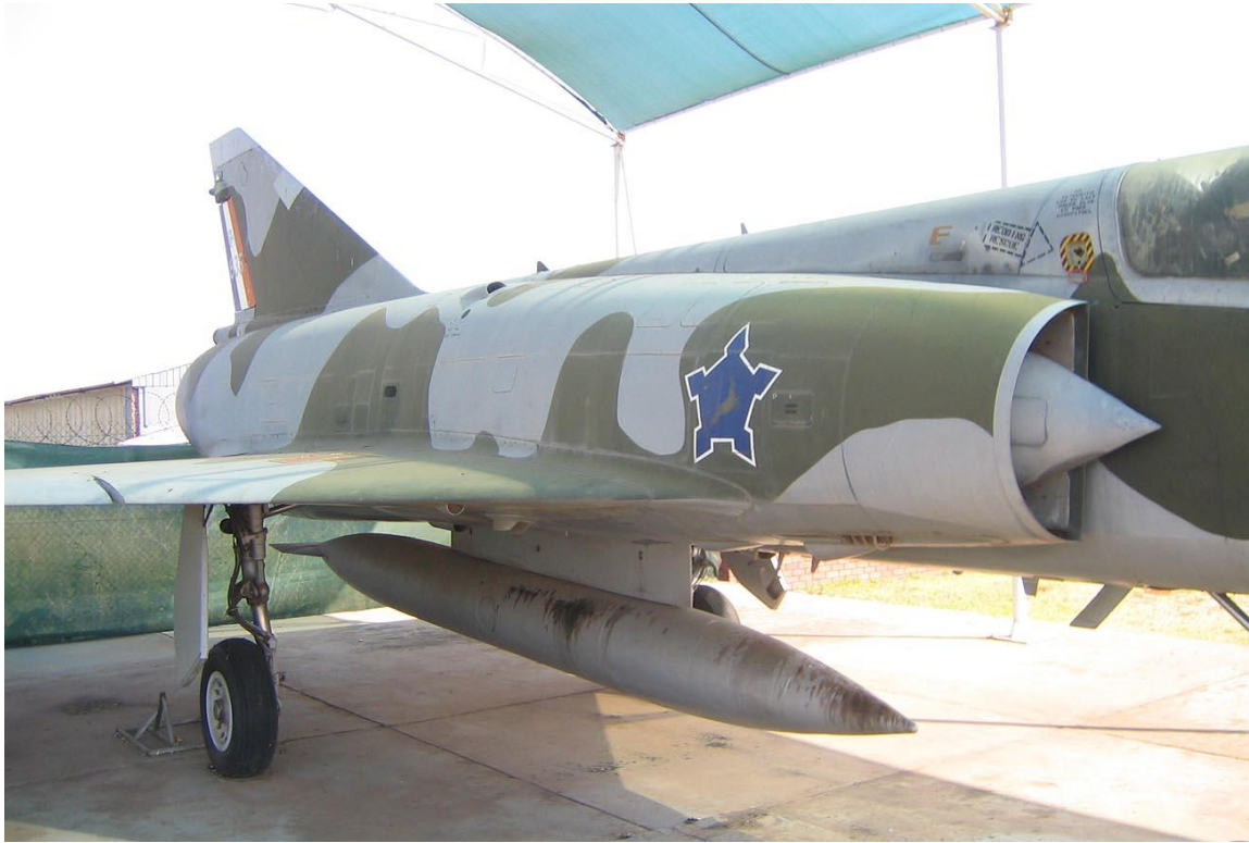
Details to note – centerline RP825 fuel tank, grey outer leading edge to intakes, but green on inside. Late antennae configuration.
