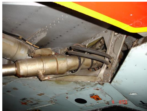
Retraction piston on right wing of R2Z #857.
