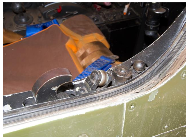
Canopy locking mechanism on right side of cockpit.
