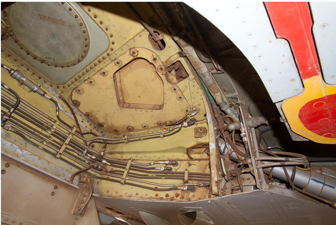
The silver piston in the image below is the undercarriage leg retraction piston.
