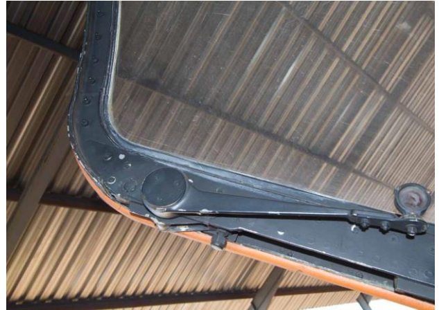
Right side of canopy with manual camera aiming sight in stowed position.
