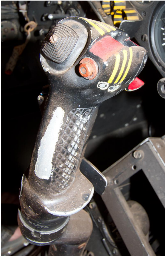
Control column. The square object to the left is the roll and pitch trim switch, the round red button is the camera start button, the red square is the trigger. The yellow stripes are the spin recovery marks.
