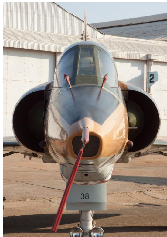
Nose wheel on RZ #838. The right hand landing light and the two front opening doors with their linkages can be seen. The main nose gear door is in the closed position. The steering mechanism is located above the nose wheel.
