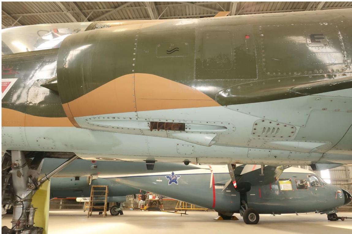
The rust coloured assembly is the muzzle brake for the port 30mm cannon.
