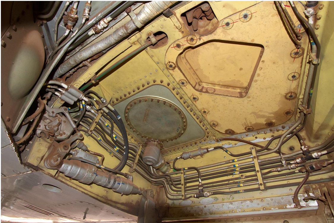
Details of the main wheel well including hydraulic hoses and electrical wiring and connectors. The silver piston to the bottom left in the image above is for the undercarriage door retraction arm. The rust coloured mechanism at the top center of the image is the undercarriage retraction lock. This locks onto a lug located on the lower undercarriage leg.
