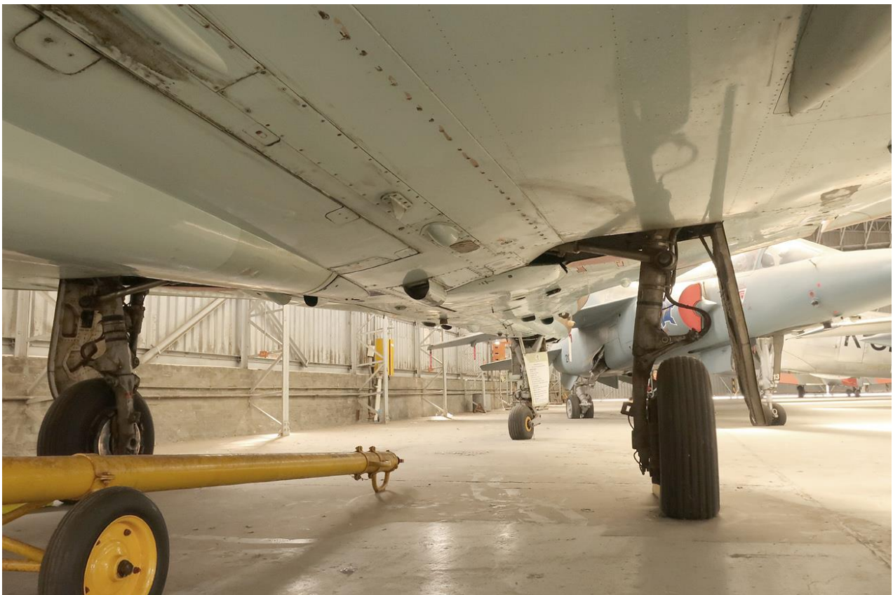
Note the various intake and vents and standard NATO aircraft servicing symbols on the underside of R2Z #857.
