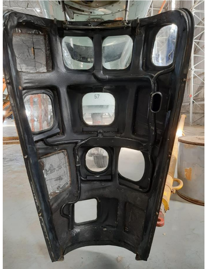
Ducting for heating air to keep windows clear is apparent in the image above.
