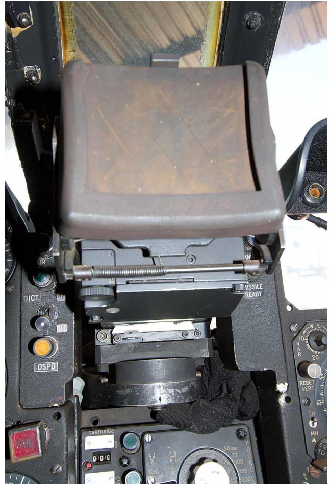
Gyro gun sight. The square box is the gun camera.
