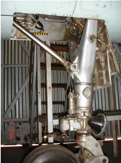
Nose landing gear. Interior of gear bay is silver. Landing light body is painted black.
