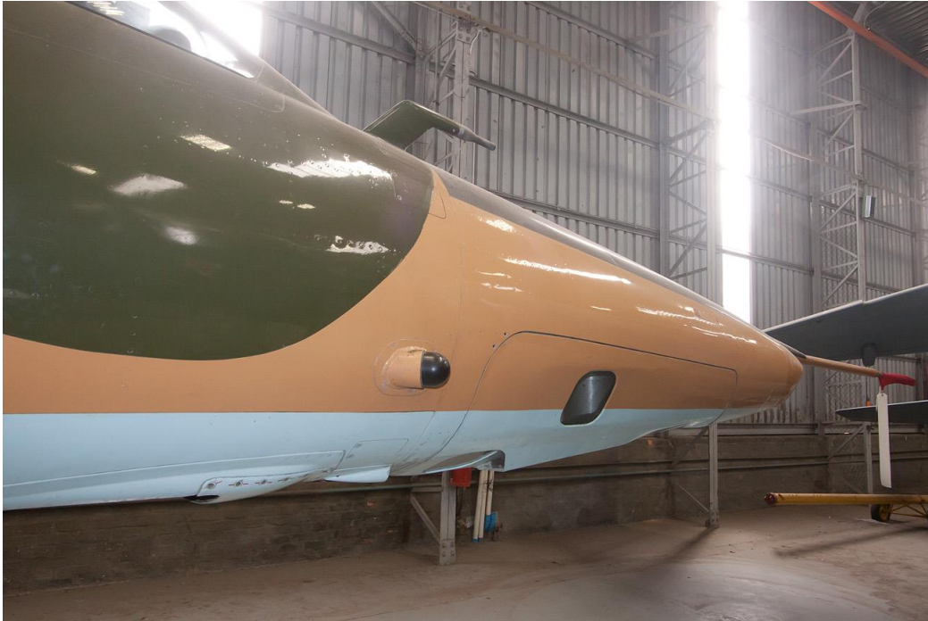
Sleek nose of the R2Z – the black round object is one of the CRWS forward looking “cat balls” antennae.
