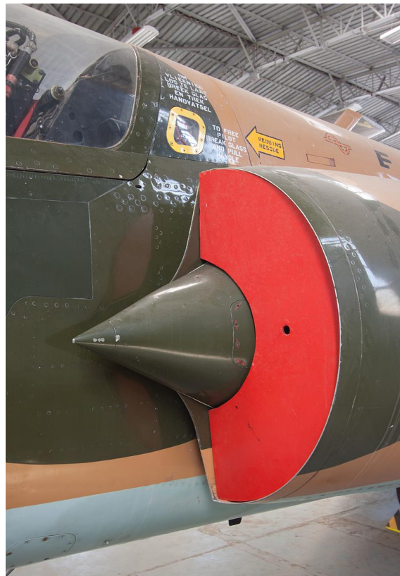
Scalloped intake splitter plate indicative of an Atar 09K50 powered Mirage.
