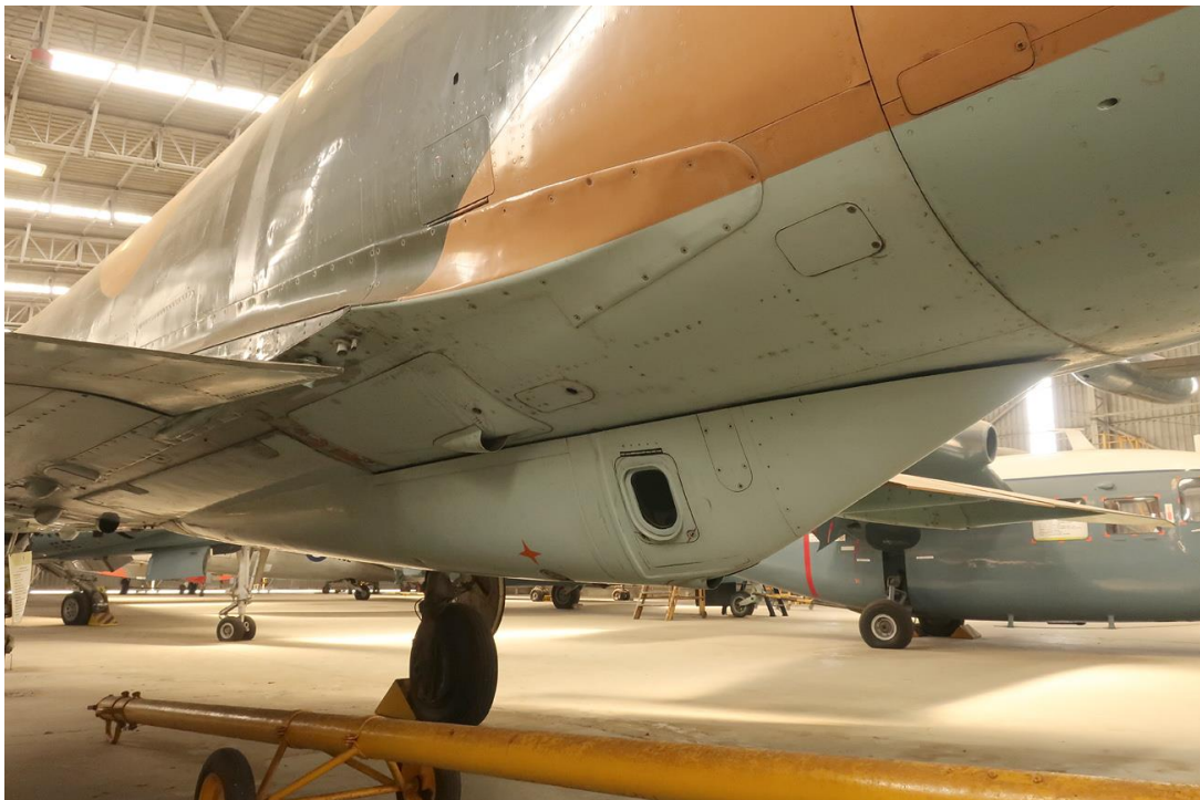
Rear ventral fuel tank with inspection window. Several small fuel dump / overflow pipes are located at the junction of the wing trailing edge to the fuselage.
