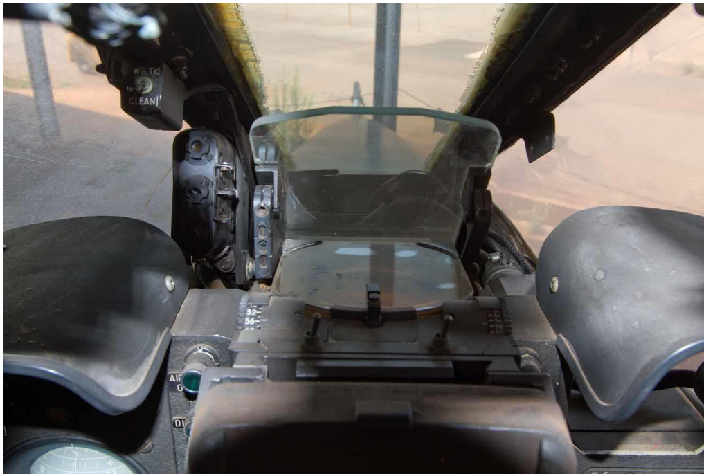
Gyro gun sight assembly and Head Up Display (HUD) details – the oblique mounted glass is the Combining Glass or HUD reflector and the round glass is part of the projector.
