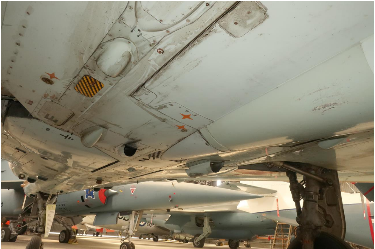
Note the various intake and vents and standard NATO aircraft servicing symbols on the underside of R2Z #857.
