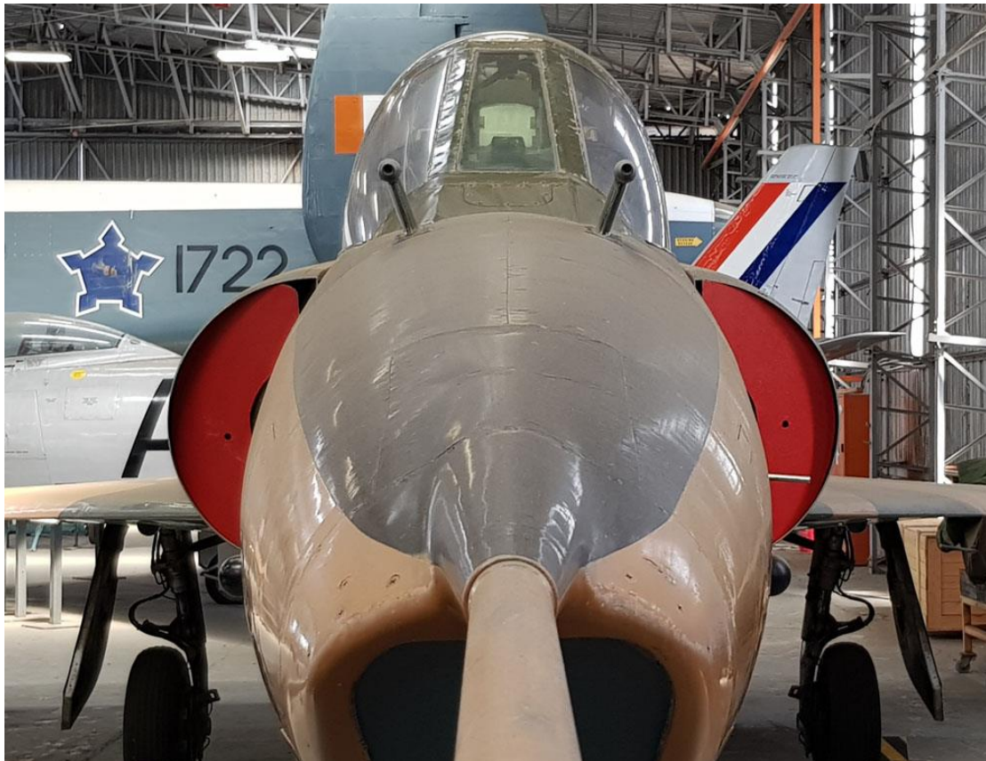
Note dual pitot probes ahead of windshield. The small rod sticking out to the right in the photo is the angle of attack or incidence probe.
