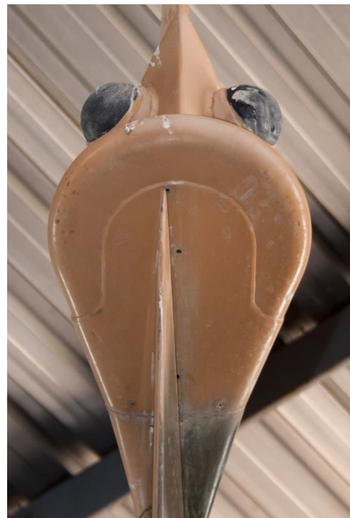
CRWS (black antennae) and original pancake shaped radar warning receiver (RWR).
