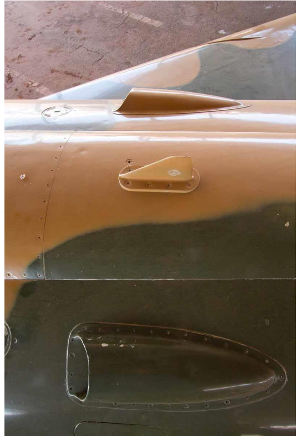
Upper fuselage detail. The blade antenna is for TACAN. The engine bay cooling intakes are symmetrical. The slot on the leading edge of the wing can be seen at the top right of the image. The round objects are the fuel tank filler caps (symmetrically located either side of the fuselage)
