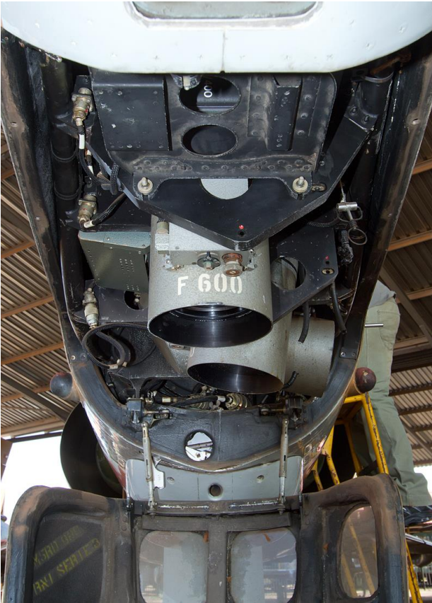
600mm focal length cameras in RZ #838s nose.
