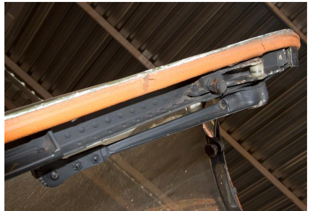
Manual aiming sight in stowed position.
