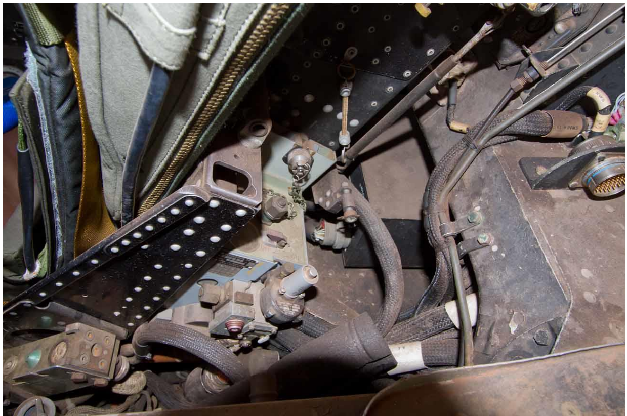
Upper left hand rear bulkhead and ejection seat.
