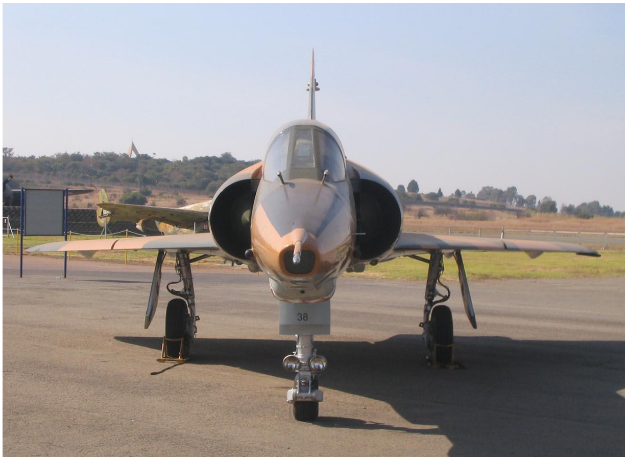
Head-on images of R2Z #857 (above) and RZ #818 (below). Note the distinct angles of the main landing gear legs. Wing anhedral is apparent as is the curvature of the leading edges.
