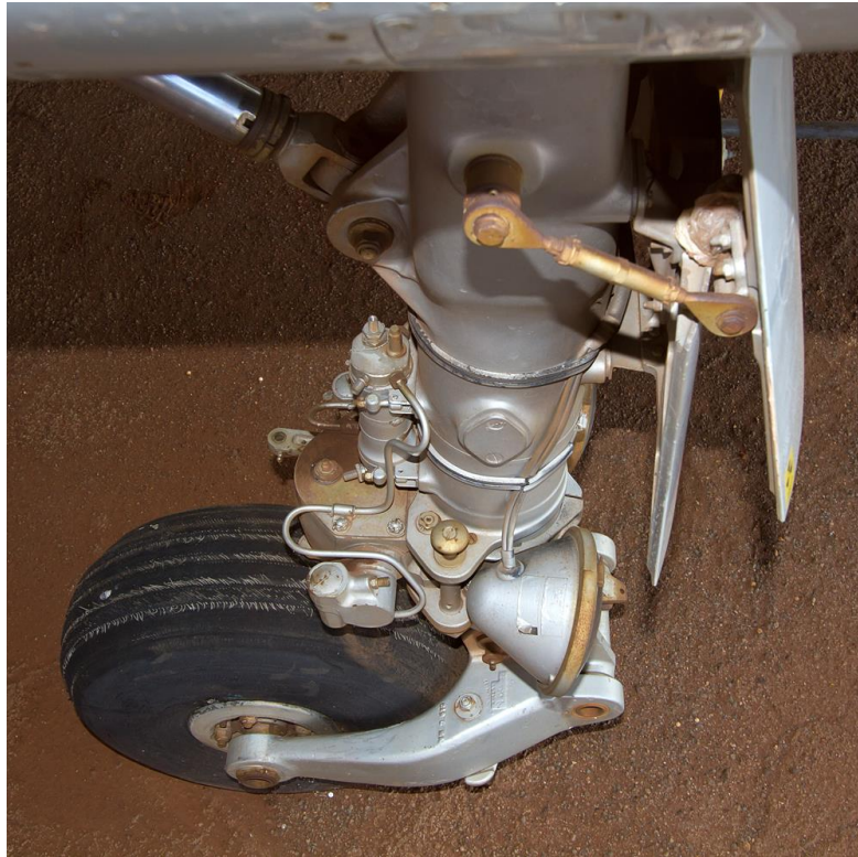
Nose wheel on RZ #838. The right hand landing light and the two front opening doors with their linkages can be seen. The main nose gear door is in the closed position. The steering mechanism is located above the nose wheel.
