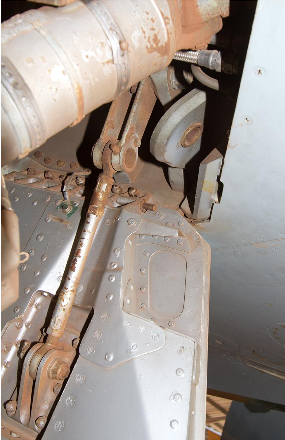
Detail view of outboard portion of landing gear on the left wing. The cylindrical object at top left is the leg stabilization arm. The empty lug for the C and B undercarriage stabilizing arm can clearly be seen (as described in Part 4).
