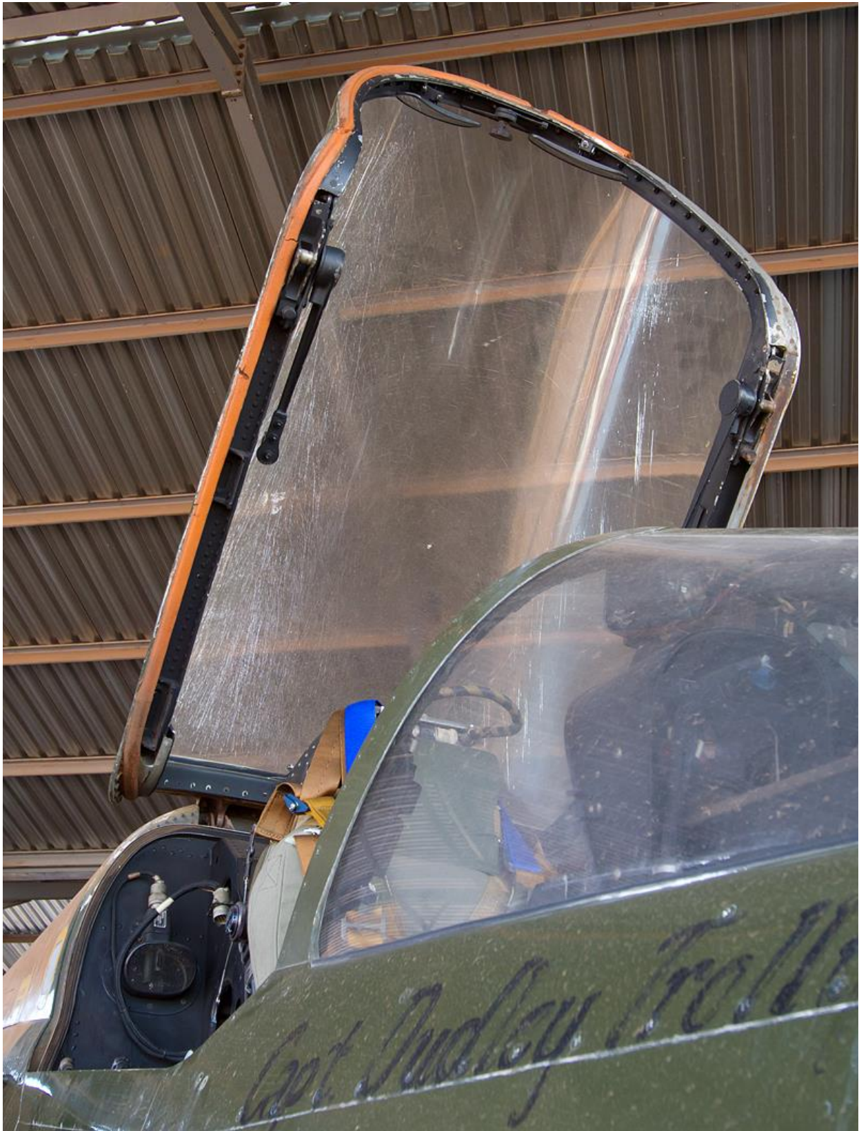
The two long black objects on either side of the canopy are the camera polaroid sights which are raised by the pilot and used to align the side looking cameras to the target.
