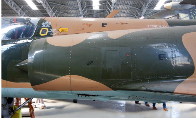
Examples of standard NATO aircraft servicing stenciling – similar for all SAAF Mirage III variants.
