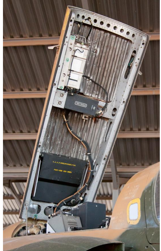
Avionics hatch aft of cockpit – RZ #838
