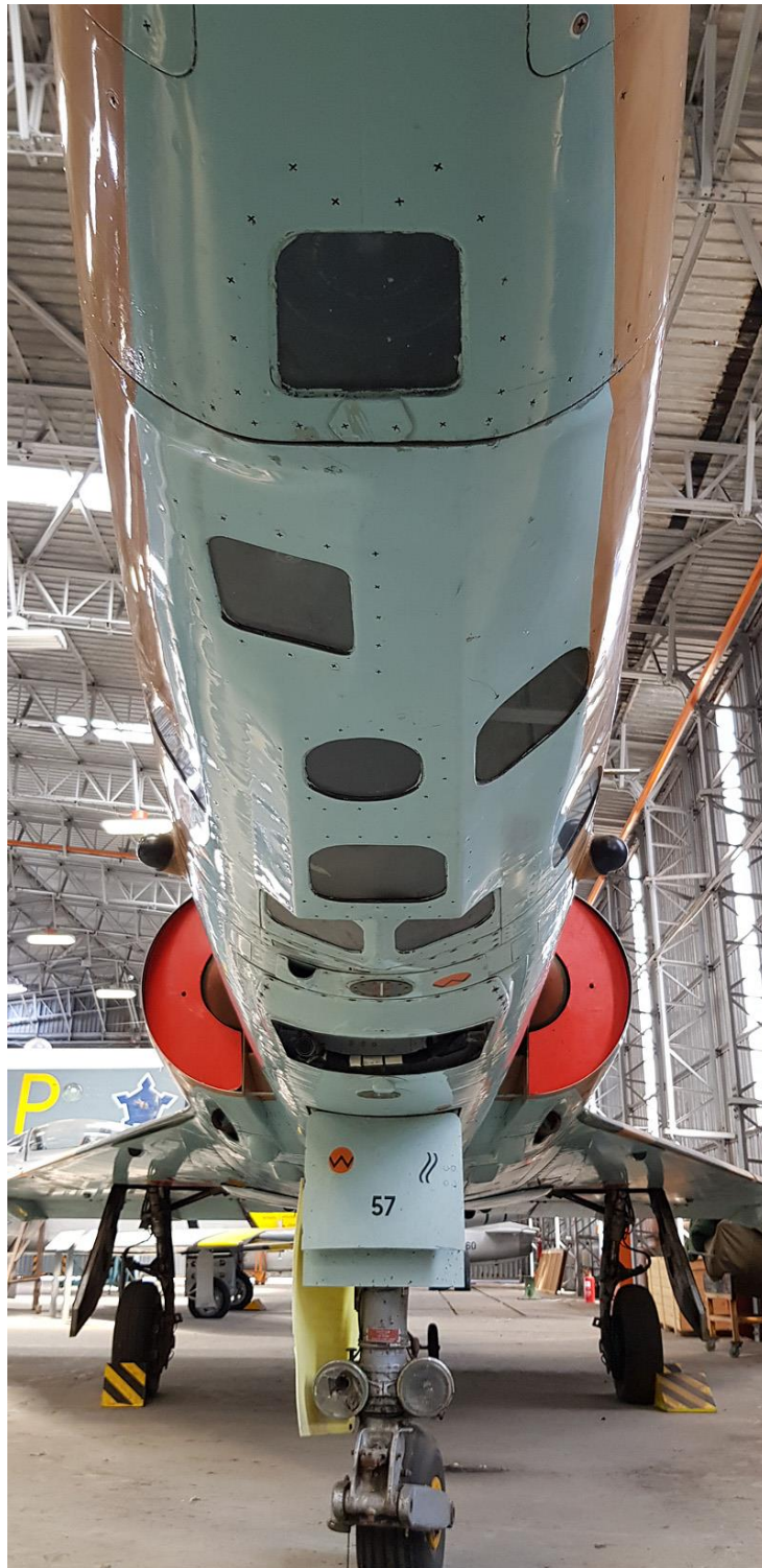
Dual landing lights characteristic of all SAAF Mirage III variants with the exception of the BZ and CZ
