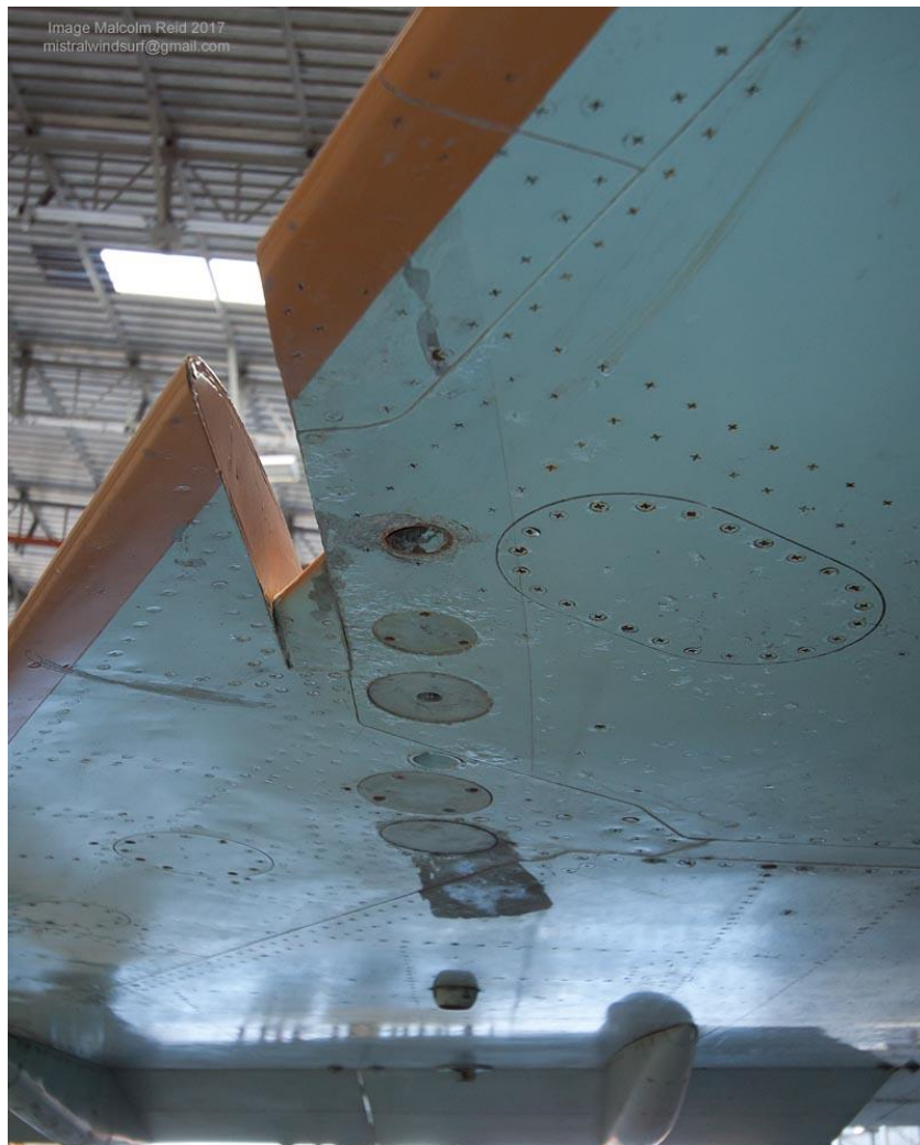
Starboard lower wing – note wrap around of upper surface camouflage colour – typical of all SAAF Mirage III versions.
