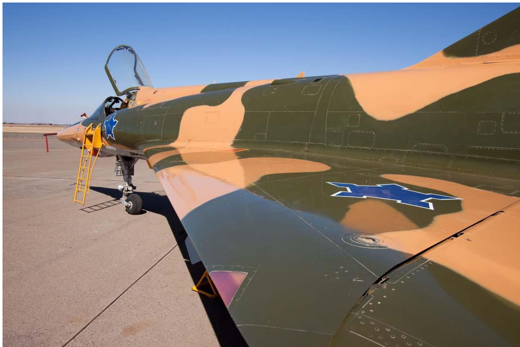
Intake detail on RZ #838. This would be typical for the DZ, D2Z, EZ and RZ. The R2Z has a more prominent scalloped intake splitter plate – see next page. Note the two support rods between the intake and the fuselage. This is different to the BZ and CZ which had a plate strengthening plate (refer to Part 4).
