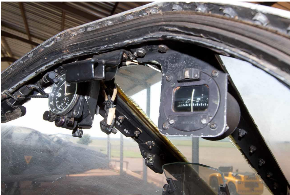
Clock (upper left) and standby compass mounted to windshield frame.
