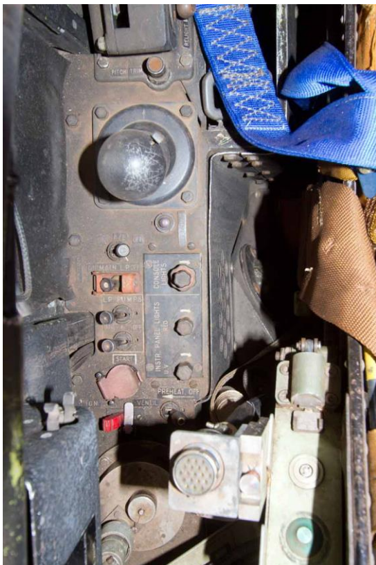
Camera selector on the left cockpit sill. Pushing the knob forward, left or back would select, respectively, the forward, left or vertical camera (no right hand camera).
