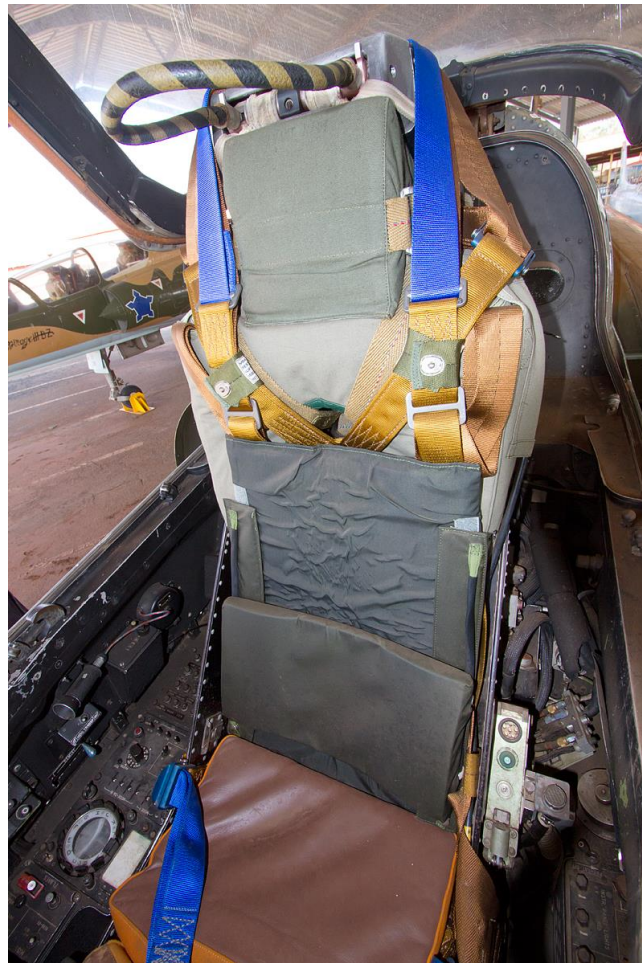
Instrument panel and Martin Baker Mk. 4 ejection seat details as seen at the SAAF Museum Swartkop Air Base in 2016.
