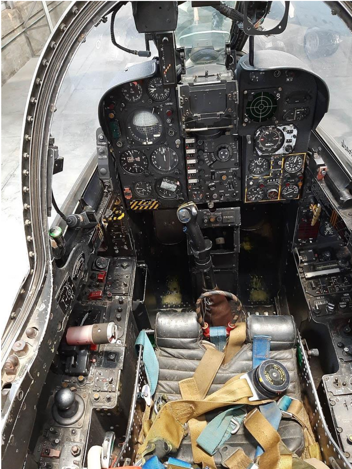
Cockpit of R2Z #857. The gun camera beneath the HUD glass appears to have been removed. The large dial immediately beneath this is the camera focal length control panel. The central panel contains camera controls.
