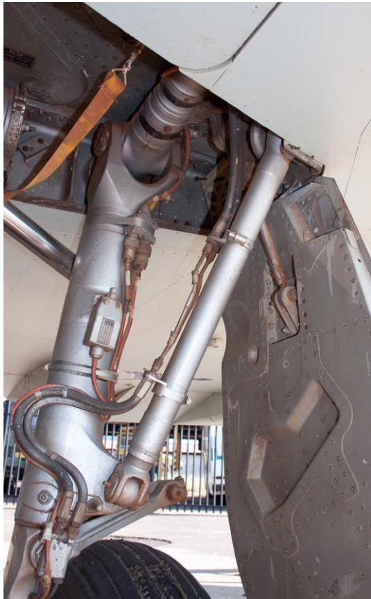
Left hand main landing gear leg detail. The diagonal stabilizing arm configuration is different to that used on the DZ, D2Z, EZ, RZ and R2Z.
