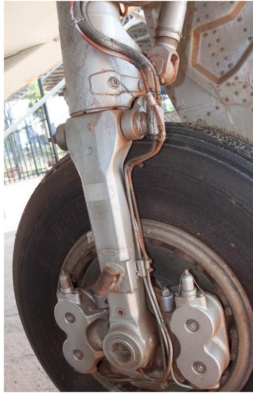
Details of CZ wheel brake assemblies and hydraulic hoses. BZ was similar.
