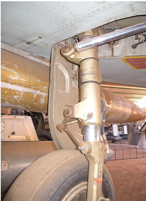
Left main landing gear leg looking forward. Silver rod is retraction piston
