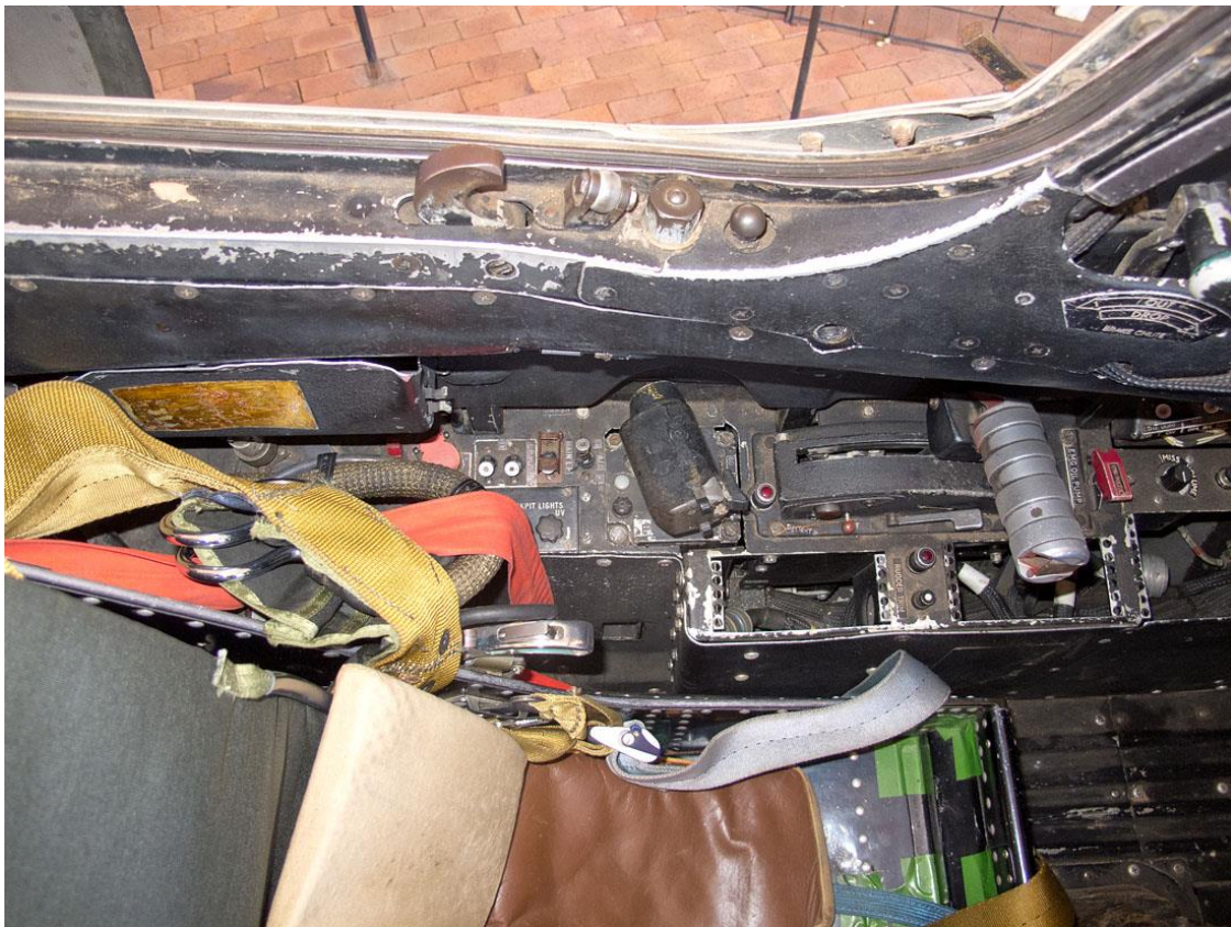
Left side of cockpit. The silver cylindrical object is the throttle lever. The lever aft of this is the radar control stick. The two open rectangular holes would house the primary and secondary UHF radio control units.
