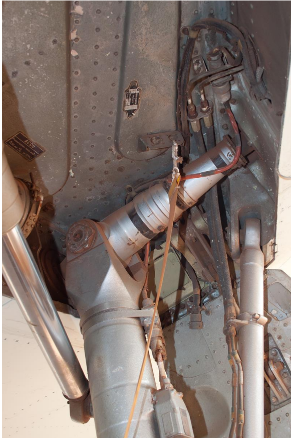
Left hand main landing gear leg detail. The diagonal stabilizing arm configuration is different to that used on the DZ, D2Z, EZ, RZ and R2Z.
