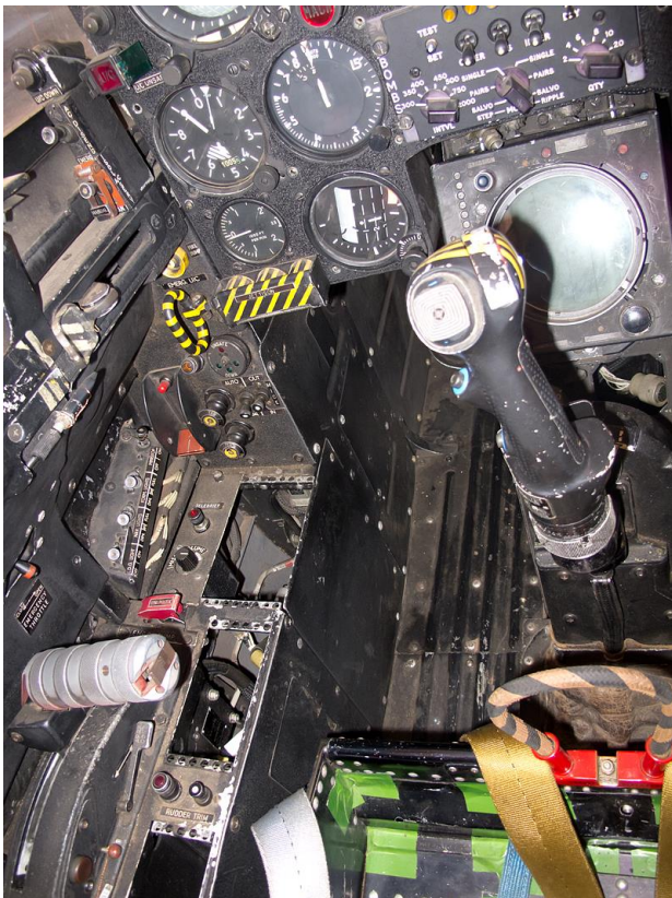
Right hand console which includes from left to right : fuse panel, and other aircraft systems control panels. The black cylindrical object at the bottom of the image is the cockpit light. The weathered handle with the curved slider at bottom right is the canopy open / close lever.
