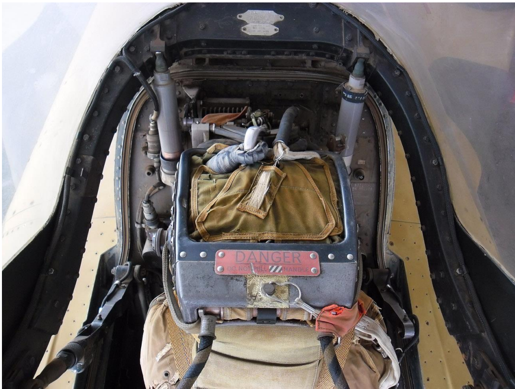
BZ #818 rear cockpit looking aft with canopy open. The top of the ejection seat is visible. The two objects at the top of the image either side of the seat are the canopy opening pistons. Note also at bottom left the additional canopy support arm. The one on the right appears to be missing. This detail is typical for the DZ and D2Z.
