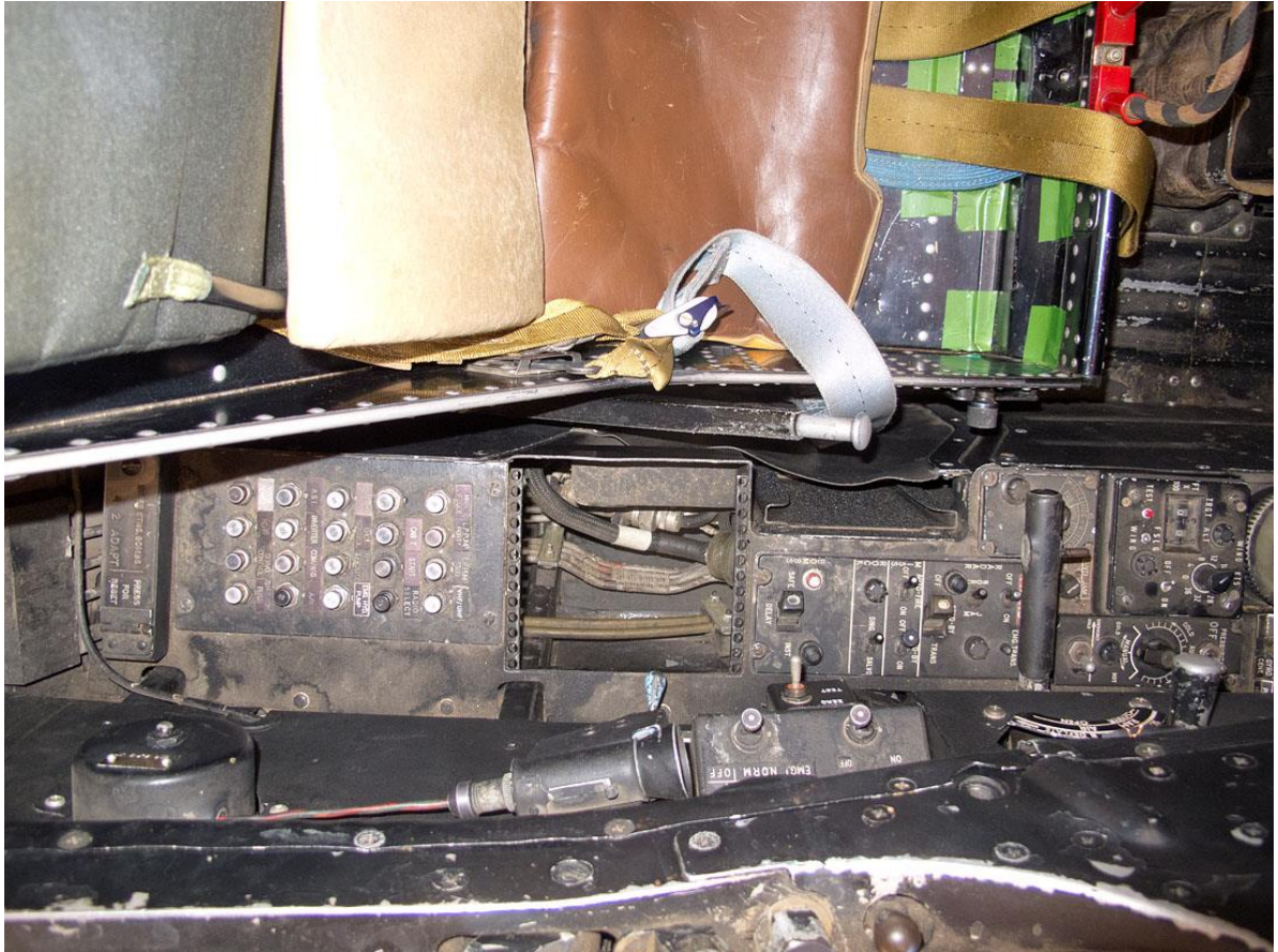
Right hand console which includes from left to right : fuse panel, and other aircraft systems control panels. The black cylindrical object at the bottom of the image is the cockpit light. The weathered handle with the curved slider at bottom right is the canopy open / close lever.
