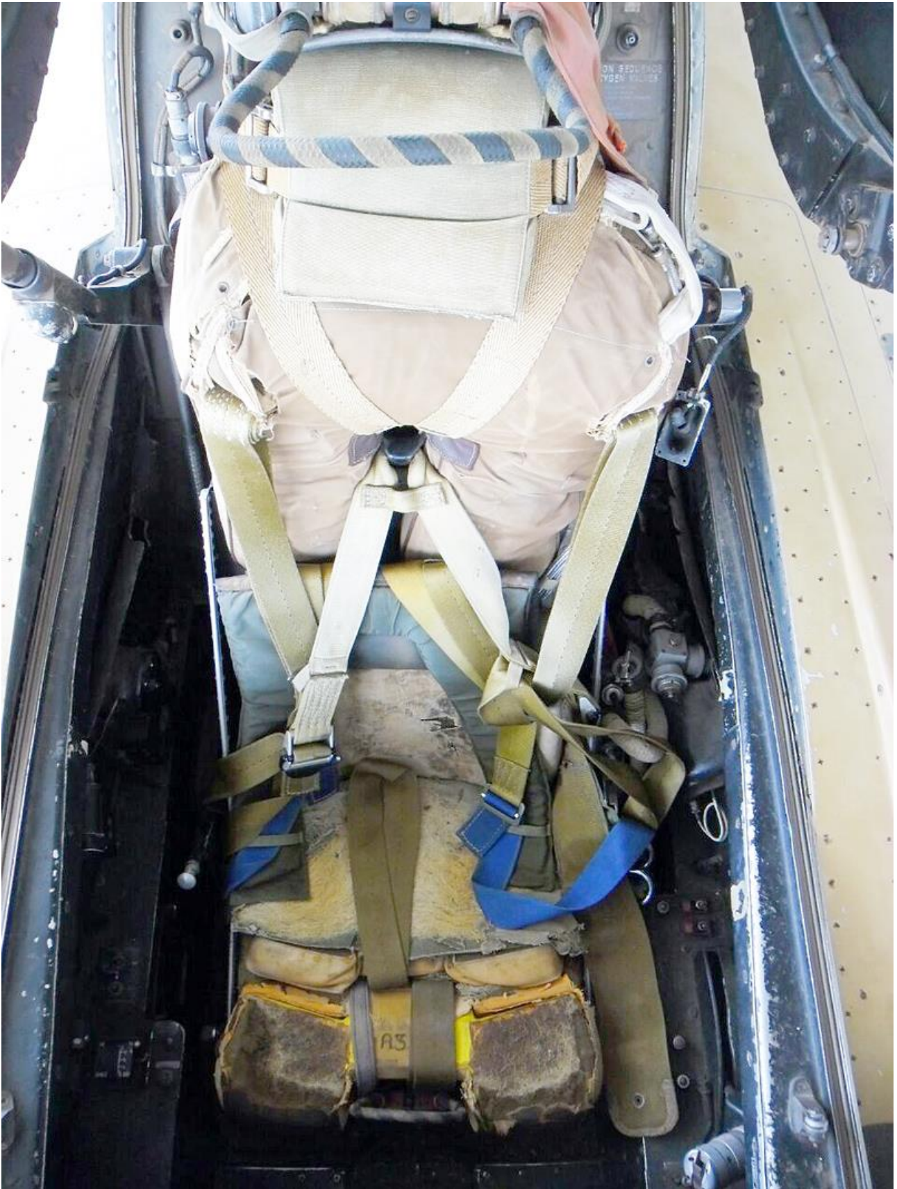
Rear MB.Mk.4 ejection seat in BZ #818.
