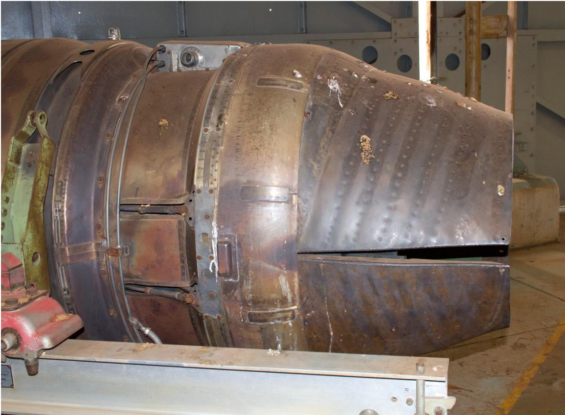
09B on its engine cradle at Swartkop. The clamshell halves are in the closed positions.
