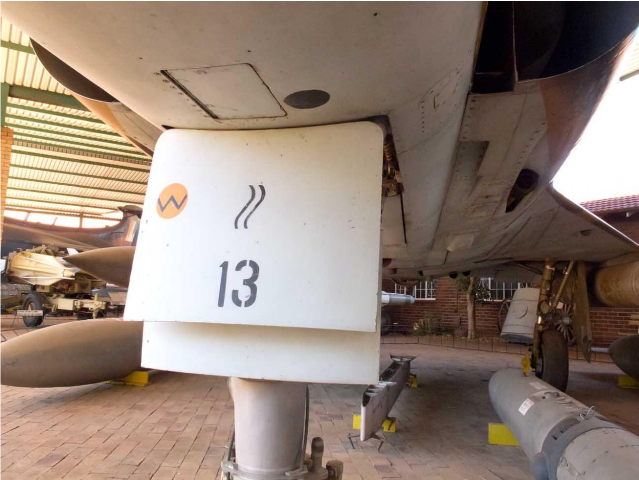
Nose gear covers comprise 3 separate doors. The two above and the lateral opening main door. "13" is typical as to the application of the last two digits of the aircraft number on the nose gear door. All SAAF Mirages were in the "800" series.
