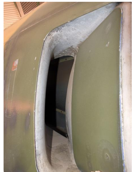
This is the auxiliary engine air door on the starboard intake. This would be opened to allow additional air to the engine at low speeds
