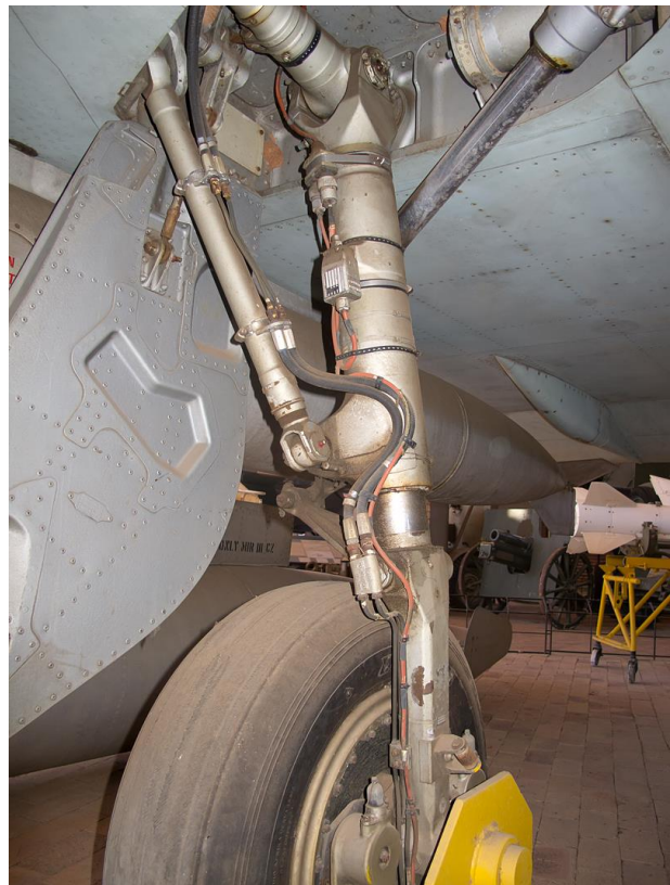
Right main landing gear leg looking aft.
