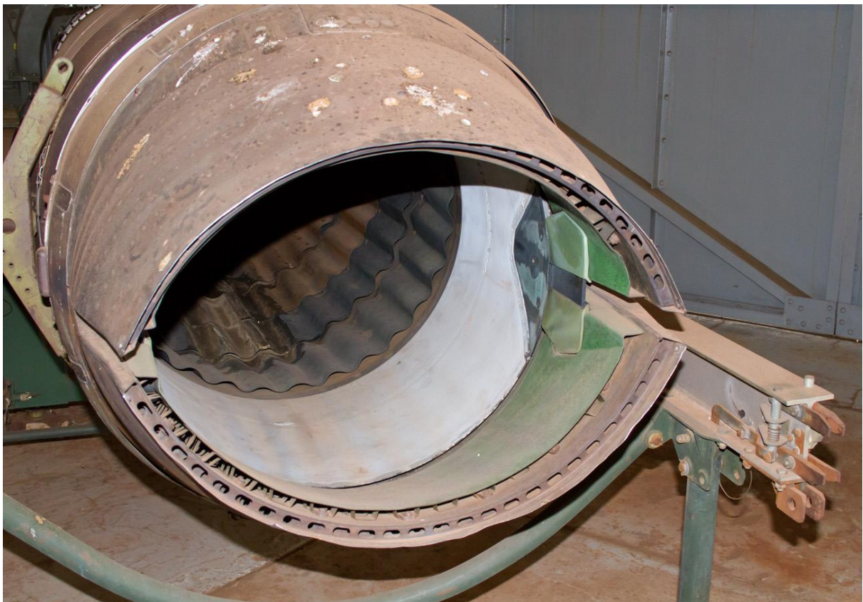
09B on its engine cradle at Swartkop. The clamshell halves are in the closed positions.
