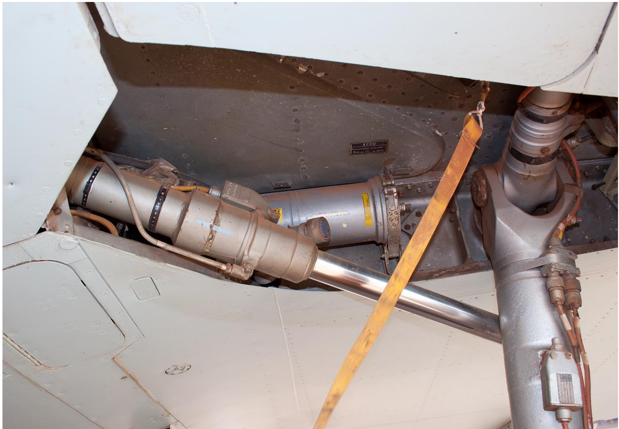
Retraction piston on the left main undercarriage leg.
