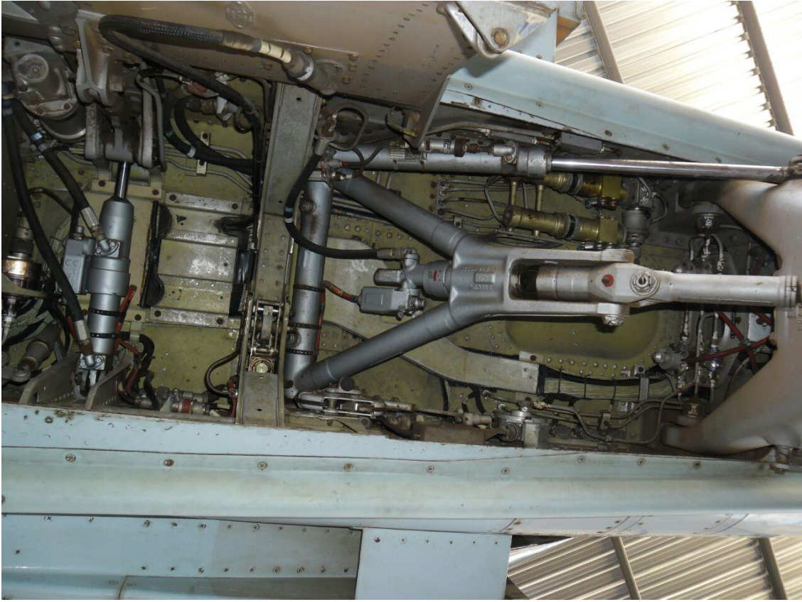
Forward section of nose gear bay on BZ #818. The nose gear retraction strut configuration of the BZ is different to that of the single seaters which have a single centrally mounted retraction piston and lack the Y-support arm.
