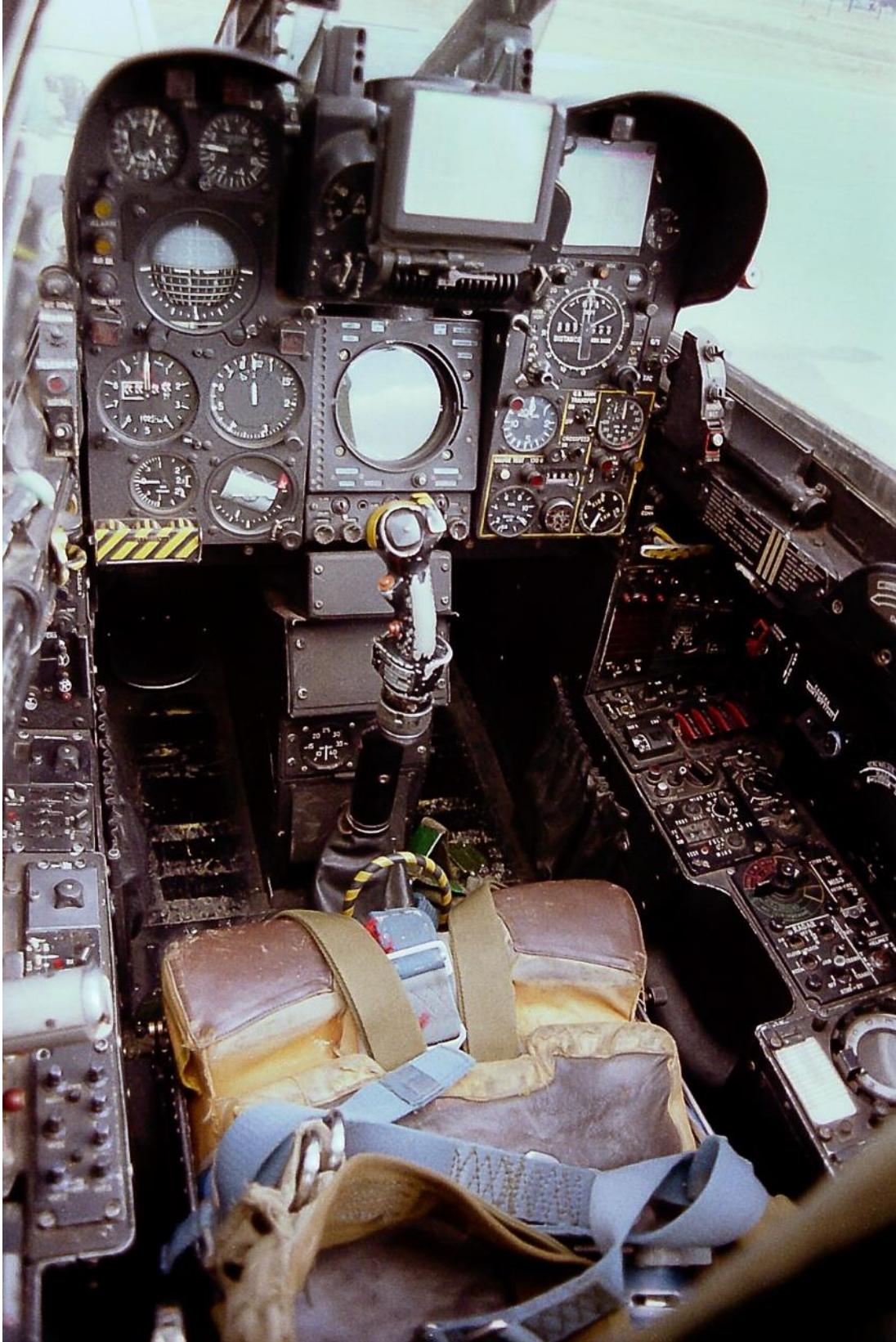
EZ cockpit. Layout of the instrument panel is largely similar to that of the CZ. The location of the central radar display is higher up than on the CZ.
