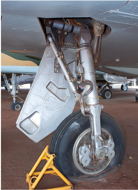
Details of CZ wheel brake assemblies and hydraulic hoses. BZ was similar.
