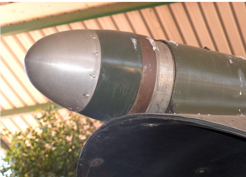
Drag chute cover. On some aircraft, the green portion would be a metallic blue. These covers were reused and some were rather badly dented.
