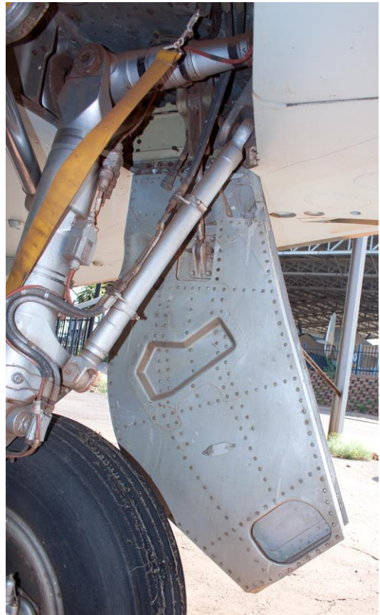
Left hand main landing gear leg detail. The diagonal stabilizing arm configuration is different to that used on the DZ, D2Z, EZ, RZ and R2Z.
