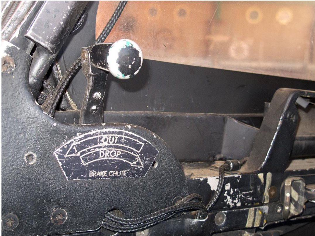
Brake chute actuation handle on the left side of the cockpit. The handle at the bottom right with diagonal yellow lines is the canopy jettison lever.
