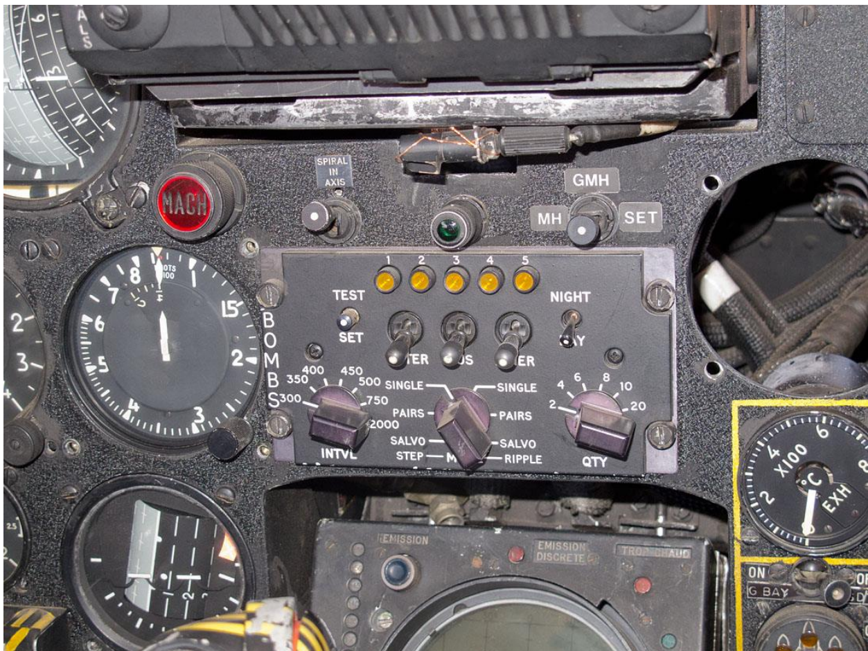
The weapons release selector panel. The switch at the left is the bomb intervalometer, in the middle is the fire control selector for the JL-100 rocket pod and on the right is the gun round selector (author's assumption).
