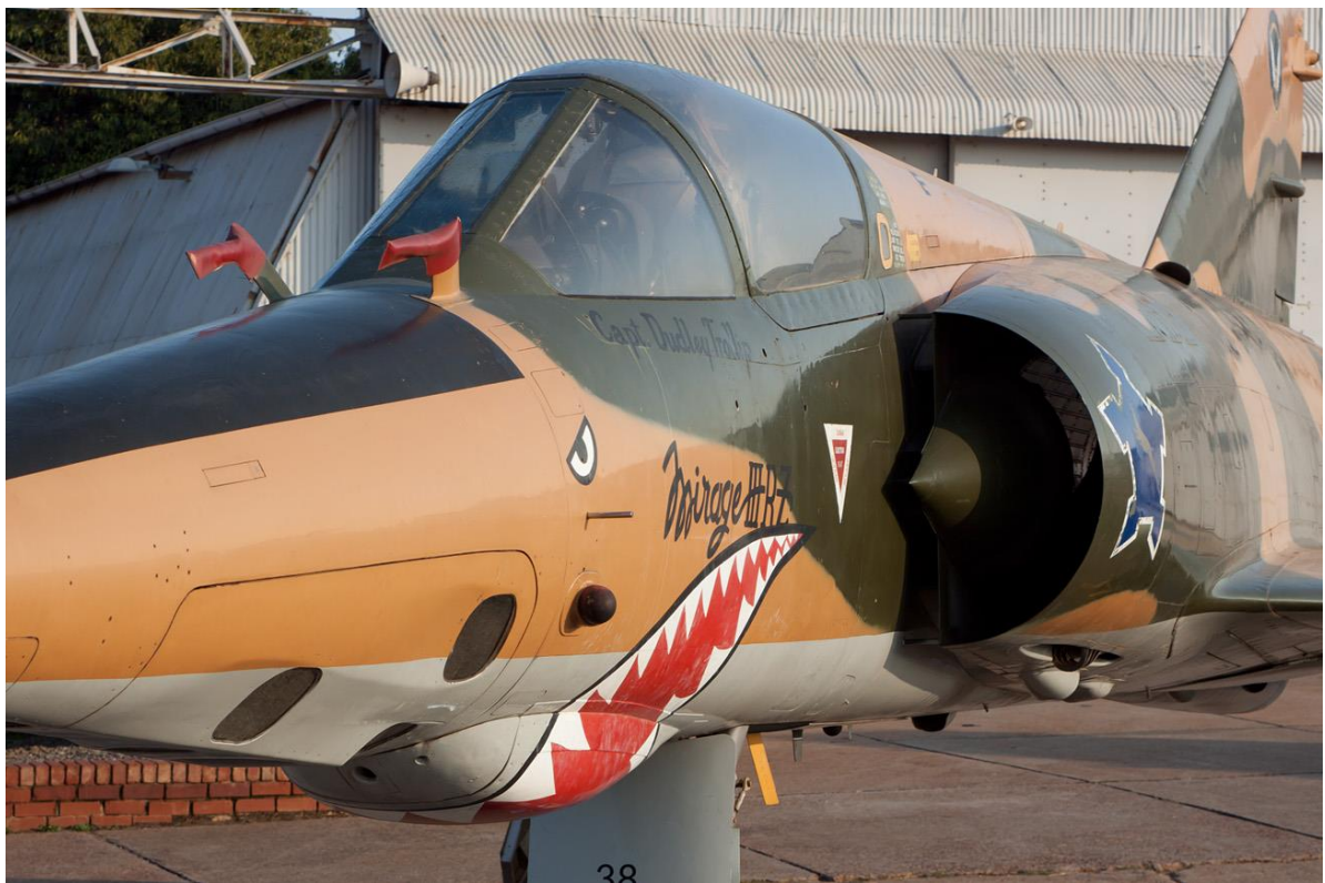
The dual total pressure probes located ahead of the windshield on RZ #838 with red FOD covers on. Just beneath the eye can be seen the thin straight incidence probe. Below that is one of the "cat balls" CRWS antennae.
