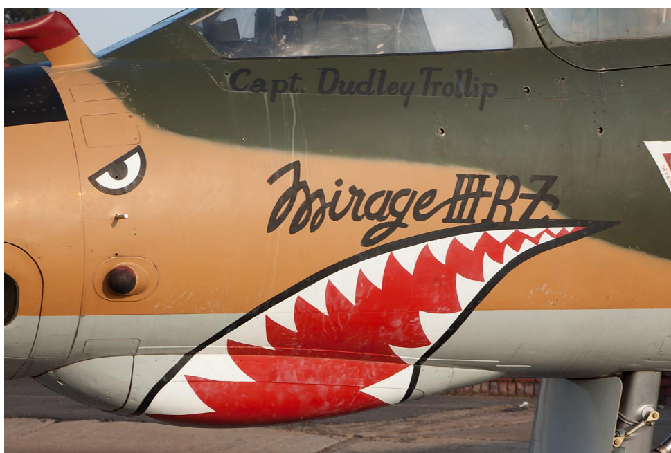
Doppler fairing on RZ #838. The teeth cover the dielectric panel.
