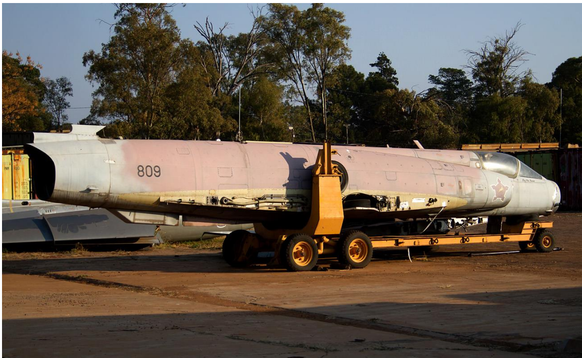
Starboard view of CZ #809 clearly showing the box like fairing (beneath the aircraft number "809") which would house the RIMS chaff and flare dispenser. Note the forward CRWS antennae just aft of the nose cone break.
