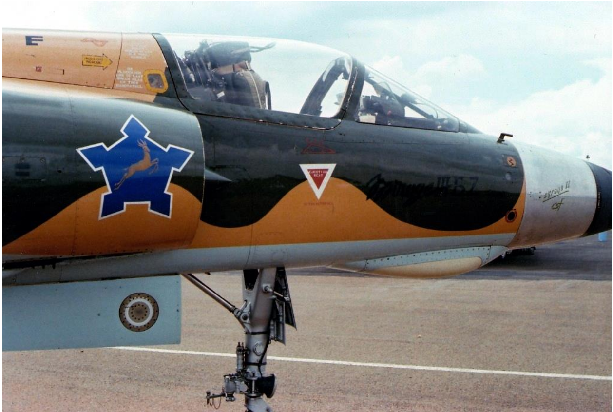
EZ – the smaller total pressure probe is located ahead of the windshield. There are two of these, one each side of the windshield. These are visibly smaller than those fitted to the RZ and R2Z.
