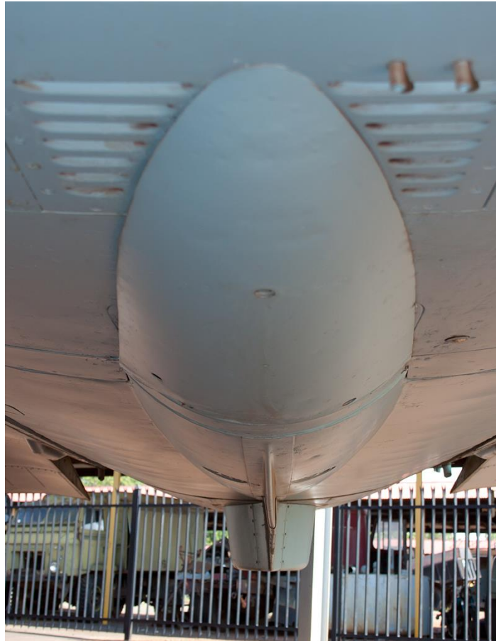
Underside view of CZ #805 clearly showing the simple blade ventral strake with the box like fairing to the rear which would house the RIMS chaff and flare dispenser.
