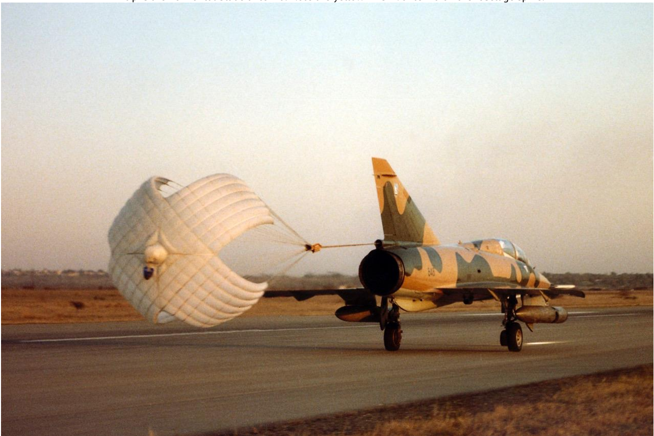
D2Z #848 with all UHF antennae painted over. The TACAN antenna is visible on the fuselage spine.
