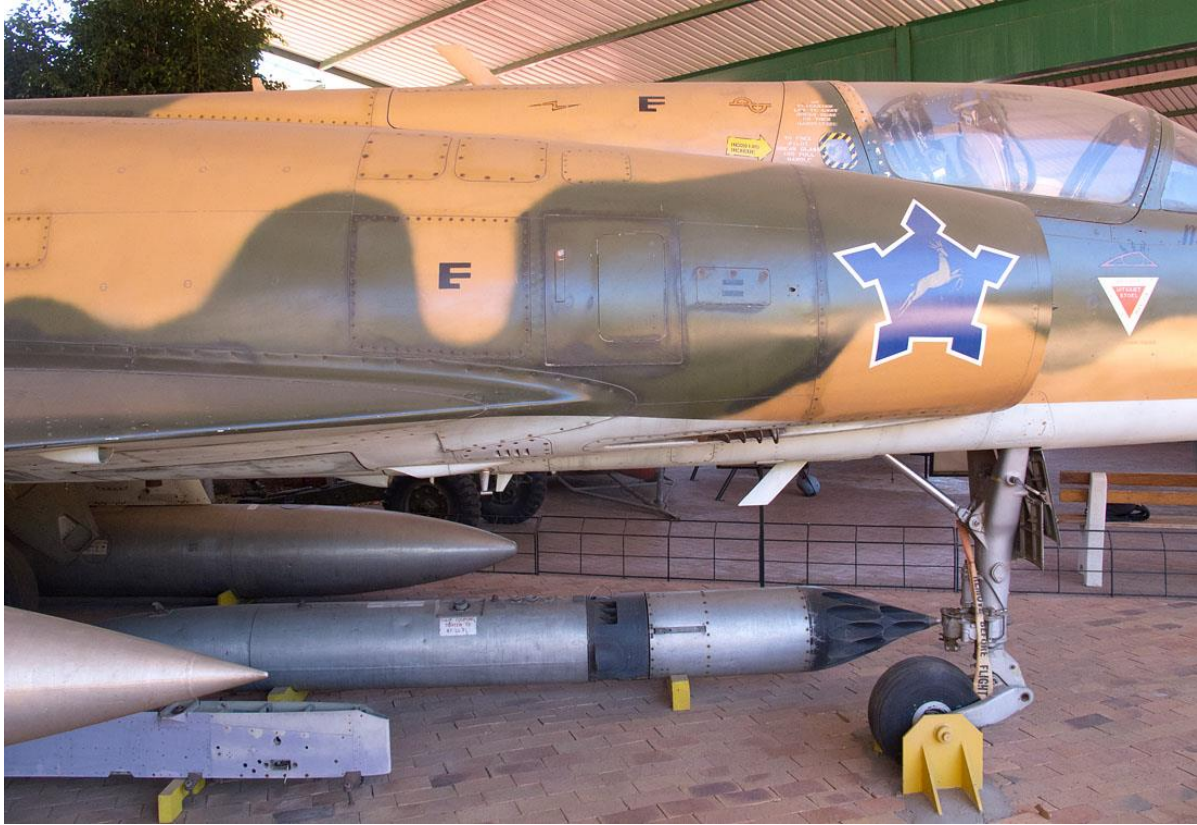
A small trapezoidal shaped antenna can be seen just aft of the nose gear bay – its purpose is unknown. Just aft of this is the impact temperature probe. The large blade antenna on the nose gear door has replaced the original circular conformal IFF antenna.
