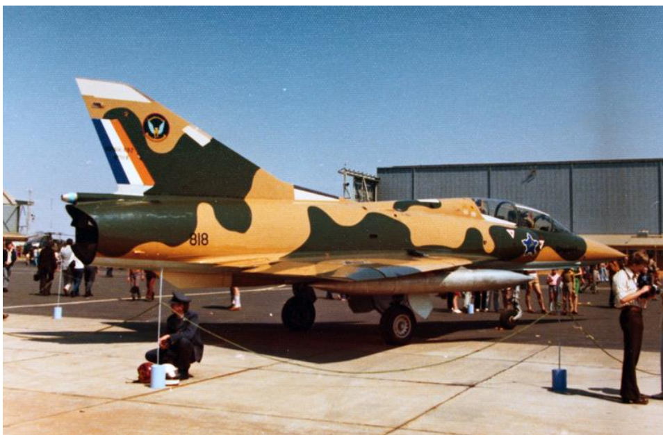
BZ #818 in fresh coat of hard edge gloss camouflage. The conformal dielectric panels have not been painted over. Note the large white panel aft of the canopy.
