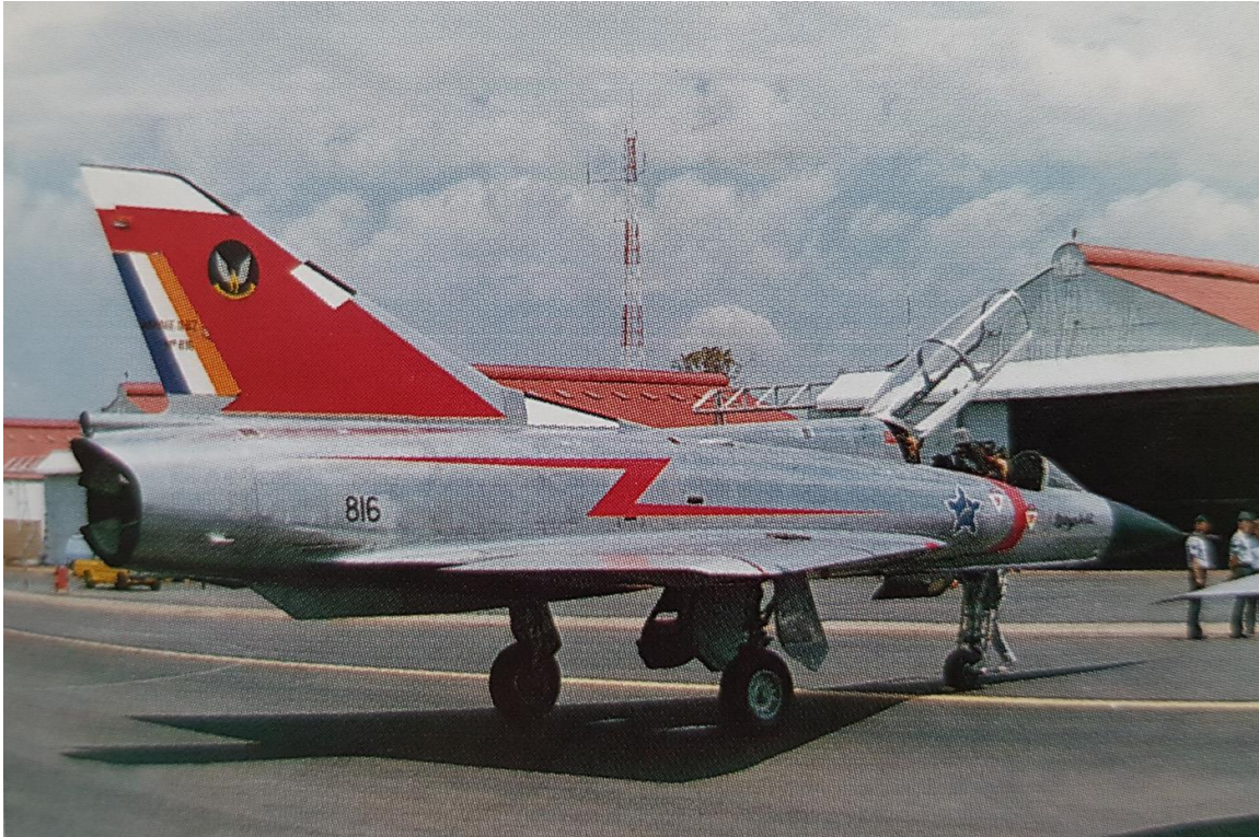
BZ #816 - note that the large white conformal dielectric panel does not appear aft of the canopy.
