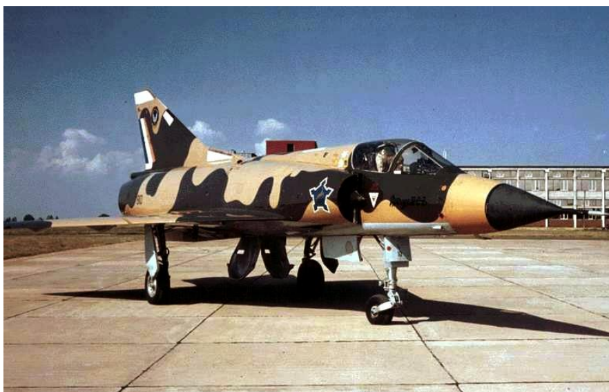
IIICZ - note the circular conformal antenna on the sideways opening nose gear door as well as the large rectangular conformal dielectric panel located towards the rear of the avionics hatch aft of the canopy.
