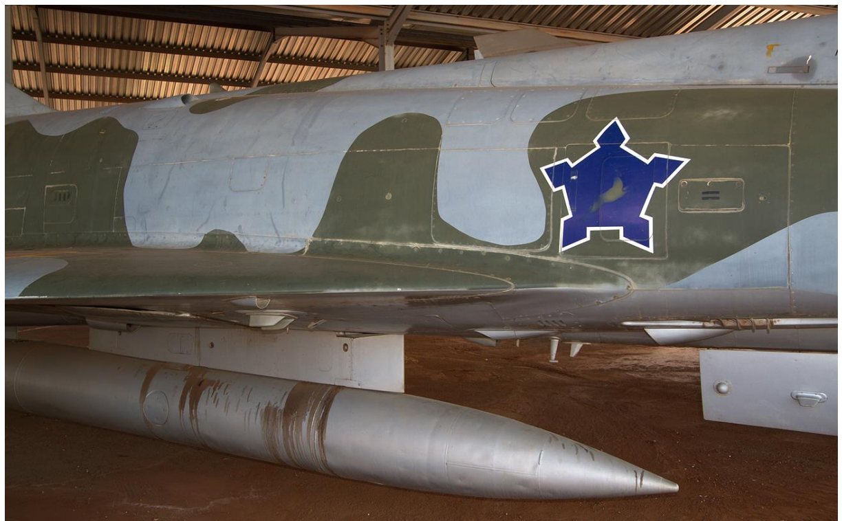
Another close-up of RZ #83. A dual blade antennae can be seen just aft of the wing leading edge scoop. It is assumed that this was associated with navigation avionics specific to the RZ as it does not appear to have been fitted to the R2Z. Aft of the nose gear door on the fuselage underside, a small blade antenna and the impact temperature probe can be seen.
