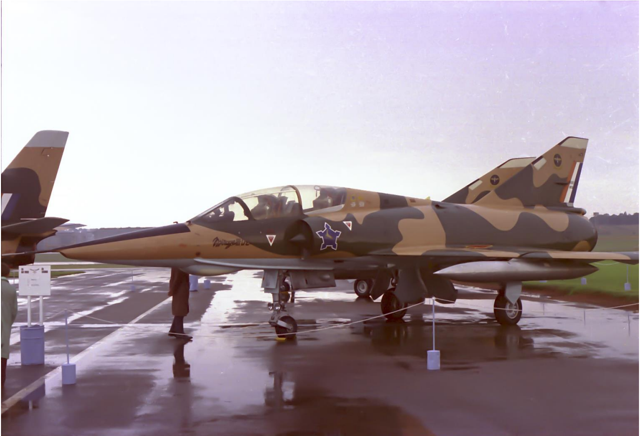
DZ #840 - note the distinctive doppler antenna just ahead of the nose gear. The yellow TACAN antenna on the fuselage spine can just be made out in this photo just forward of the engine cooling intake scoops.
