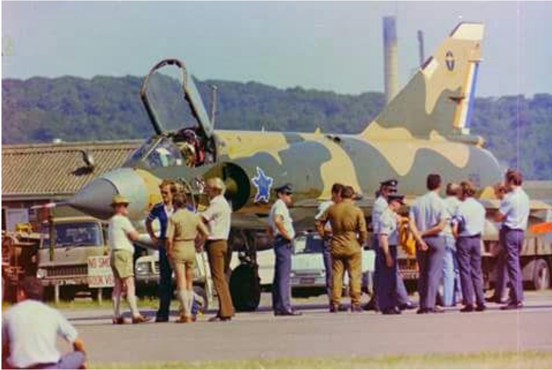
Possibly EZ #825. An additional small blade antenna has now been added to the aft end of the avionics bay on the spine. The original yellow TACAN antenna is clearly visible ahead of the vertical stabilizer. The UHF conformal antennae on the vertical stabilizer are still clearly present.
