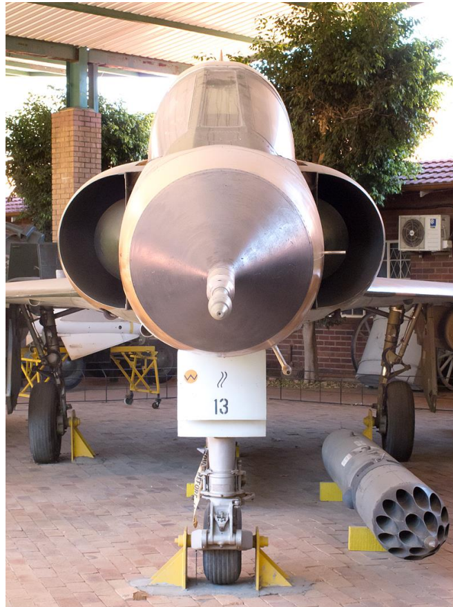
CZ #813 showing the pitot probe and its total pressure orifice. The supplementary total pressure probe can be seen on the lower fuselage offset to port. This was typical for the BZ and CZ.
