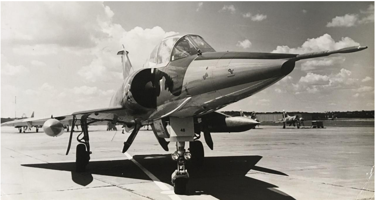
D2Z #848. The starboard total pressure probe is visible ahead of the windshield. These are similar in size to those on the DZ and EZ.
