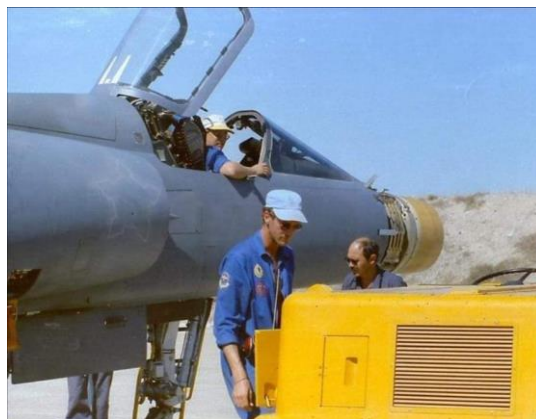
Unidentified CZ, in low visibility blue-grey camouflage, with radar exposed. Note the open latches for removal of the nose cone.
