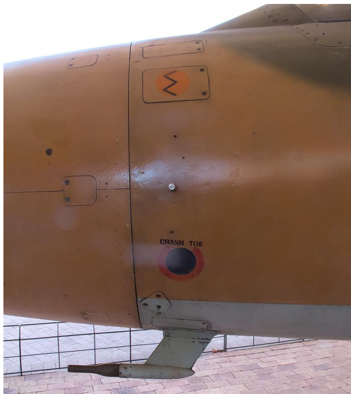
The single total pressure probe located on the lower left forward fuselage of CZ #813. The round hole above this is the crash tow tube.
