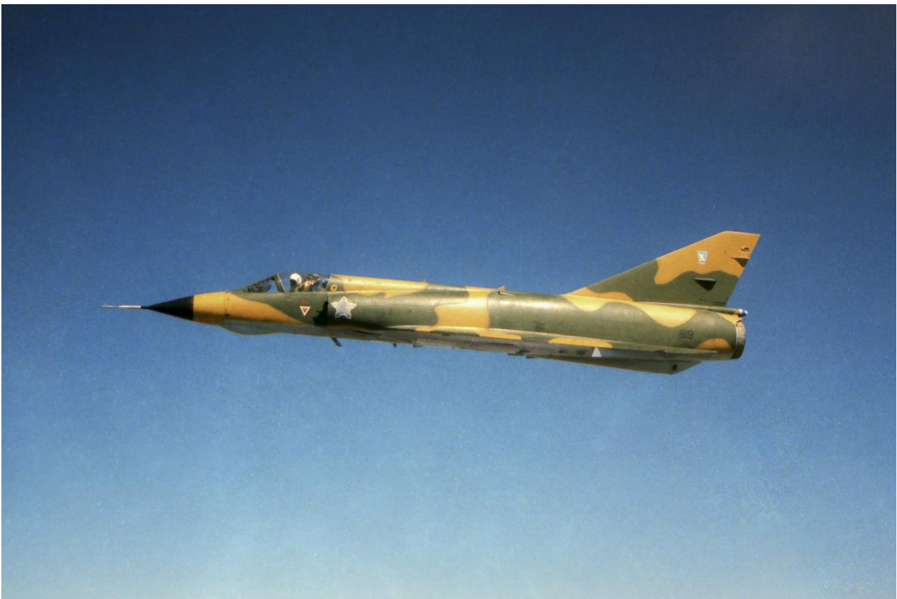
Final EZ antenna configuration on EZ #819 which appears to have coincided with application of the late matt soft edge buff/green camouflage. The conformal antennae on the vertical stabilizer have been painted over. A large blade antenna has been added to the nose gear door. The two blade antennae are visible on the fuselage spine, the rearmost one being for TACAN.
