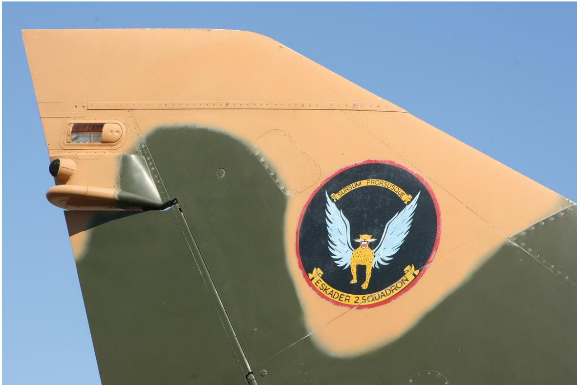
Round black CRWS antenna above the rudder on RZ #838. The original pancake shaped antenna has been retained.
