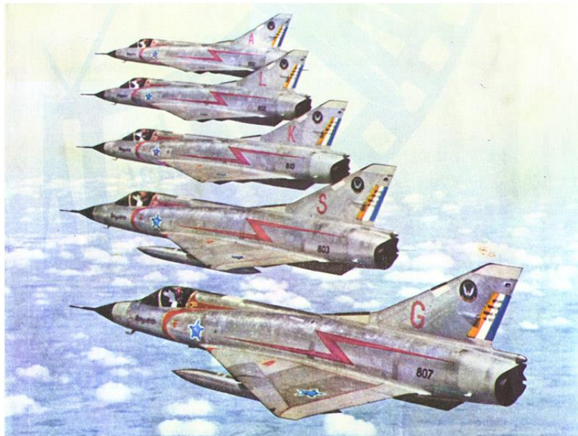
Mirage IIICZs in delivery scheme clearly showing the various conformal antennae as noted in the text above.
