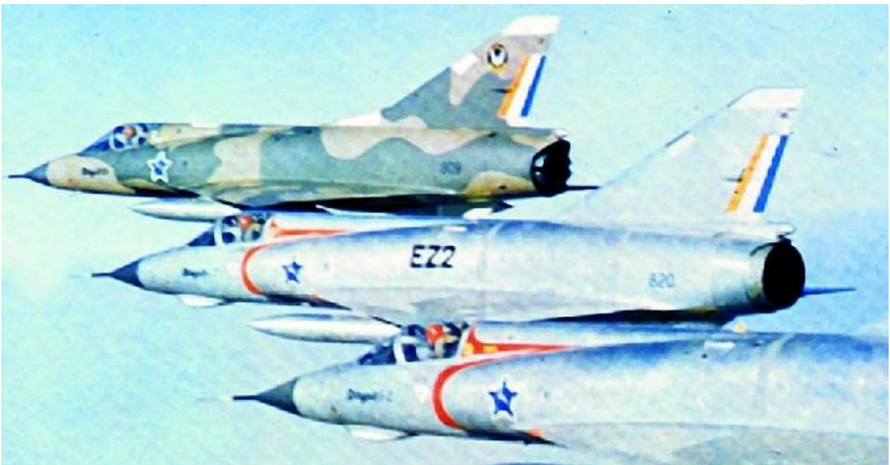
Two natural metal EZs in formation with a camouflaged CZ. The conformal antennae on the vertical stabilizer of EZ #820 are readily apparent. The doppler antenna beneath the nose of the two EZs are also apparent. The yellow TACAN blade antenna on the fuselage spine is visible on the closest aircraft. This is not present on the CZ.
