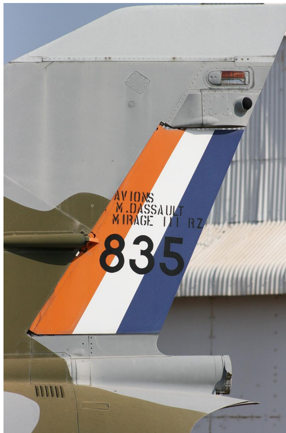
Round black CRWS antenna above rudder on RZ #835. The pancake shaped antennae has been removed.
