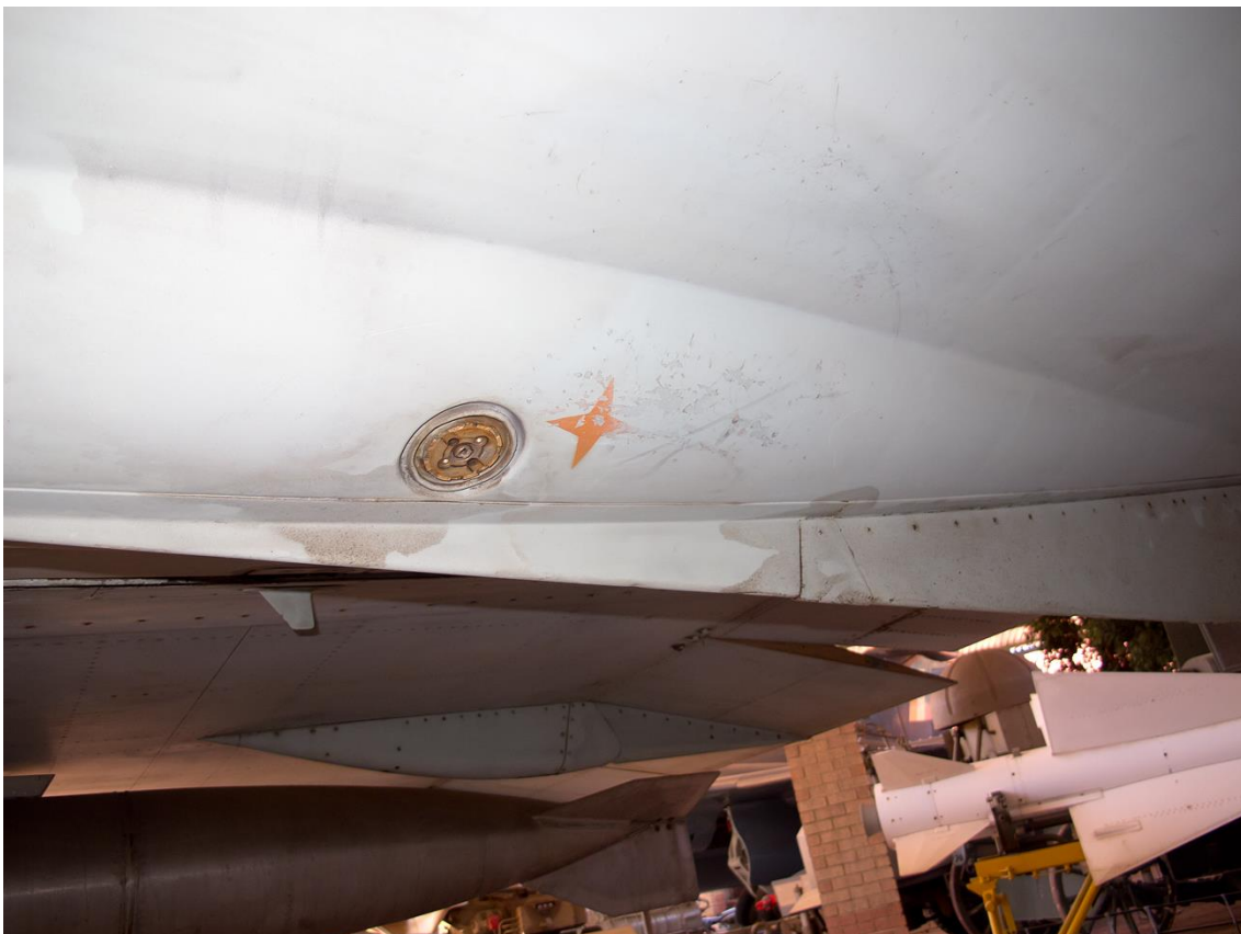
CZ #813 - this antenna is the underside TACAN antenna and is offset to starboard.
