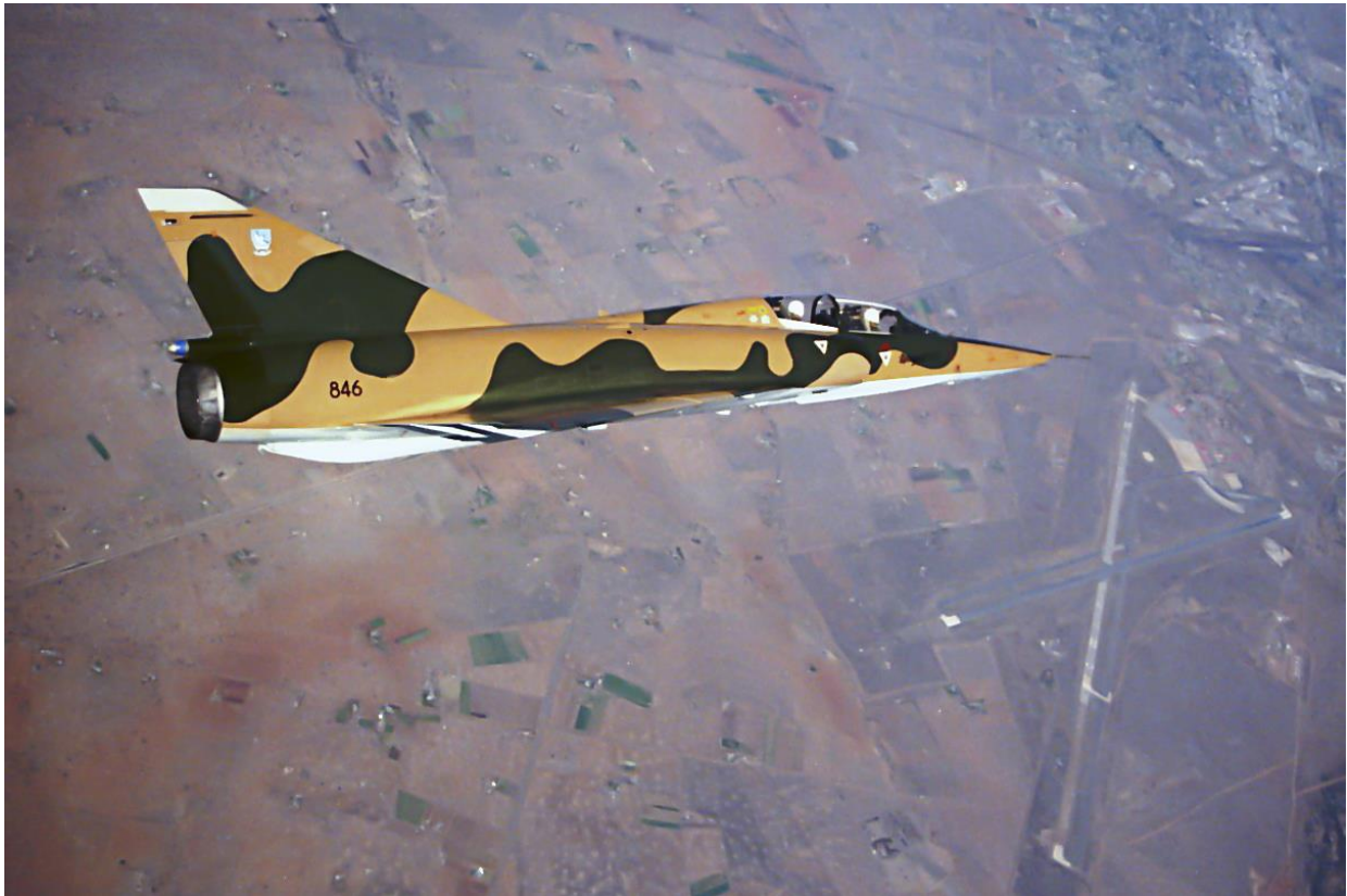
D2Z #846. The white antennae panel on the leading edge of the vertical stabilizer has been painted over. The black stripe beneath the white fin tip is the horizontal blade antenna. Note the yellow TACAN antenna on the fuselage spine.
