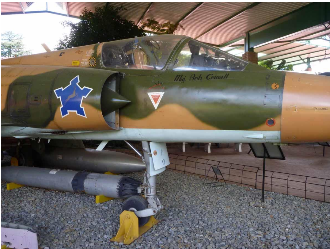
CZ #813 - the large blade antennae can be seen on the spine and on the nose gear door.
