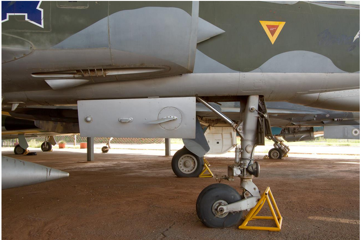
RZ #835 – three antennae on the nose gear door : large (possibly IFF) and small (CRWS) blade antennae and small round CRWS antenna to the rear. The CRWS and smaller blade antennae were originally black and may have erroneously been painted over when #835 was repainted.
