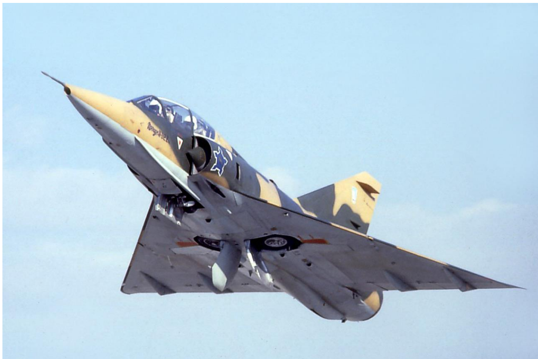
Another D2Z showing the ventral fairing with the arrestor hook protruding out the rear of the fairing. Note that the arrestor hook fitted neatly into a slot down the center of the fairing.
