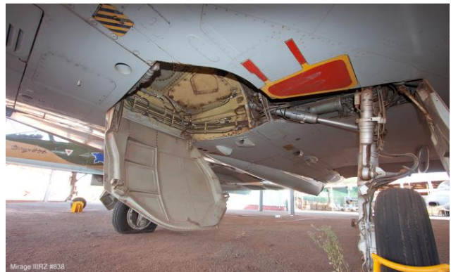
RZ #838 left main undercarriage leg looking towards rear of aircraft. Note absence of slots in the doors. (EZ, DZ, D2Z and R2Z the same)
