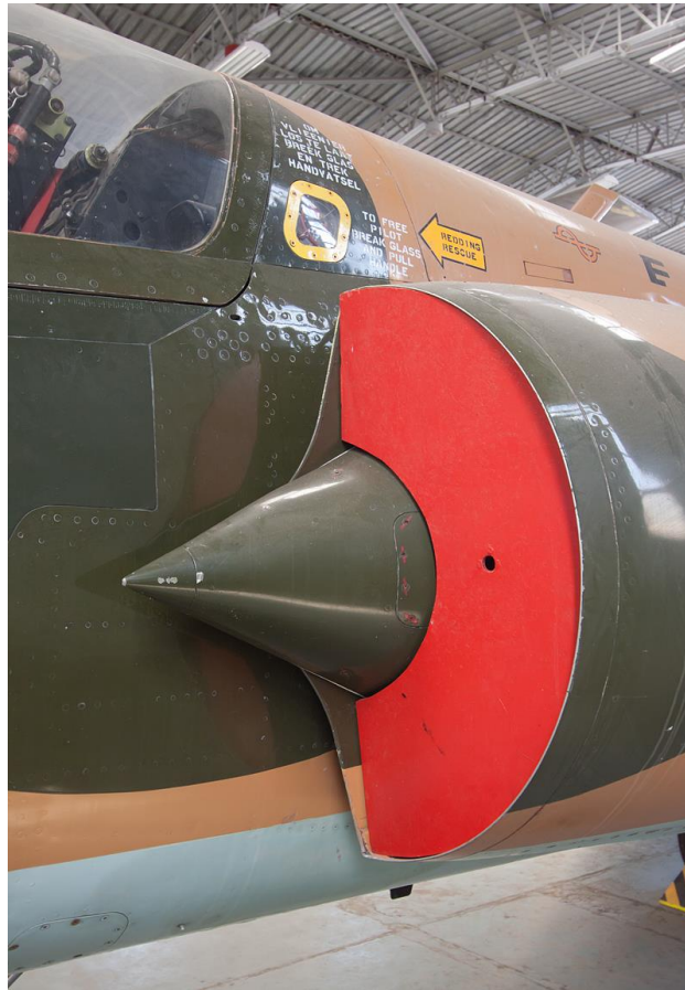
Air intake of R2Z #857 which clearly shows the distinct scalloped leading edge splitter plate, indicating that the aircraft has been fitted with the higher thrust (increased air flow rate) Atar 09K50 engine.
