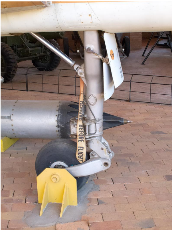
CZ #813 nose landing gear leg. There are no landing lights located on leg. (BZ the same)
