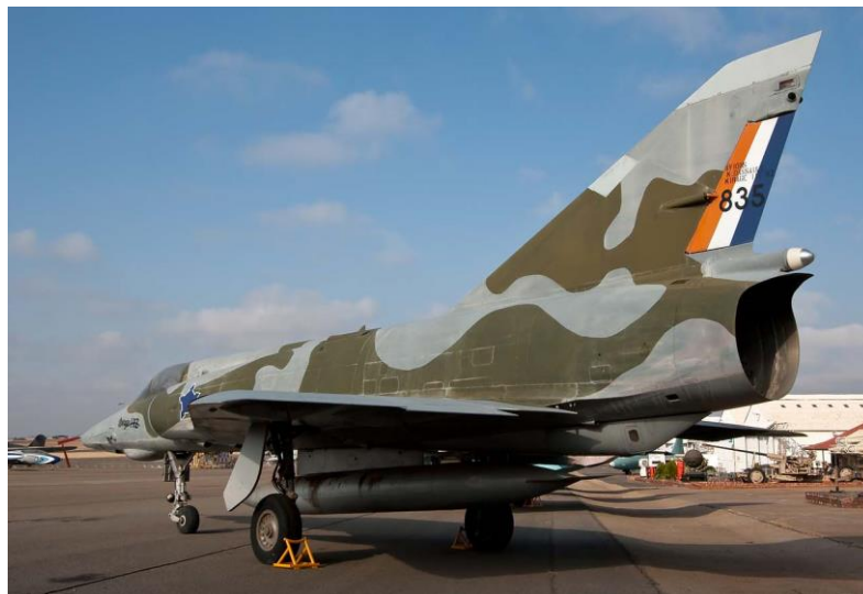
By comparison, RZ #835 with the "3 dimensional" ventral fairing which housed additional fuel. Note the inspection window to the rear of the fairing. DZ, EZ and R2Z would have been similar.
