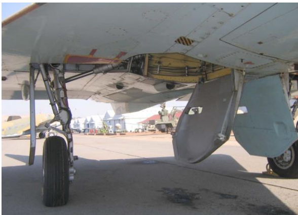
BZ #818 right main undercarriage leg looking towards rear of aircraft. Note the slots in the doors. (CZ the same)
