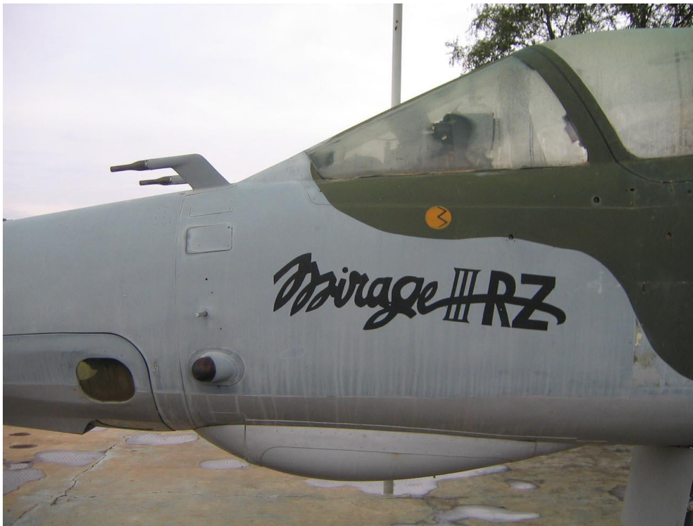
RZ #835 showing Doppler antenna, small black CRWS antenna and large pitot probes.
