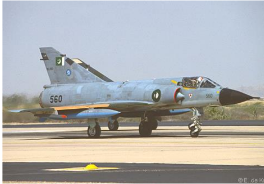
Mirage IIIIO #560 of Pakistan Air Force with what can only be ex-SAAF Mirage IIIIE wings in the original SAAF camouflage.
