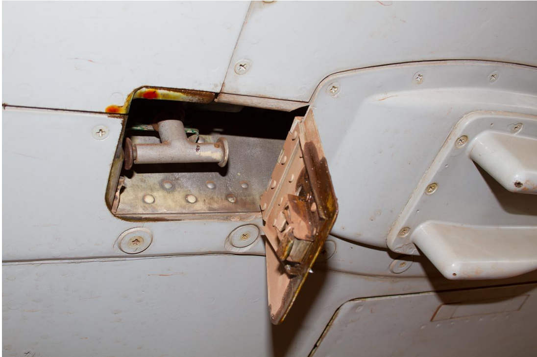
RZ #838 main undercarriage door opening handle located inside the wing. The cover is painted yellow and black on the outside. This is similar for both wings.
