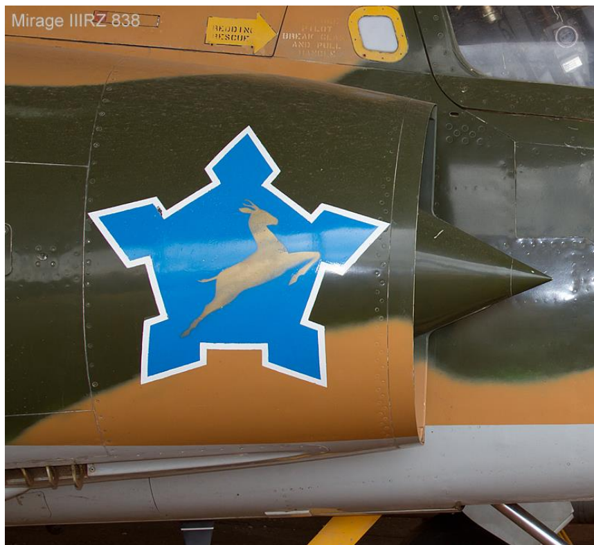
Air intake of RZ #838 which shows the straight leading edge splitter plate, indicating that the aircraft has been fitted with the Atar 09C engine.
