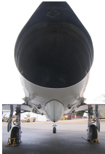
By comparison, rear view of RZ #838 with the ventral fairing which would house additional fuel.
