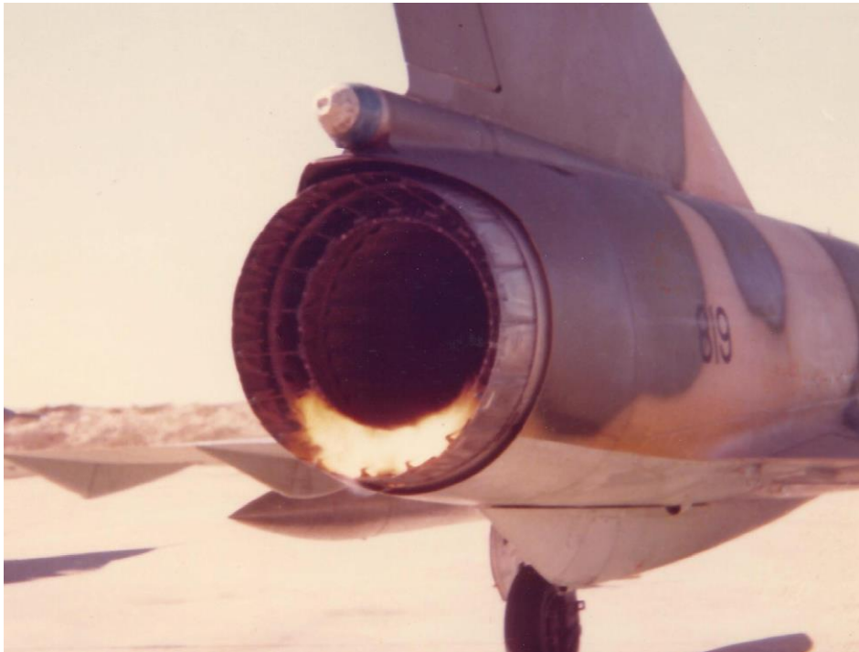
Atar 09C on EZ #819 and as fitted to DZ, D2Z, EZ and RZ annular type variable exhaust nozzle. The R2Z uses the Atar 09K50 which has a similar exhaust nozzle arrangement as for 09C.
