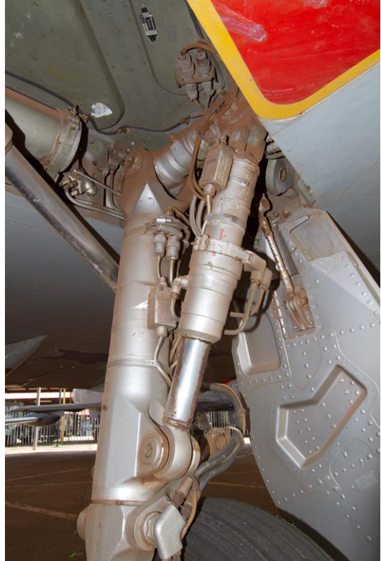
RZ #838 left main undercarriage leg (similar view to the image to the left). Note that the front stabilization arm now has a hydraulic ram for different retraction kinematics. The empty bracket for the C style arm can be seen in the right hand corner of the bay.
