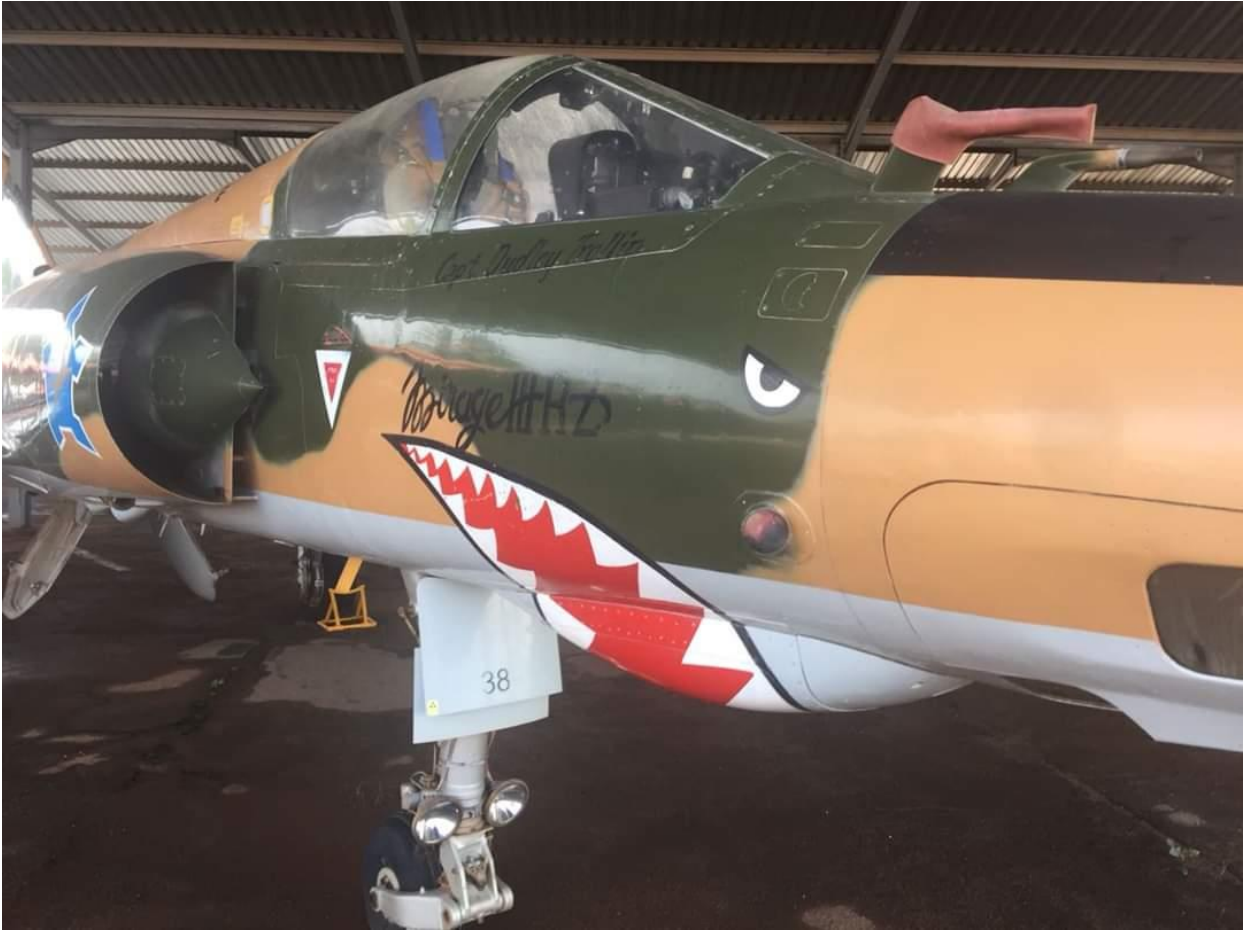
RZ #838 – note doppler antenna, small black CRWS antenna and large pitot probes – the one has a red cover on it.
