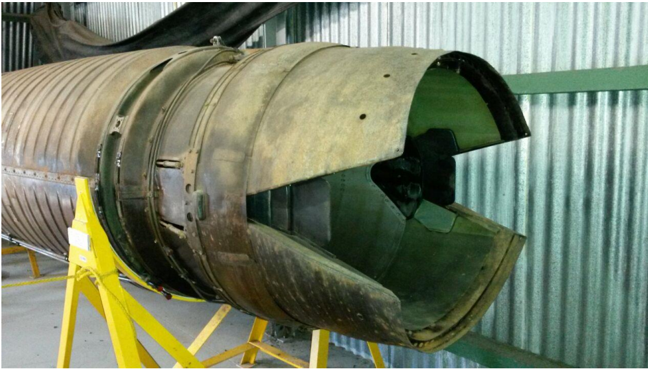
Atar 09B as fitted to the BZ and CZ. This illustrates the clamshell type variable exhaust nozzle.
