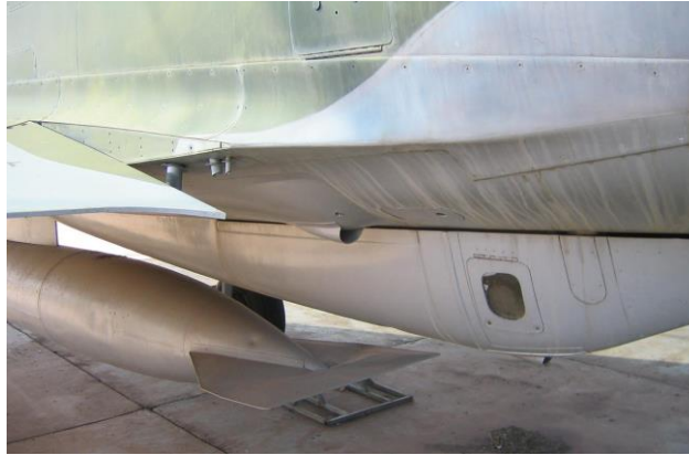
Close up image of ventral fairing on RZ #835 showing the fuel tank inspection window. Note also the configuration of the external RP825 fuel tank fins
