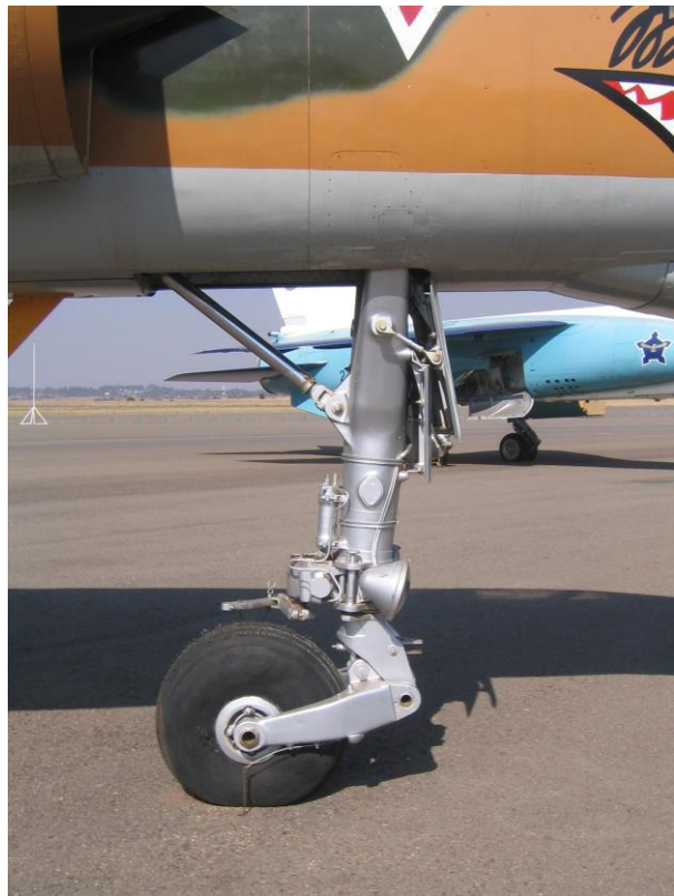
RZ #838 nose landing gear leg. Note one of the dual landing lights located on leg. (EZ, DZ, D2Z and R2Z the same)
