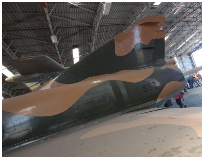
RZZ #857 – note the horizontal blade antenna near the top of the vertical stabilizer.
