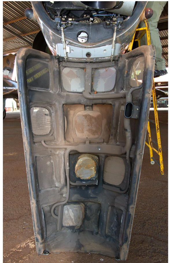
Details of interior of camera windows complete with ducting – RZ #838
