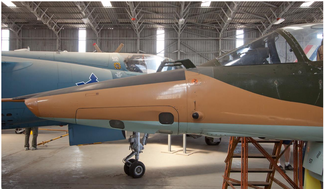
RZ #857 – no doppler antenna. Black CRWS antenna is present.
