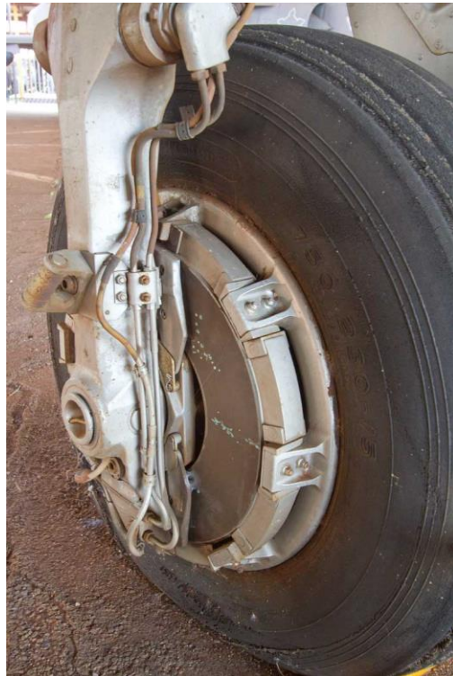
RZ #838 main wheel brake assembly. (EZ, DZ, D2Z and R2Z the same)
