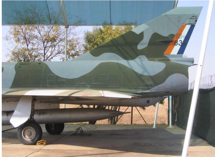
Vertical stabilizer of RZ #835 – standard SAAF CRWS antenna above rudder.
