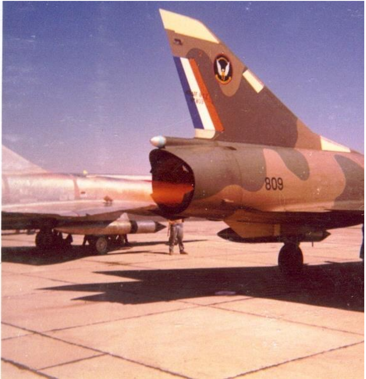
CZ #809 demonstrating its 09B in action with clamshell exhaust arrangement.
