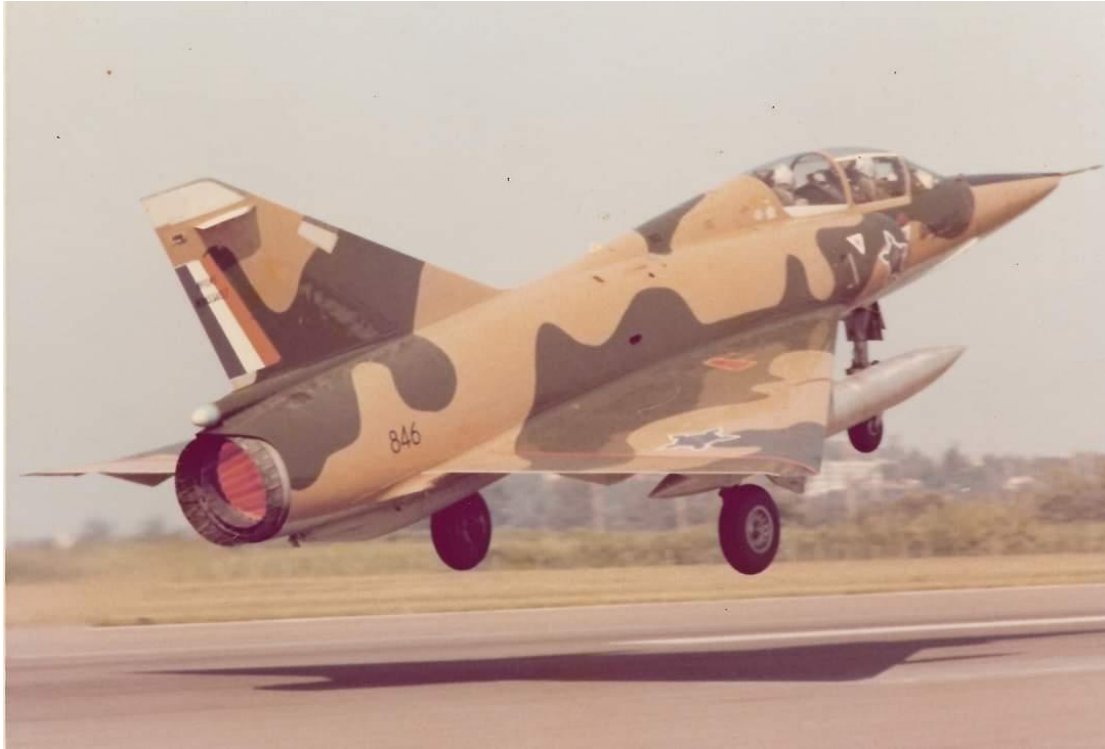
D2Z #849 showing the aft ventral fairing with the arrestor hook protruding out the rear of the fairing. D2Zs were the only SAAF Mirages so equipped.
