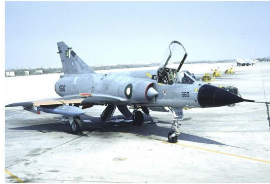
Mirage IIIIO #560 of Pakistan Air Force with what can only be ex-SAAF Mirage IIIIE wings in the original SAAF camouflage.
