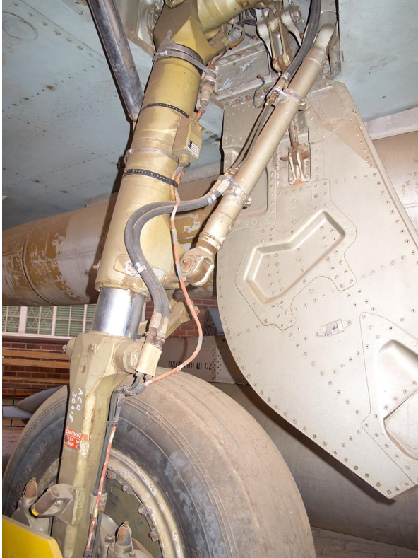
CZ #813 left main undercarriage leg. Note that the front stabilization arm connects to a bracket inside the bay (top right in image).
