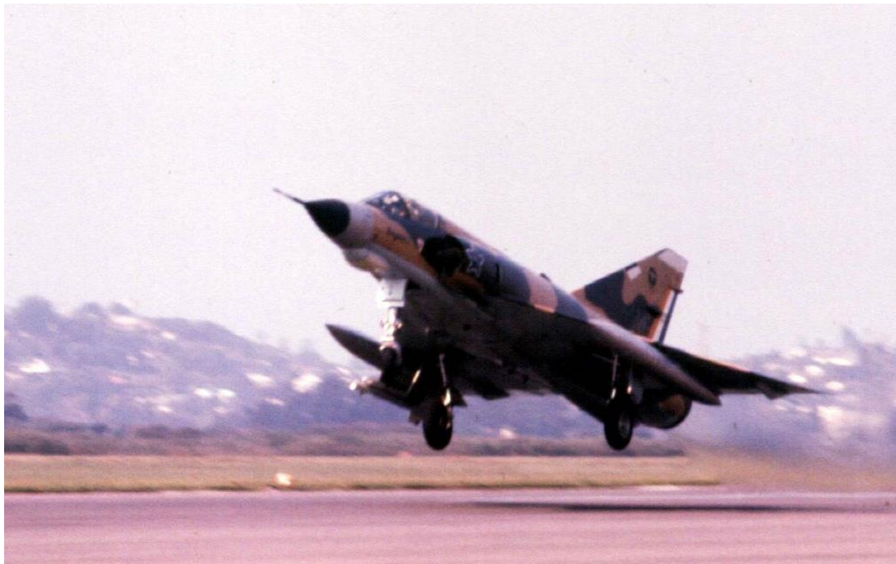
EZ with two RP18R supersonic wing tanks and a single AIM-9B air-to-air missile on the starboard outer pylon. Note that there is no pylon on the port outboard harp point. The elevon aerodynamic fairing is in place.
