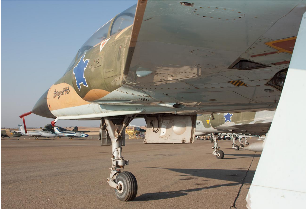
Port 30mm cannon muzzle trough on BZ #818. Note that the BZ does not have the muzzle brake assembly. The fact that no gun barrels protrude and that the gun palette does not have the forward facing air scoop indicates that the gun pack is not fitted.
