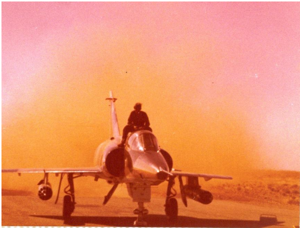
Demonstrating that anything was possible in the SAAF, here's an unidentified R2Z (note camera window on forward fuselage and lack of doppler antenna) with a non-typical (for the reconnaissance Mirage) offensive load of two JL-100 combined fuel tank / rocket pods.
