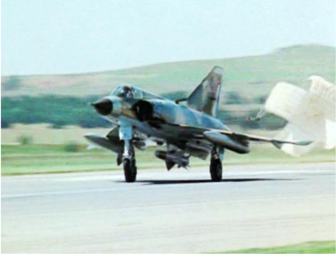
CZ with Matra R530 on the centerline pylon and two wing mounted RP18R 500 liter fuel tanks..
