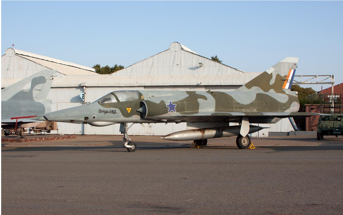
1,100 liter RP825 fuel tank carried on the centerline station only, as demonstrated in this image of RZ #835 at Swartkop. Note the distinct nose down angle of the tank and the flat horizontal tail fin.
