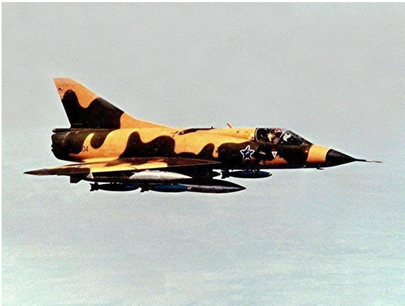
CZ #804 with centerline RP825 fuel tank and two wing mounted 110G wing tanks carrying practice (blue colour) Mk81 or Mk82 GP bombs in tandem. The outboard wing missile pylons are fitted, but the missile launch rails are not.
