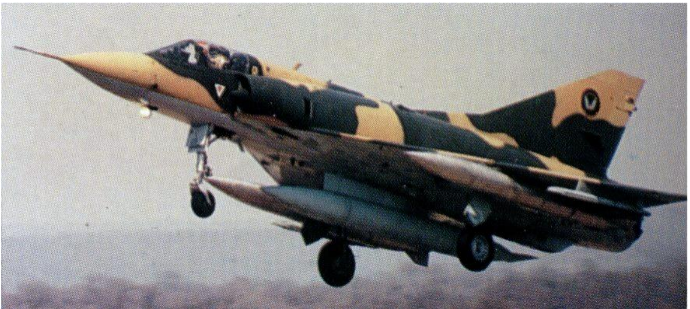
CZ with ferry configuration including a centerline RP825 and two wing mounted 110G tanks (note fins). Outboard wing pylons are present complete with Aero 3B missile launch rails for AIM-9B Sidewinder missiles.
