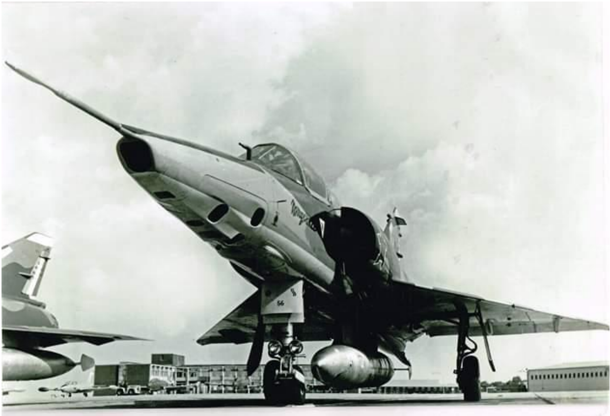
R2Z #857 with a single RP62 1,300 liter fuel tank mounted on the centerline. This was not a common configuration
