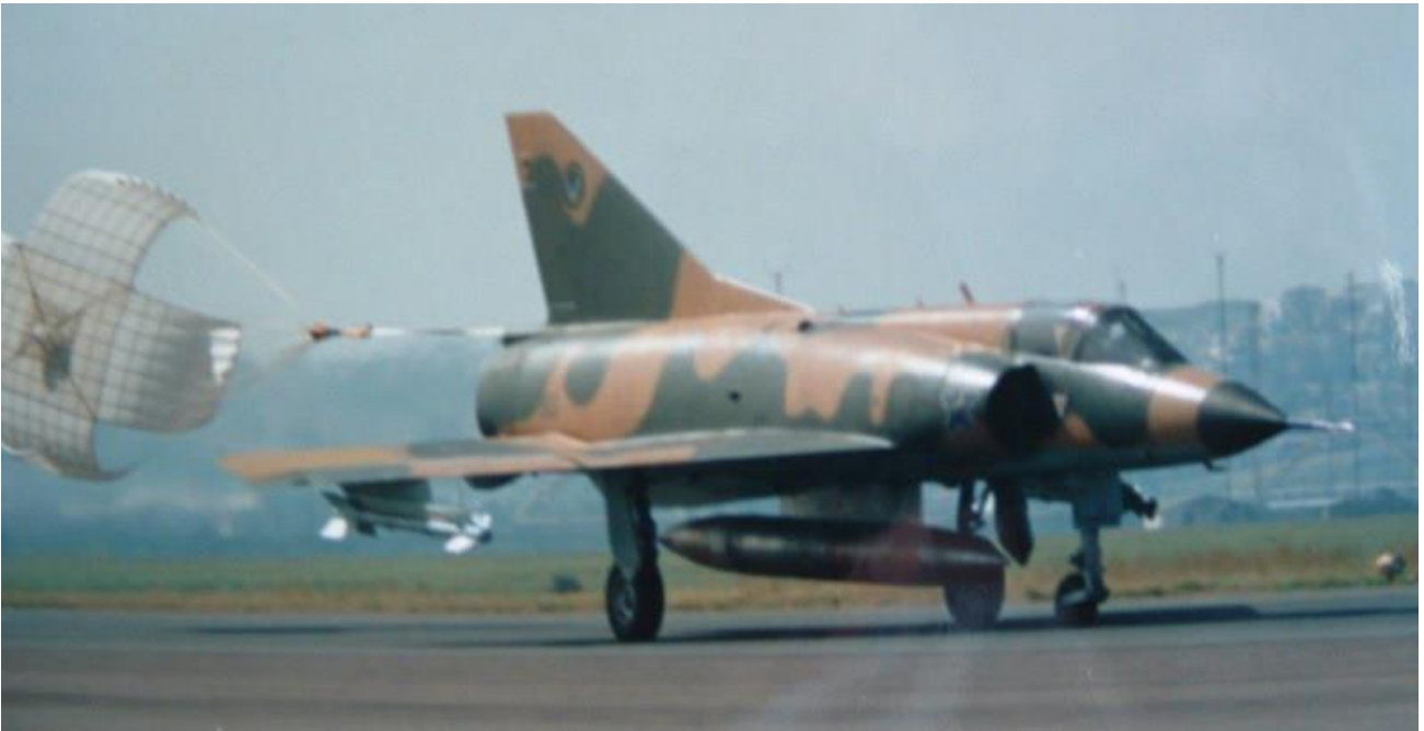
Two images of possibly the same CZ (soft edge buff/green camouflage (original pattern), radar nose with buff/grey nose cone, 2 squadron badge on the vertical stabilizer), likely seen at Durban. It would appear that the standard layout for ACM camps was a centerline RP825 fuel tank and two wingtip mounted V3B missiles.
