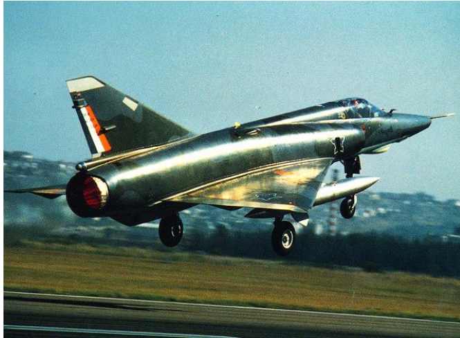
RZ with two wing mounted RP18R 500 liter supersonic fuel tanks.
