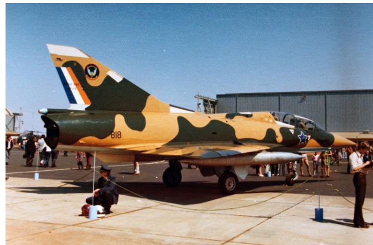
Another view of BZ #818 with RP18R fuel tanks.
