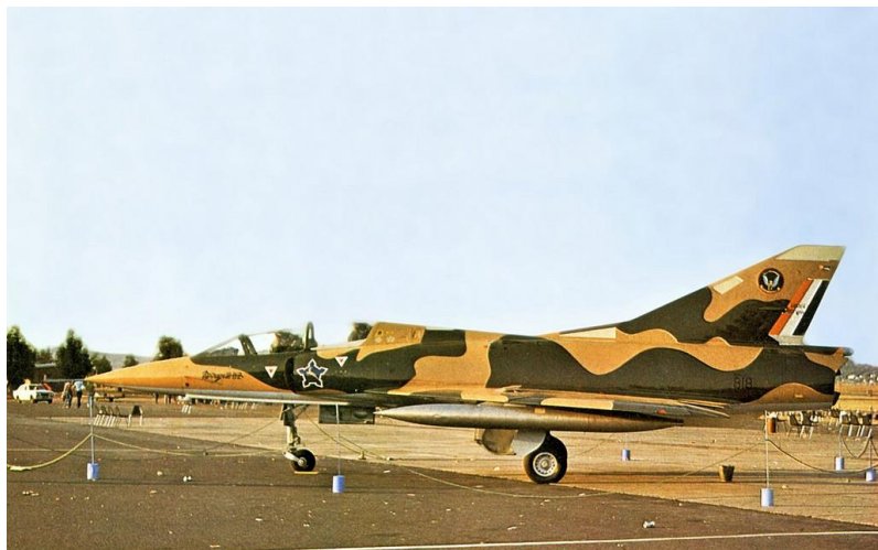
BZ #818 with two wing mounted RP18R 500 liter supersonic fuel tanks.
