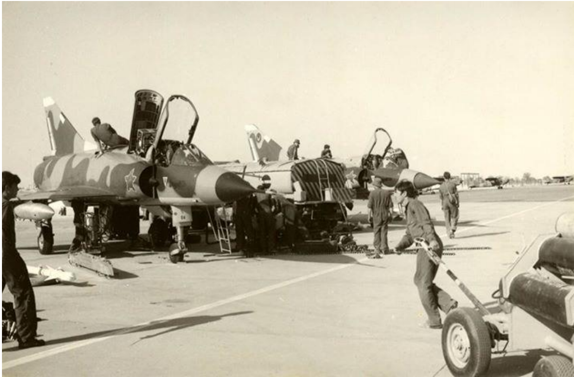
CZ #804 in the Operational Area (most likely Ondangwa) being prepared for a combat mission. RP18R fuel tanks are on the wings. An AIM-9B Sidewinder is on the ground to the left. Just to the right of the AIM-9B looks like the PM-3 bomb beam which will be installed on the centerline station to carry two bombs in tandem. #804 has been painted in the soft edge buff/green camouflage whereas the second CZ appears to still be in the original gloss hard edge camouflage.
