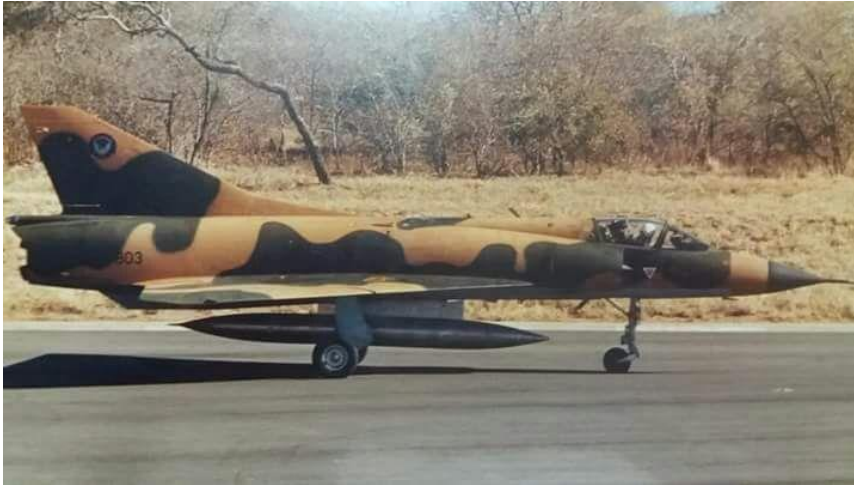
CZ #803 with single centerline RP825 supersonic fuel tank.
