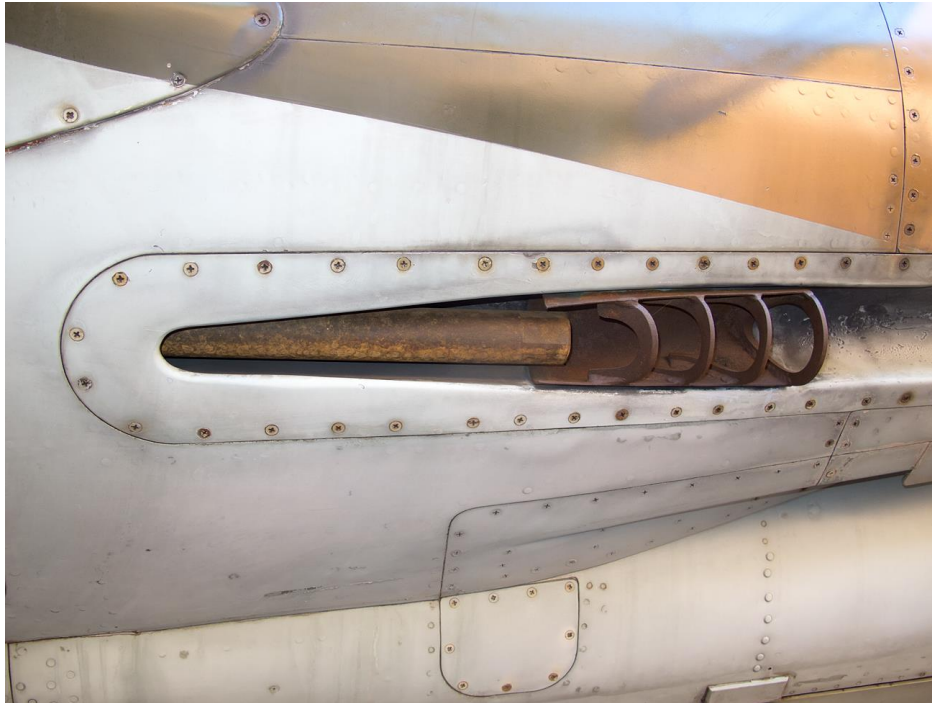
Starboard 30mm cannon barrel with muzzle brake on CZ #813. Note how far forward the canon barrel protrudes.
