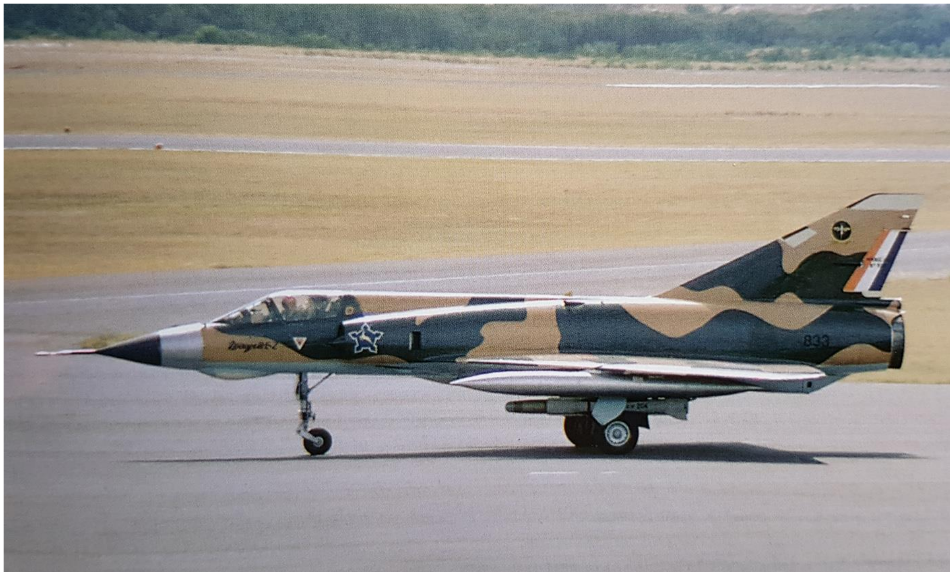
EZ #833 with two RP18R supersonic wing tanks and a Matra R530 air to air missile on the centerline.
