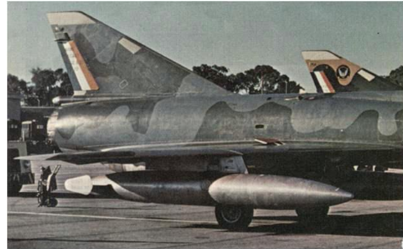
RZ #835 with centerline RP825 fuel tank.
