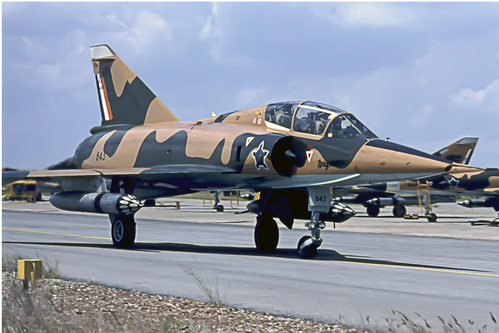
D2Z #843 providing a different perspective of the JL-100 pod. This would be a typical training and combat load for the D2Z. The yellow sections of the nose cone of the JL-100 are frangible covers over the rockets. Note the buff painted canopy frame and the white forward canopy strengthening strips. The cable ducting on the lower forward fuselage is also visible. The airbrakes are fully closed and the auxiliary air intake door is open.
