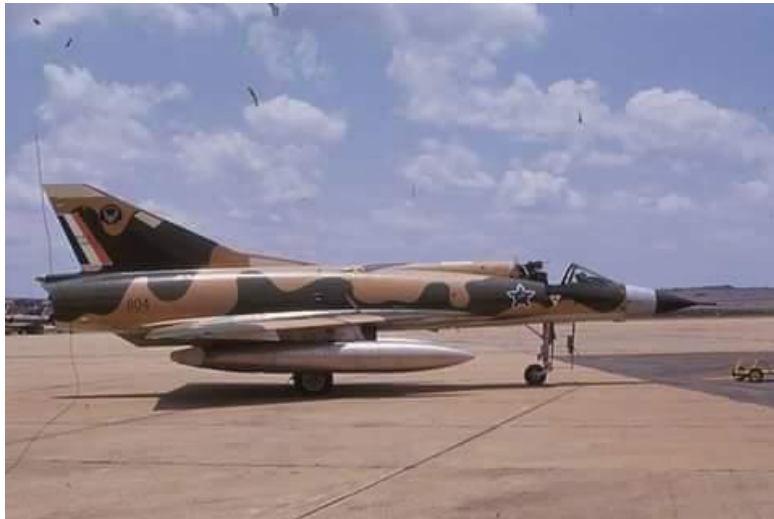
CZ #804 with two subsonic RP62 1,300 liter tanks on the inboard wing stations.
