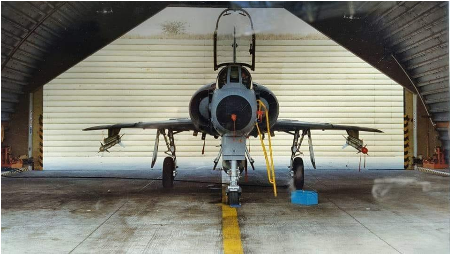
CZ #801 in its Hardened Air Shelter (HAS) with what appear to be two V3B air-to-air missiles on the outboard wing pylons and a centerline RP825 fuel tank. #801 is painted in the low visibility blue/grey camouflage scheme.
