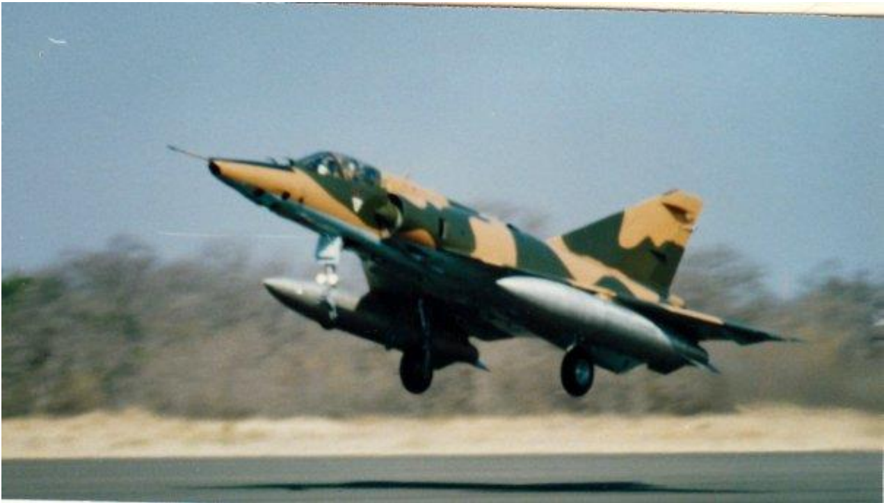
Great shot (even if low quality) of an R2Z with two of the large RP30 1,700 liter fuel tanks. The aircraft has been painted in the matt soft edge camouflage and all markings have been removed
