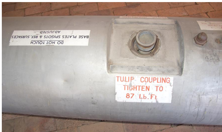
JL-100 wing pylon mounting details.
