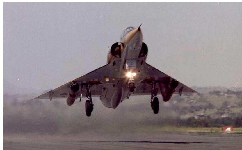
DZ with two JL-100 combined rocket / fuel tank pods.
