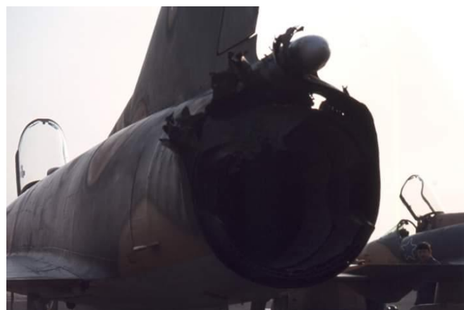
CZ #811 with AIM-9B air-to-air missile at Ondangwa. Note the damaged tail pipe care of a SAM-7 Strella air to ground manpad missile. #811 was flown by Captain Rynier Keet on this sortie.
