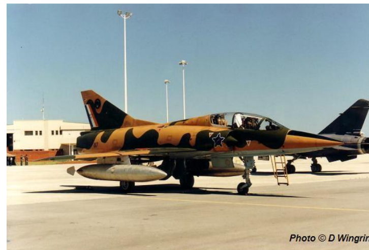
Different view of BZ #817 with two wing mounted RP62 1,300 liter fuel tanks.
