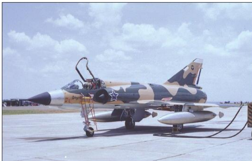
EZ #842 with two wing mounted RP62 1,300 liter subsonic fuel tanks.
