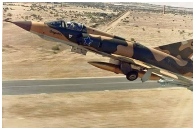
EZ with centerline RP825 fuel tank and two wing mounted V3B IR missiles.
