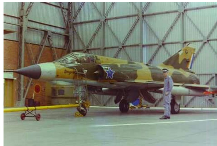
EZ #828 with two wing mounted RP62 1,300 liter subsonic fuel tanks. Red AIM-9B Sidewinder Aero 3B launch rail is fitted to the outboard wing pylon. 3 Squadron badge on vertical stabilizer
