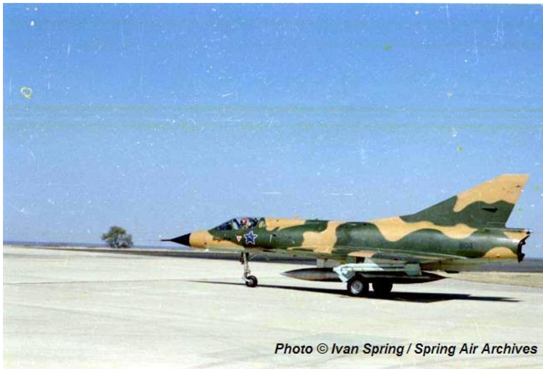
CZ #804 with single centerline RP825 supersonic fuel tank and two wing mounted V3B IR missiles. Compare #084 with #811 above : #804 is painted in the soft edge buff/green camouflage (original pattern) with the Castles on the intakes and Mirage III CZ can be seen on the forward fuselage.
