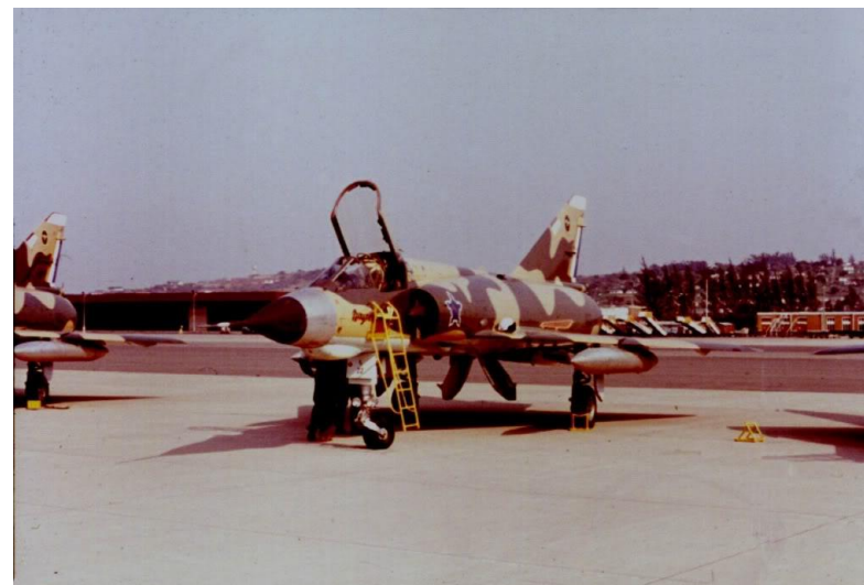
EZ #822 with two wing mounted RP18R 500 liter supersonic fuel tanks.
