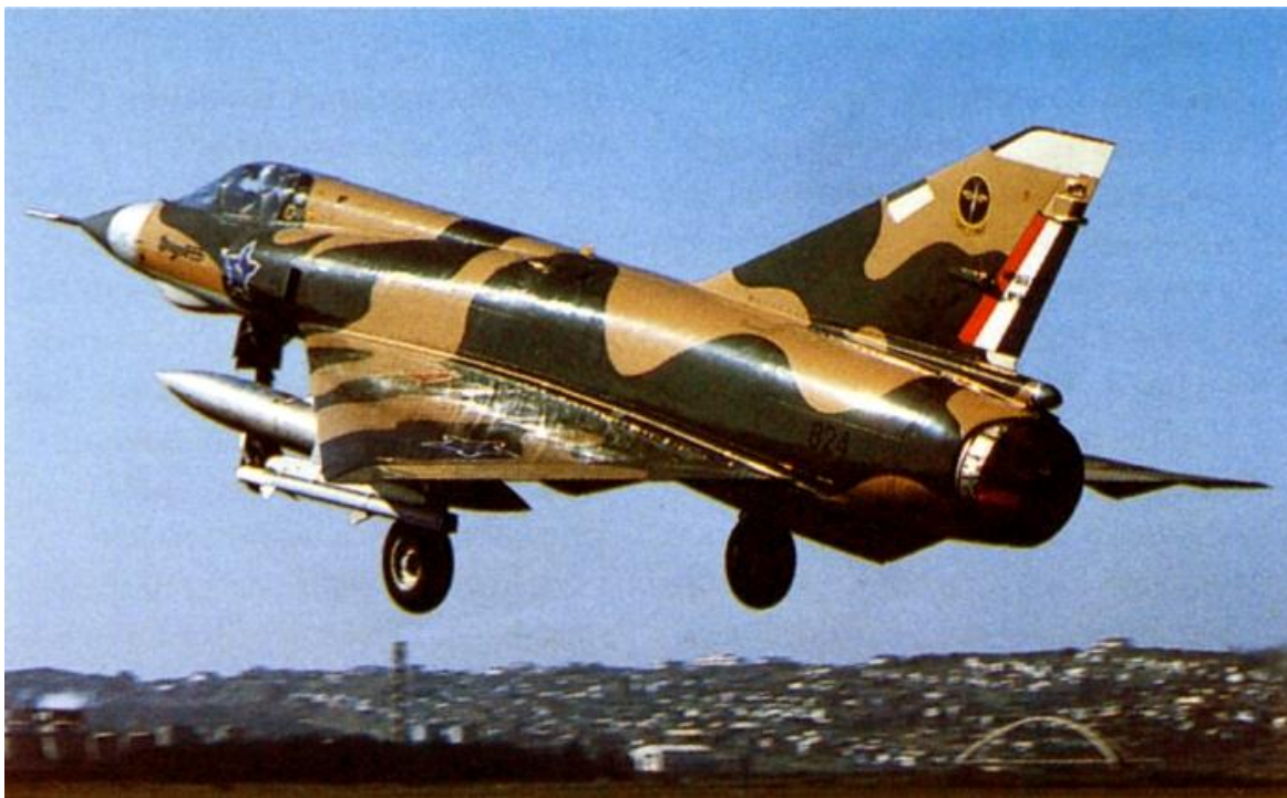
EZ #824 with two wing mounted RP18R 500 liter supersonic fuel tanks and a single AIM-9B Sidewinder missile on the port outboard wing station. The lack of rear fins leads one to deduce that this is a "captive" training item. Note the location of the Castle on the upper port wing.
