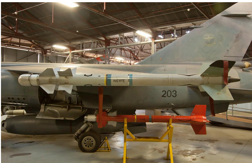
Matra R550 IR missile on Mirage F1CZ #203 at Swartkop. Note the different canard arrangement when compared to the V3A and V3B. Note also the higher aspect ratio on the rear fins as compared to the AM-9B, V3A and V3B. Overall the R550 is larger in diameter.
