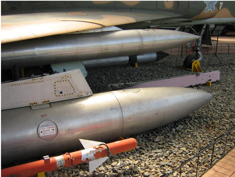
CZ #813 with (front to back) red practice V2 (AIM-9B) air-to-air missile, 1,300 liter RP62 fuel tank, 500 liter RP18R fuel tank and Matra JL-100 combined fuel tank / rocket pod. The pink coloured object is the PM-3 bomb beam for use on the centerline station.
