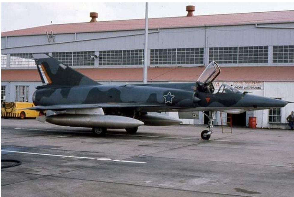
RZ with 1,300 liter RP62 wing tanks.
