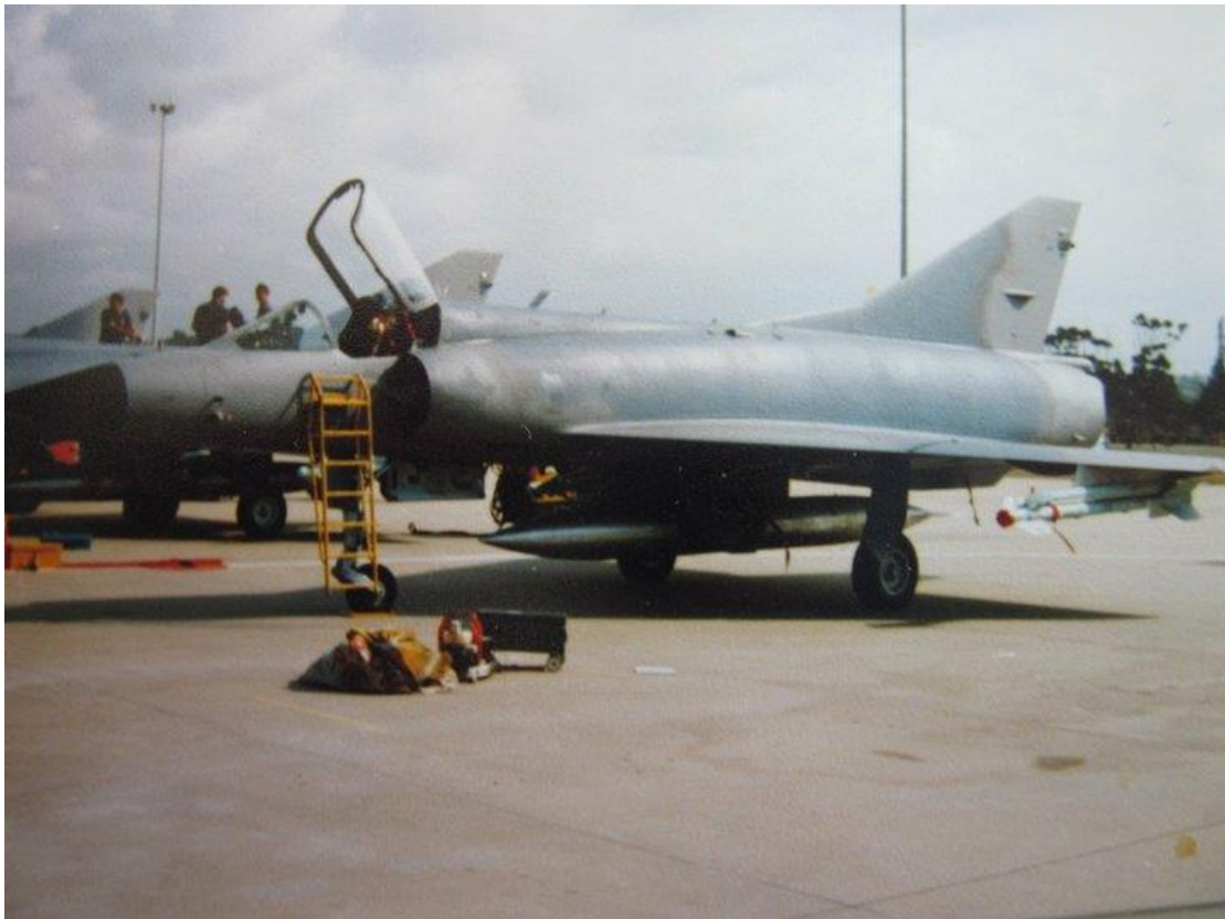
Probably CZ #807 again showing the centerline RP825 fuel tanks and wing mounted V3B missiles.
