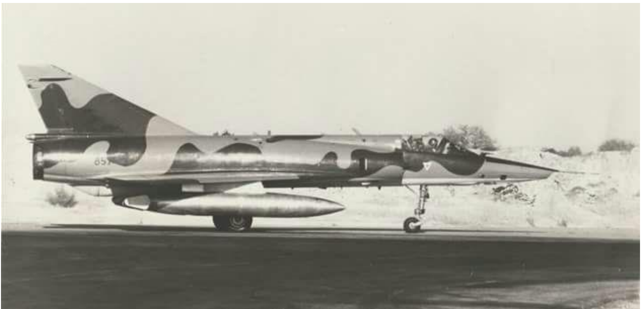
R2Z #857 with two wing mounted RP62 1,300 liter fuel tanks
