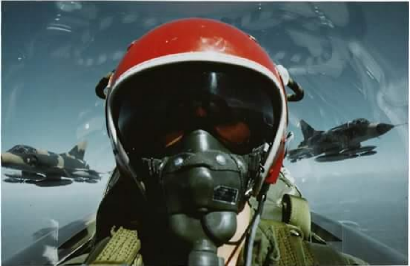
Two CZs each carrying 110G fuel tanks with tandem bombs on the wings and RP825 fuel tank on centerline. Both are painted in the soft edge buff/green camouflage (revised pattern).
