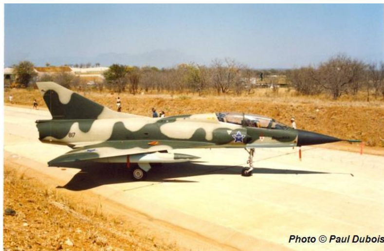
BZ #817 with two 110G fuel tanks. The tanks have been camouflaged in a similar fashion to the rest of the aircraft.
