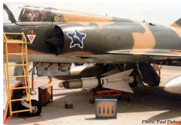
This aircraft has two wing mounted RP62 1,300 liter fuel tanks and a Matra R530 air to air missile displayed beneath the aircraft. This is actually RZ #838 going by the two digits on the nose door – the RZ would not have carried the R530.
