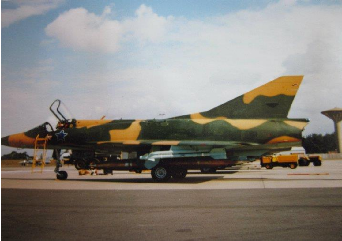
CZ #811 with single centerline RP825 supersonic fuel tank and two wing mounted V3B IR missiles. Camouflage is soft edge buff/green (revised pattern) with Castles on the intakes. Mirage III CZ is absent from the forward fuselage.
