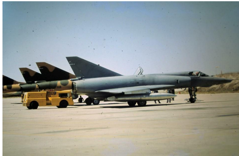
RZ #835 with two wing mounted RP62 1,300 liter subsonic fuel tank
