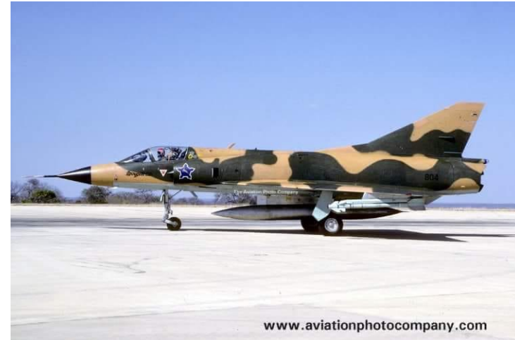
CZ #804 with single centerline RP825 supersonic fuel tank and two V3B IR air-to-air missiles on the outboard wing pylons.
