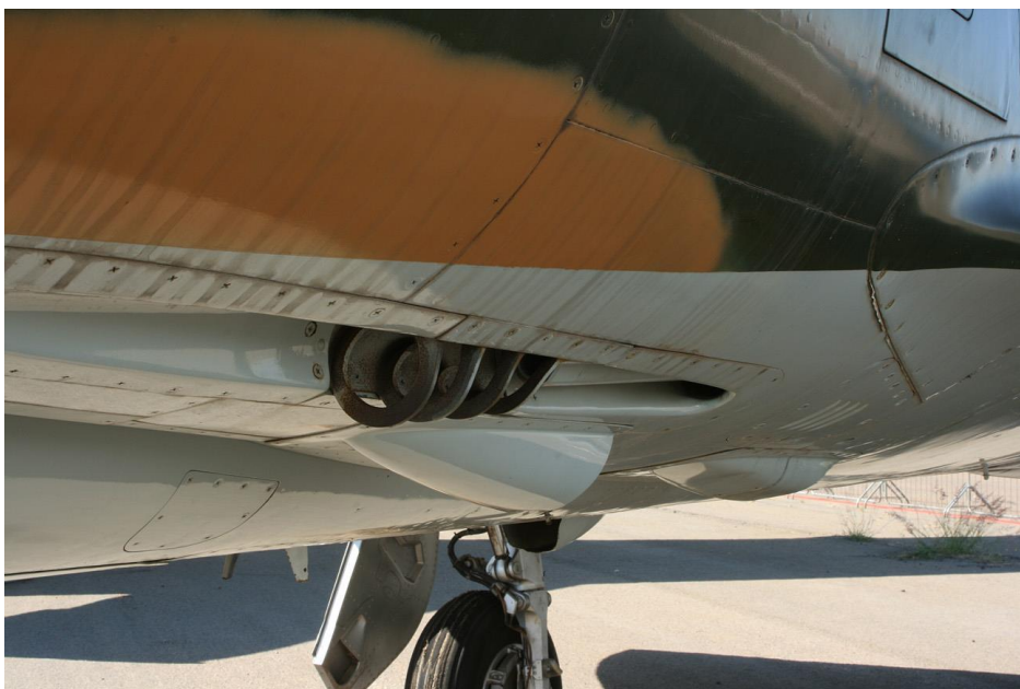
Port 30mm cannon muzzle brake on RZ #838. The canon barrel is missing.
