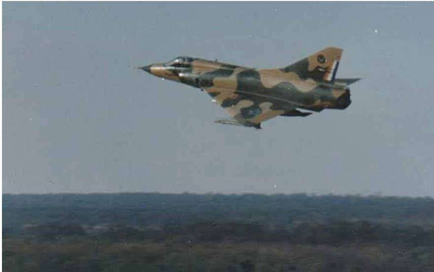
Unidentified CZ with what appears to be a captive AIM-9B round on the port outboard wing pylon (note lack of forward fins on missile). Aircraft carries an RP825 fuel tank on the centerline pylon.
