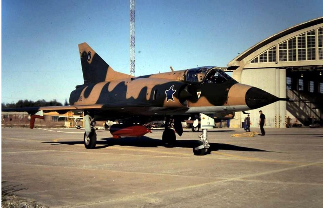
CZ #813 with towed aerial target pod mounted on the centerline and the target kite on the starboard outer wing pylon.
