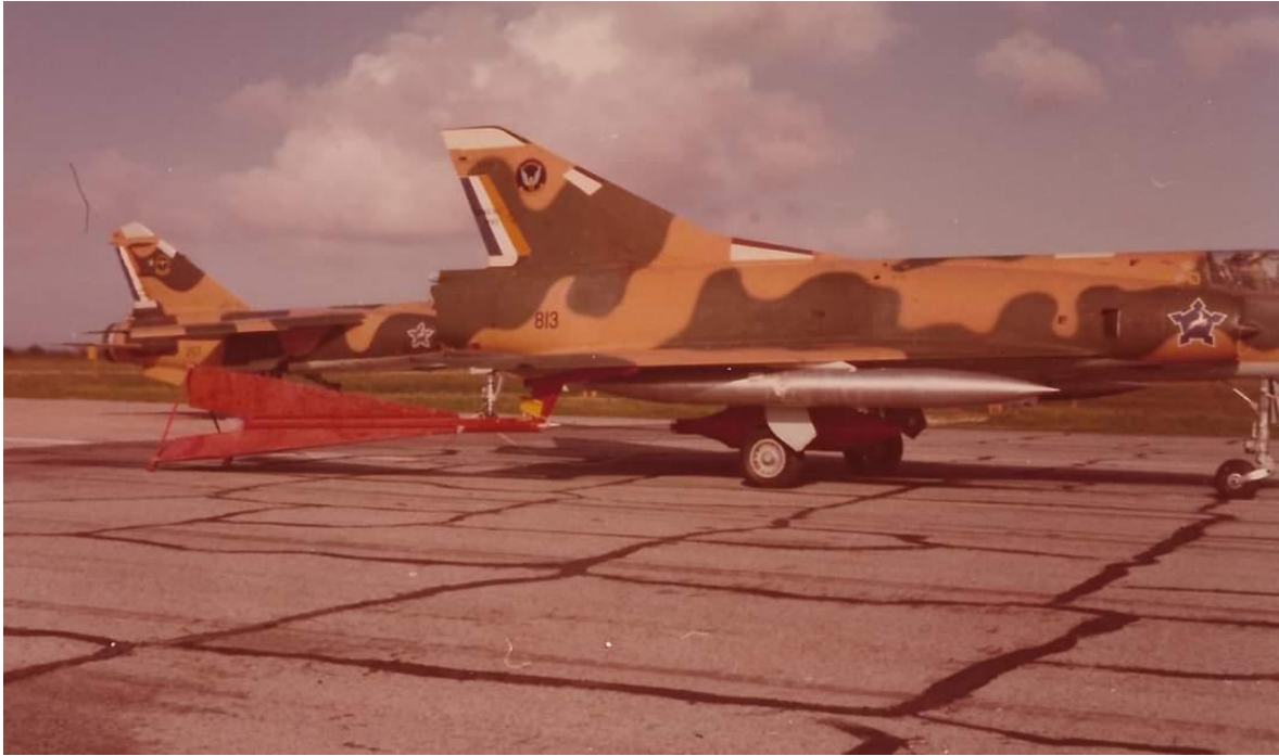
CZ #813 (above) and #810 (below) with towed aerial target including the winch pod mounted on the centerline. The target kite is mounted on the outboard wing station and tethered to the winch pod. RP18R fuel tanks are carried on the wings.
