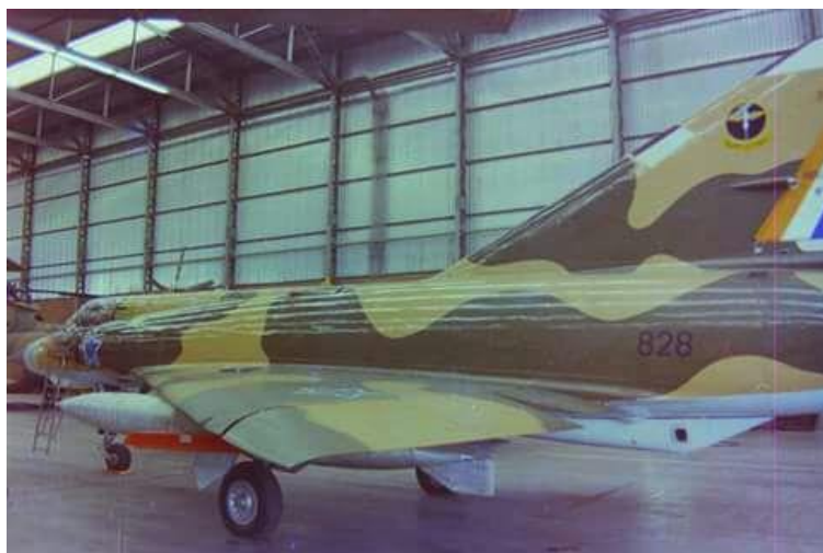
EZ #828 with two wing mounted RP62 1,300 liter subsonic fuel tanks. Red AIM-9B Sidewinder Aero 3B launch rail is fitted to the outboard wing pylon. 3 Squadron badge on vertical stabilizer
