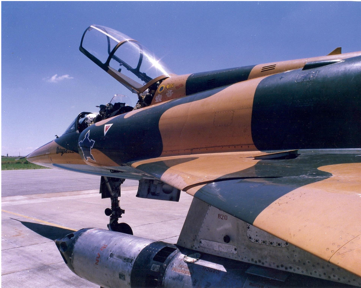
D2Z with wing mounted JL-100 combined fuel tank / rocket pod. The air brake is slightly open which was characteristic of the Mirage III with power off. This photo gives an idea of how sleek the twin seat Mirages were.
