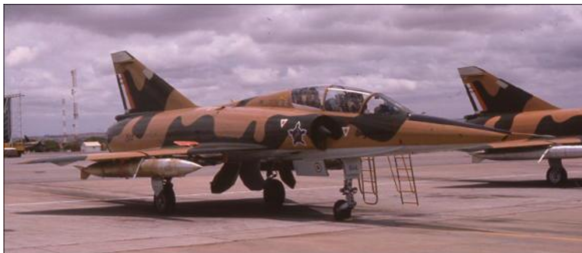
D2Z #844 with two wing mounted 110G fuel tanks. Note the weathered orange coating on the fuel tanks.
