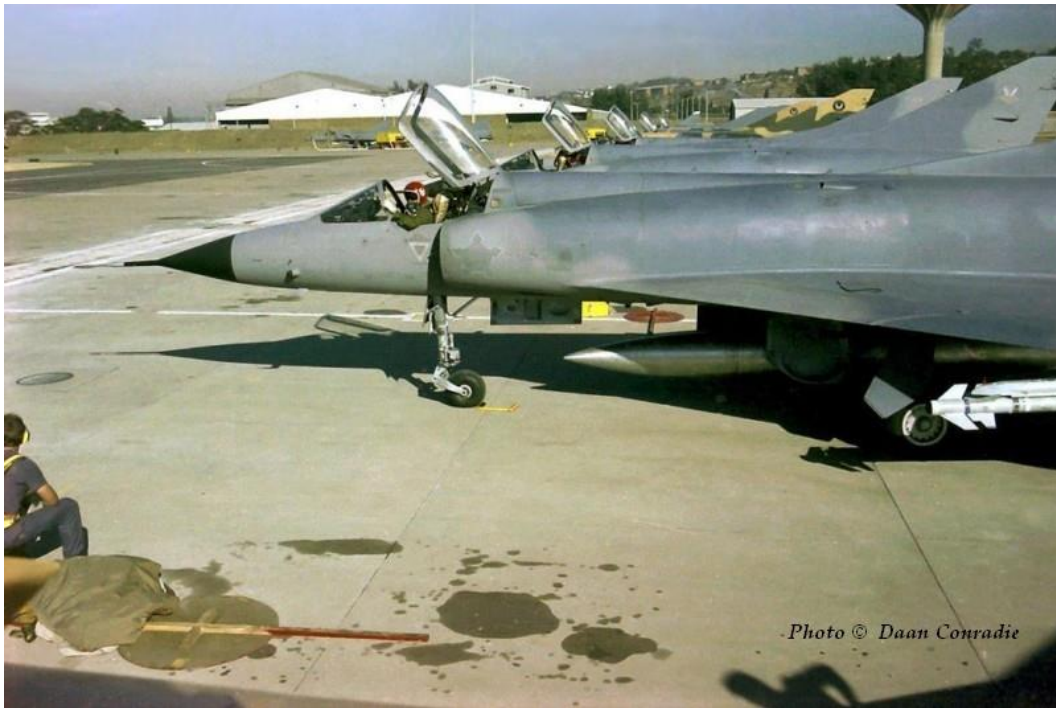
CZ with single centerline RP825 supersonic fuel tank and wing mounted V3B IR missile. Weapons Camp, Durban. Note the Cheetahs at the far end near the warehouse.
