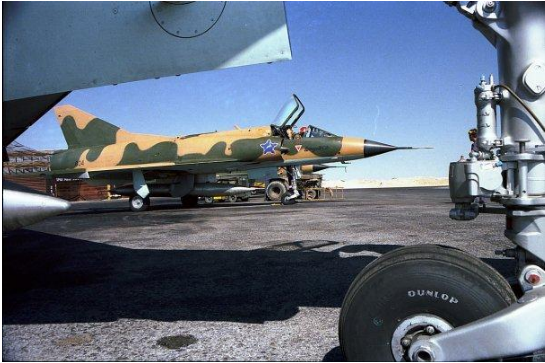
CZ #804 at Ondangwa painted in soft edge buff/green camouflage (original pattern). #804 is fitted with an PR825 fuel tank on the centerline and missile pylons on the outboard wing station.
