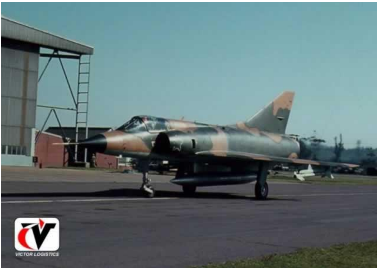
Two images of possibly the same CZ (soft edge buff/green camouflage (original pattern), radar nose with buff/grey nose cone, 2 squadron badge on the vertical stabilizer), likely seen at Durban. It would appear that the standard layout for ACM camps was a centerline RP825 fuel tank and two wingtip mounted V3B missiles.
