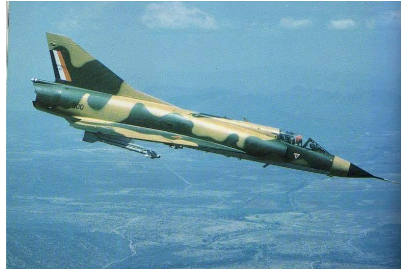
CZ #800 with V3B air-to-air missiles on the outboard wing pylons.
