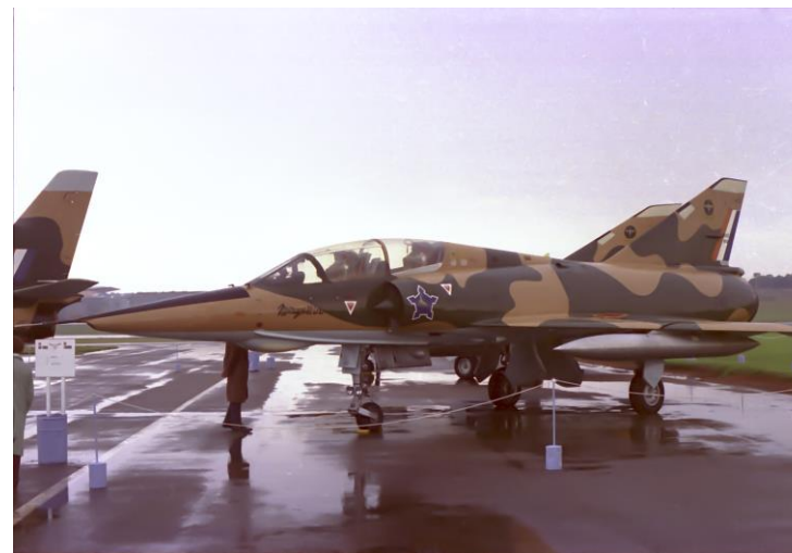
DZ #840 with two RP18R 500 liter supersonic fuel tanks as seen at Waterkloof Airshow in 1980.
