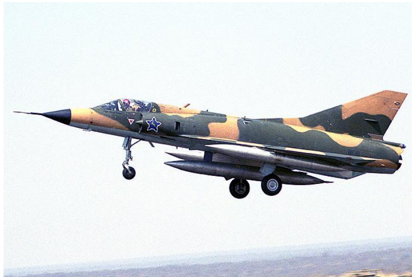
CZ #806 with centerline RP825 and two wing mounted 110G tanks.
