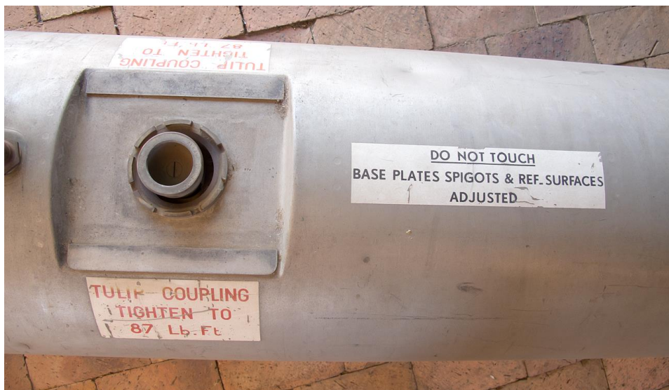
JL-100 wing pylon mounting details.
