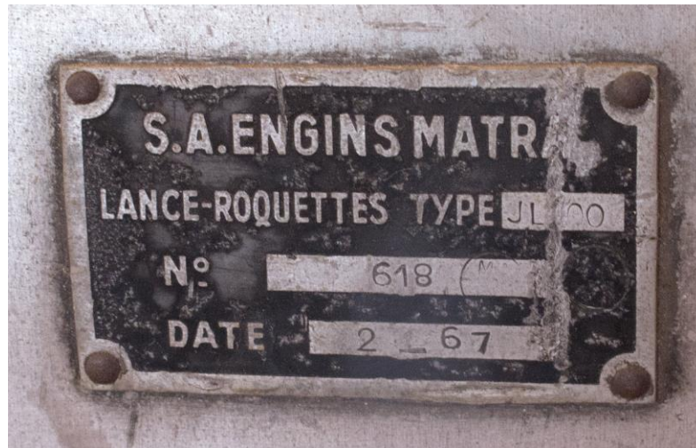
Data plate detail from the JL-100 combined fuel / rocket pod at the Johannesburg Museum of Military History. The one above is from the dark coloured rocket exhaust section (serial #180 manufactured in 1964) and the one below from the natural metal rocket pod section (serial #618 manufactured in 1967). This would indicate that the JL-100 was of modular assembly with sections being interchangeable. The data plates can be seen on the pod in the bottom image.
