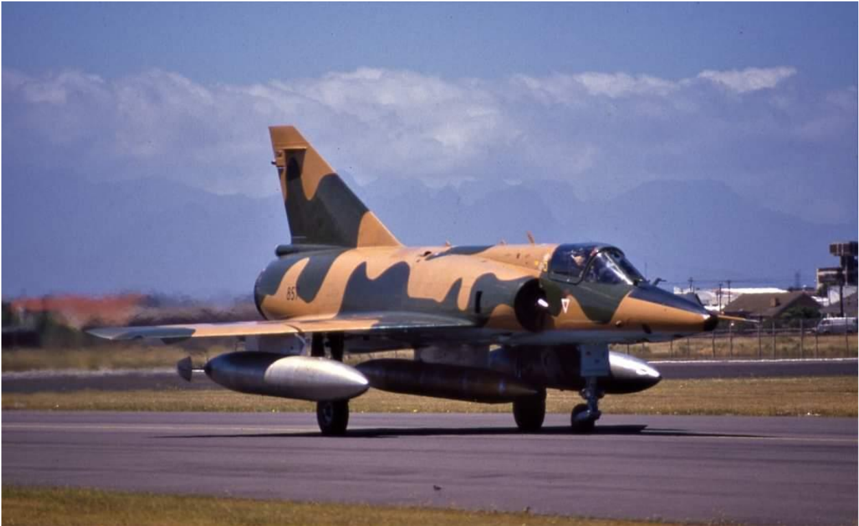
R2Z #857 carrying RP825 fuel tank on center station and two wing mounted RP62 fuel tanks.
