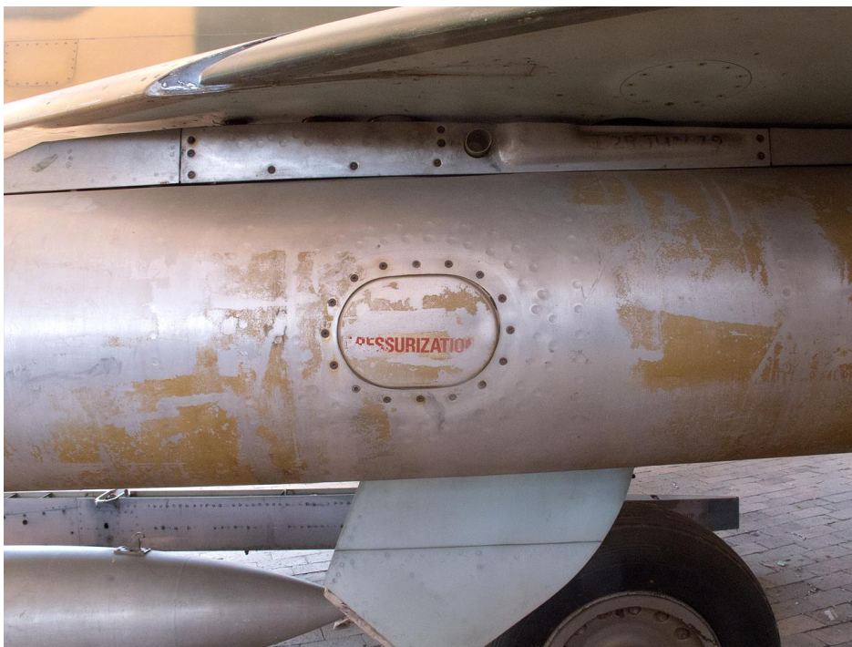
Detail of a 500 liter RP18R supersonic fuel tank mounted on CZ #813. Note the weathered orange protective coating. It appears that the tank is of combined riveted and welded construction.
