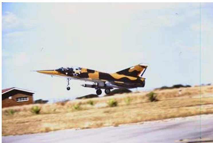
D2Z with two wing mounted JL-100 combined rocket/fuel tank pods.
