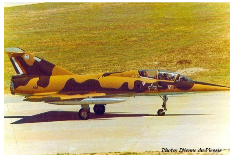
D2Z #851 with two wing mounted RP18R fuel tanks.
