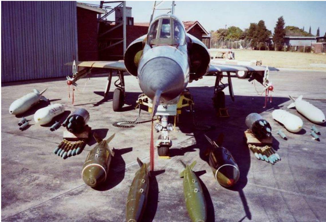
Different view of the same scene as on the previous page, now with a front view of EZ #834. The stores are, working from the center outwards, Mk.81 250lb GP bombs, 1,000lb GP bombs, the rocket section of the JL-100 combined fuel tank/rocket pod with rockets, a practice bomb dispenser (with grey practice bombs) and an unidentified store which could possibly be a napalm bomb. The author could find no images of SAAF Mirage IIIs in operation carrying with either of the latter two stores.
