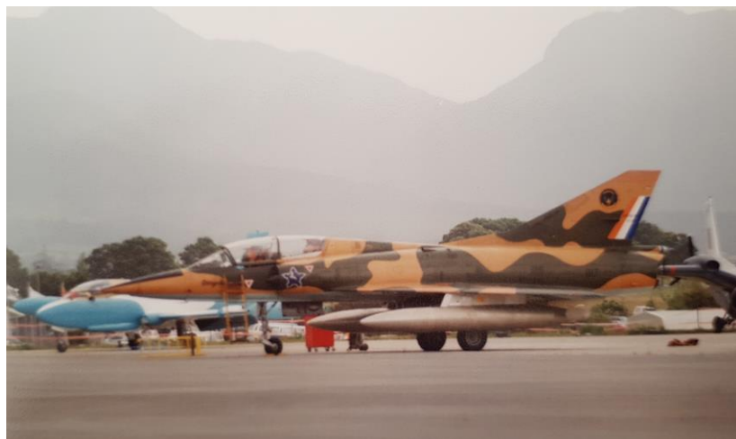
BZ #817 at Ysterplaat with two RP62 1,300 liter fuel tanks.
