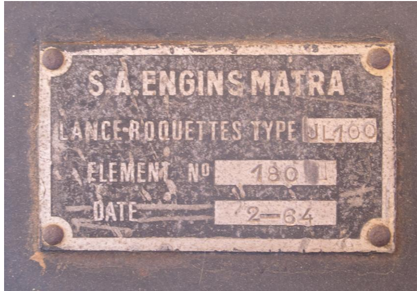
Data plate detail from the JL-100 combined fuel / rocket pod at the Johannesburg Museum of Military History. The one above is from the dark coloured rocket exhaust section (serial #180 manufactured in 1964) and the one below from the natural metal rocket pod section (serial #618 manufactured in 1967). This would indicate that the JL-100 was of modular assembly with sections being interchangeable. The data plates can be seen on the pod in the bottom image.
