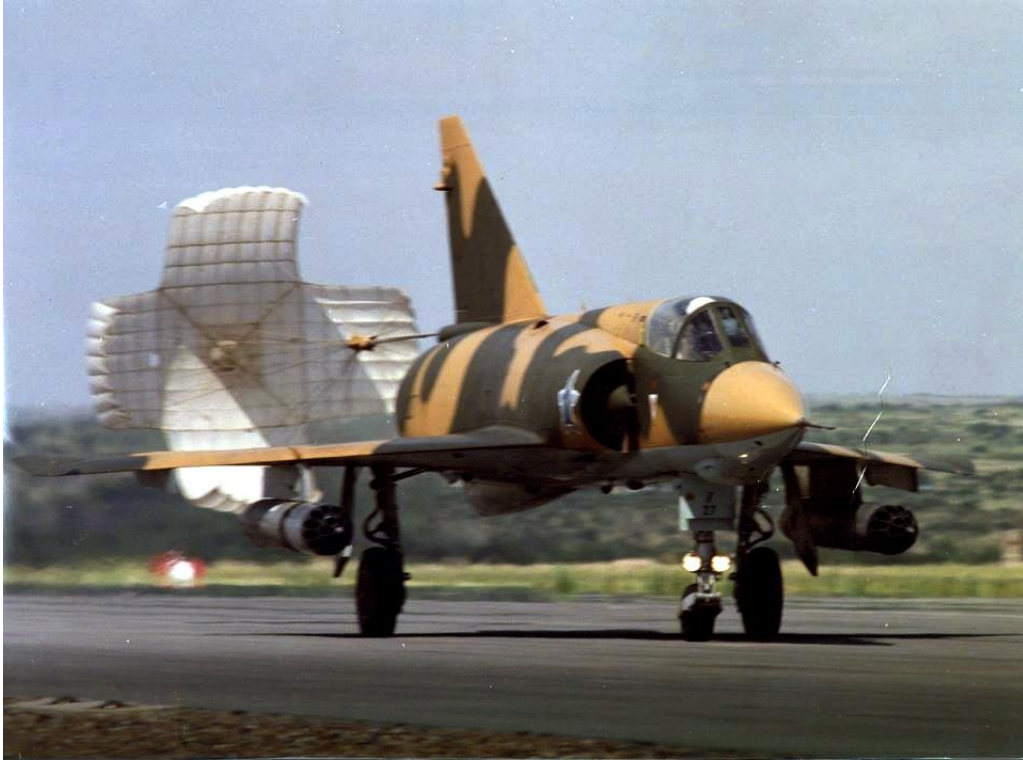
EZ #827 seen at Pietersberg AFB in 1987 painted in the soft edge buff/green camouflage. It carries two JL-100 pods.
