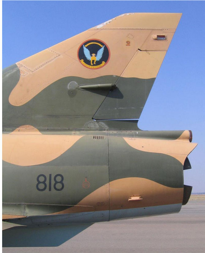
BZ #818 showing the 8" standard aircraft number as well as the 2 Squadron "Flying Cheetahs" badge.
