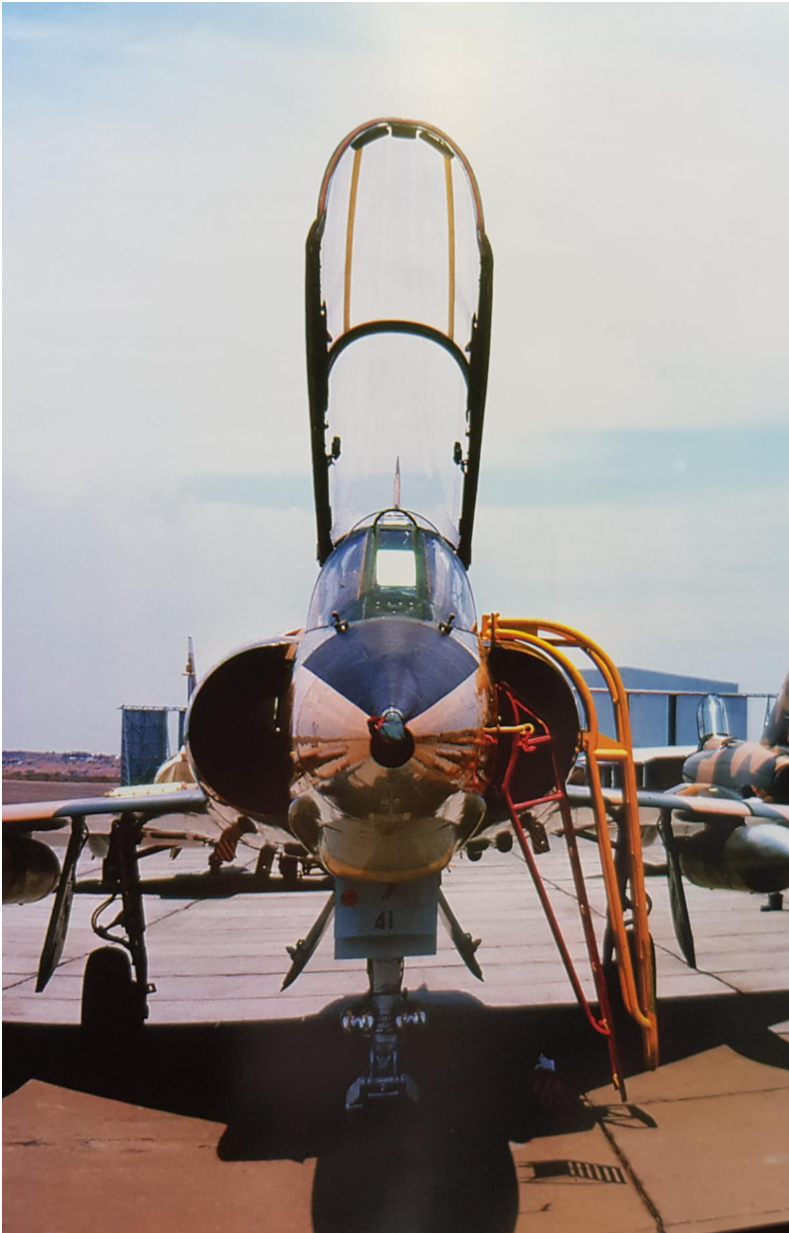
DZ #841. The doppler antenna is clearly visible beneath the nose. Note the reinforcing strips on the forward canopy section as well as the mirrors. The round air intake for avionics cooling is visible on the extreme nose beneath the pitot probe.
