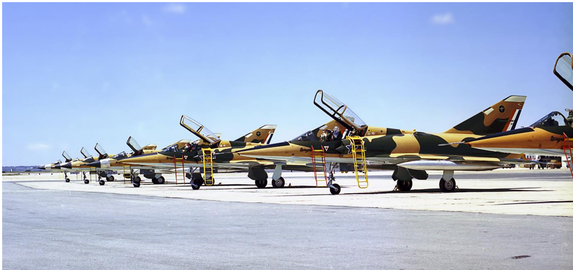
A lineup of seven Mirage IIIs. From right to left these are : D2Z, DZ, D2Z and four EZs. The D2Zs do not have the doppler antenna present. The DZ and the first EZ appear to be carrying RP18R fuel tanks. All of the aircraft are in the hard edge buff/green camouflage with full markings. Note that the entire opening section of the canopy frame of the third aircraft (D2Z) is painted buff and does not match the surrounding camouflage. Three of the EZ have unpainted nose cones and one has a buff/light blue nose cone. 3 Squadron badges are present on the vertical stabilizers.
