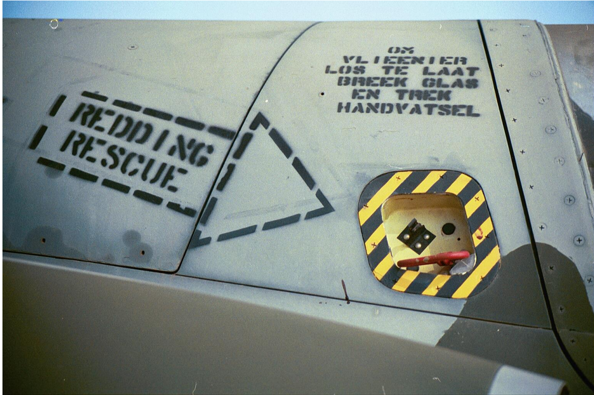
RZ #835 showing details of canopy emergency release handle markings. The window has been broken and the red handle lies in a horizontal position. It would normally be stowed in the vertical using the square black clip to retain it in position as shown in the following image.
