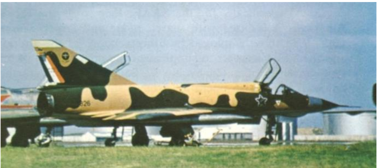
EZ #826 in gloss hard edge camouflage with natural metal nosecone. 826 has the 3 Squadron badge on the vertical stabilizer The two seater behind the EZ is a BZ as can be identified by the forward fillet to the vertical stabilizer.
