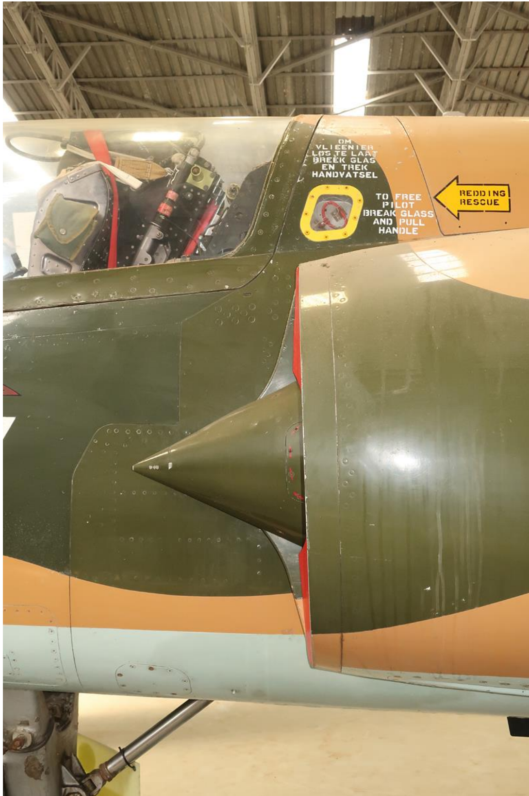
R2Z #857 showing details of markings and text associated with the canopy emergency release handles.
