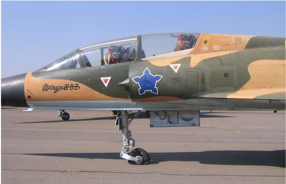
Port side of BZ #818 showing front and rear ejection warning triangles. The stylized canopy appears in red above both warning triangles. There is a yellow surround to the canopy emergency release handle window aft of the canopy.
