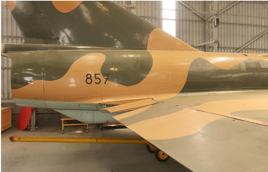
RZ #857 showing no “no step” markings on the elevons or pitch control surfaces.
