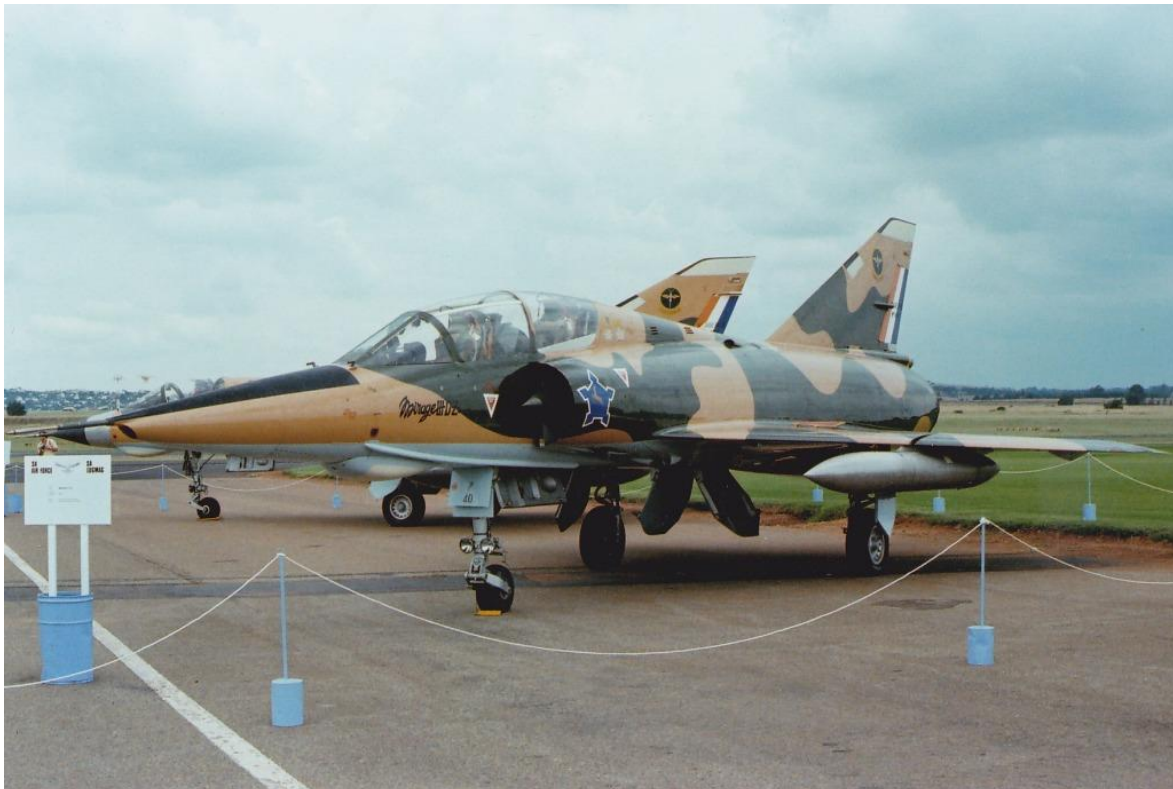
DZ #840 in hard edge gloss camouflage with full complement of markings and black anti-glare panel on the nose. Note the 3 Squadron badge on the vertical stabilizer. RP18R 500 liter fuel tanks are installed. Note the chisel shaped nose with an intake for avionics cooling at the tip. The aircraft in the background is an EZ.
