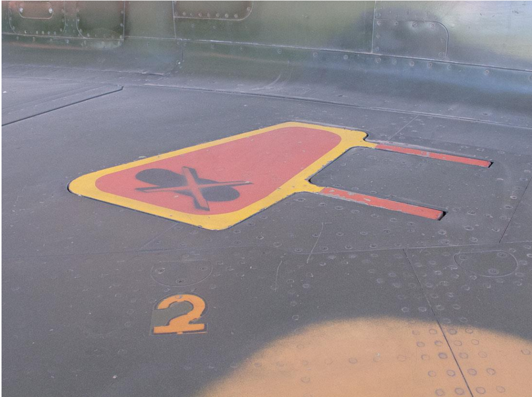
CZ #813 showing red/yellow airbrake with boot and cross marking. The coat hanger shaped symbol is to designate the aircraft wing hoisting hard point which is located behind the semi-spherical access hatch.
