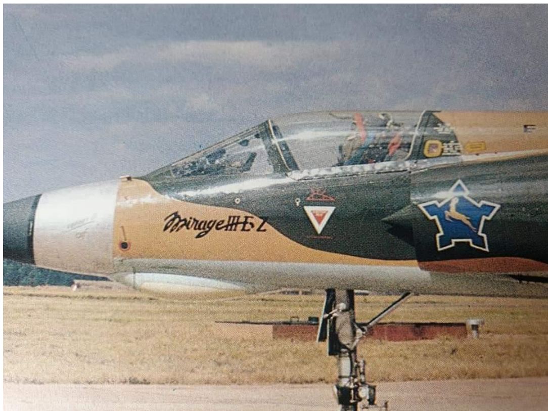
Unidentified EZ showing marking details on forward fuselage including “Cyrano II CSF” on unpainted natural metal nose cone. The red surrounded black circle above the doppler antennae is the tube used to locate the ground recovery tow bar.
