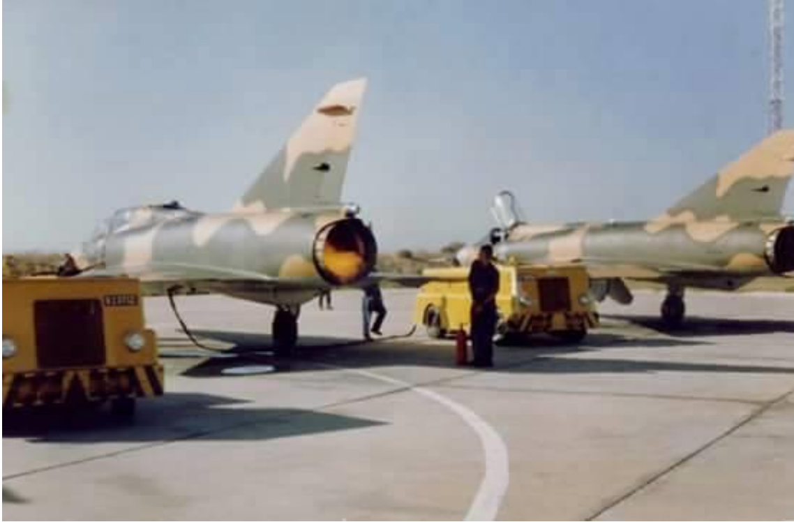
The aircraft on the left is a D2Z (note antennae on upper vertical stabilizer which distinguishes this from the DZ) with an EZ to its right. Both aircraft are in soft edge matt camouflage with what appears to be a total lack of markings.
