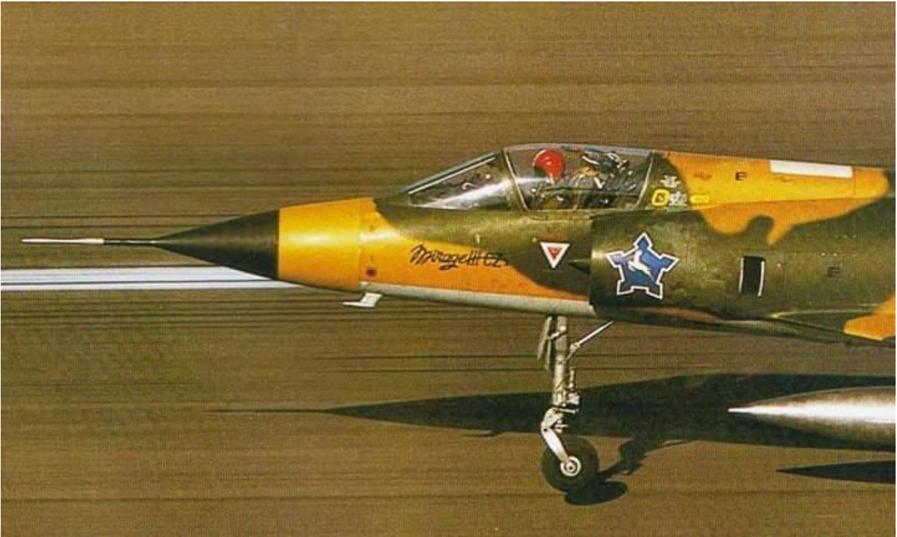
Unidentified CZ showing forward fuselage markings including the standard NATO symbols on the avionics bay panel aft of the cockpit. The canopy emergency release handle window aft of the canopy is surrounded in solid yellow edging.
