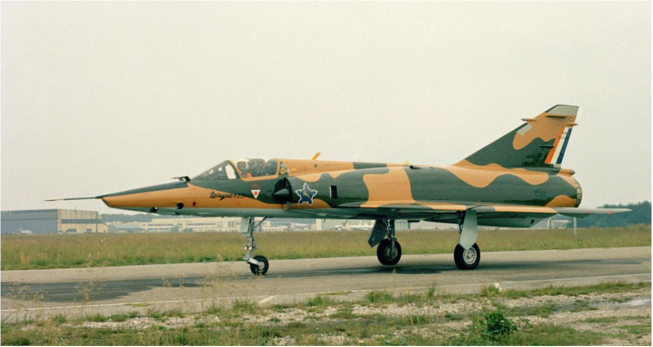
R2Z #856 in early delivery gloss hard edge camouflage scheme. 2 Squadron badge has not been applied to the vertical stabilizer. The entire canopy frame is painted in buff. Note the original French factory mounted RWR antennae on the leading and trailing edges of the vertical stabilizer. This was unique to the R2Z as the only SAAF Mirage III variant so equipped.
