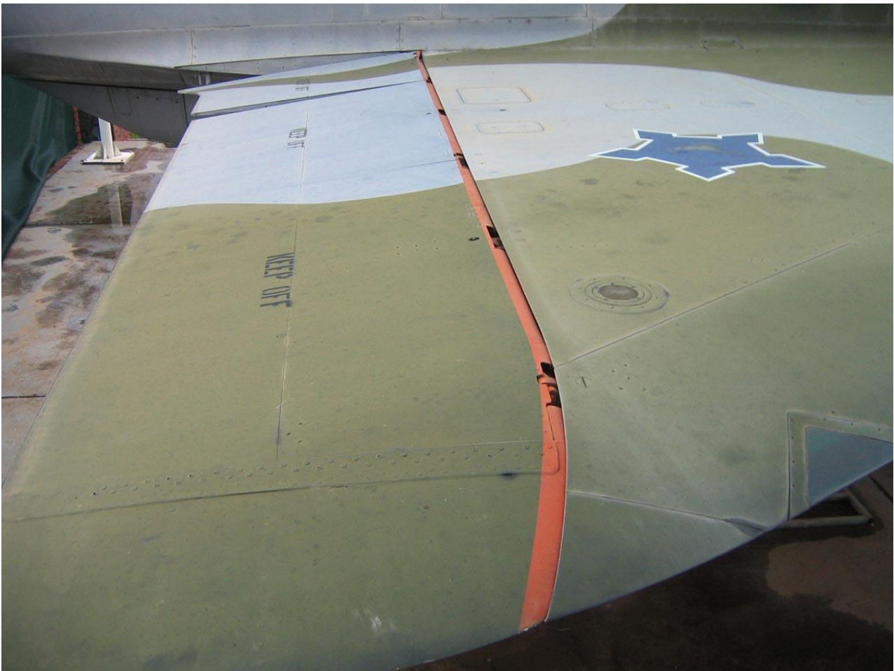
RZ #835 showing “KEEP OFF” markings on all three control surfaces on starboard wing. Note that the red stripe is painted on the elevon leading edge and not the wing surface.
