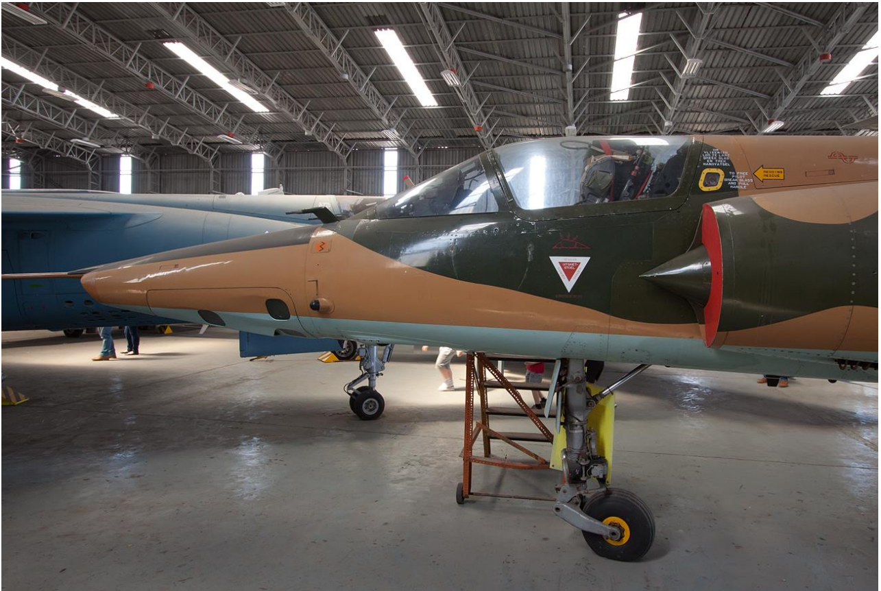
R2Z #857 showing port forward fuselage marking details. Note absence of Castles. Typical warning and maintenance symbols and text are present aft of the cockpit as is the yellow surround to the canopy emergency release handle window.
