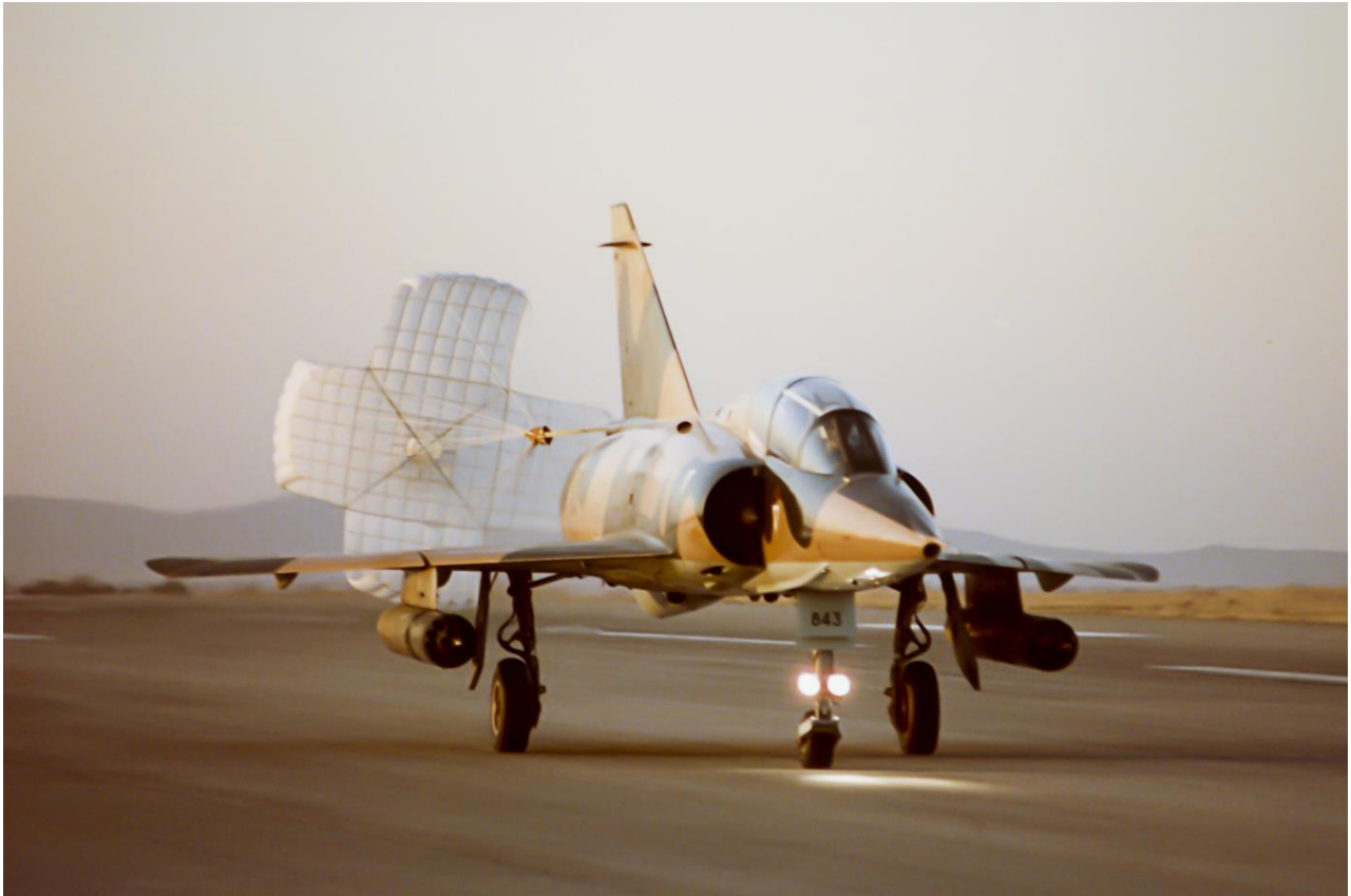
D2Z #843 landing at Pietersberg AFB, 1984. The three digits "843" appear on the nose door whereas this would usually be limited to the last two digits of the aircraft number. #843 is carrying JL-100 pods.
