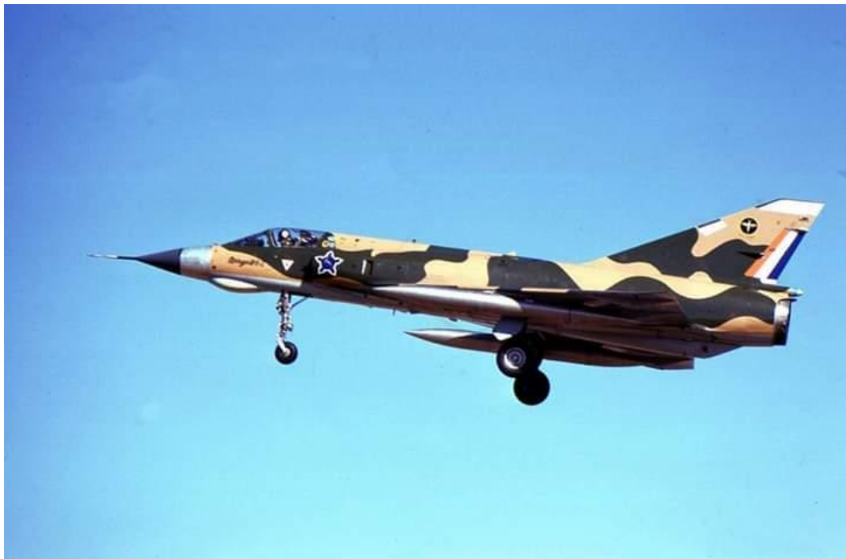
Another image of an EZ in hard edge buff/green camouflage with natural metal nose cone and full markings including the 3 Squadron badge on the vertical stabilizer. The wing fuel tanks are 500 liter RP18R.
