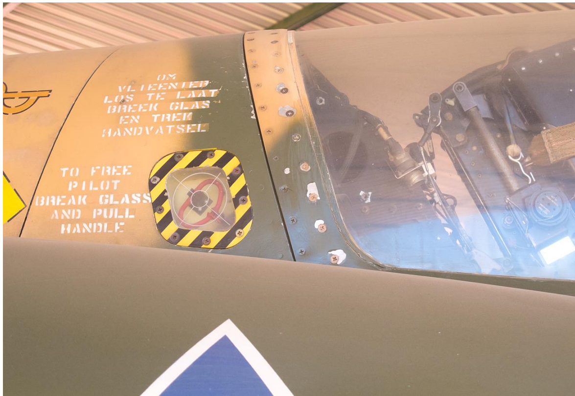
CZ #813 showing details of canopy emergency release handle markings. Note mismatched camouflage between canopy frame and fuselage.
