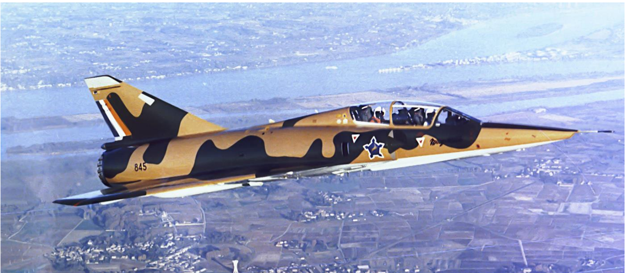
Two images of D2Z #845 in the gloss hard edge camouflage (original pattern) with full markings except for the squadron badge on the vertical stabilizer. The entire opening section of the canopy frame is painted buff. Note that the text "Mirage IIID2Z No. 8xx" is applied on the top portion of the rudder.
