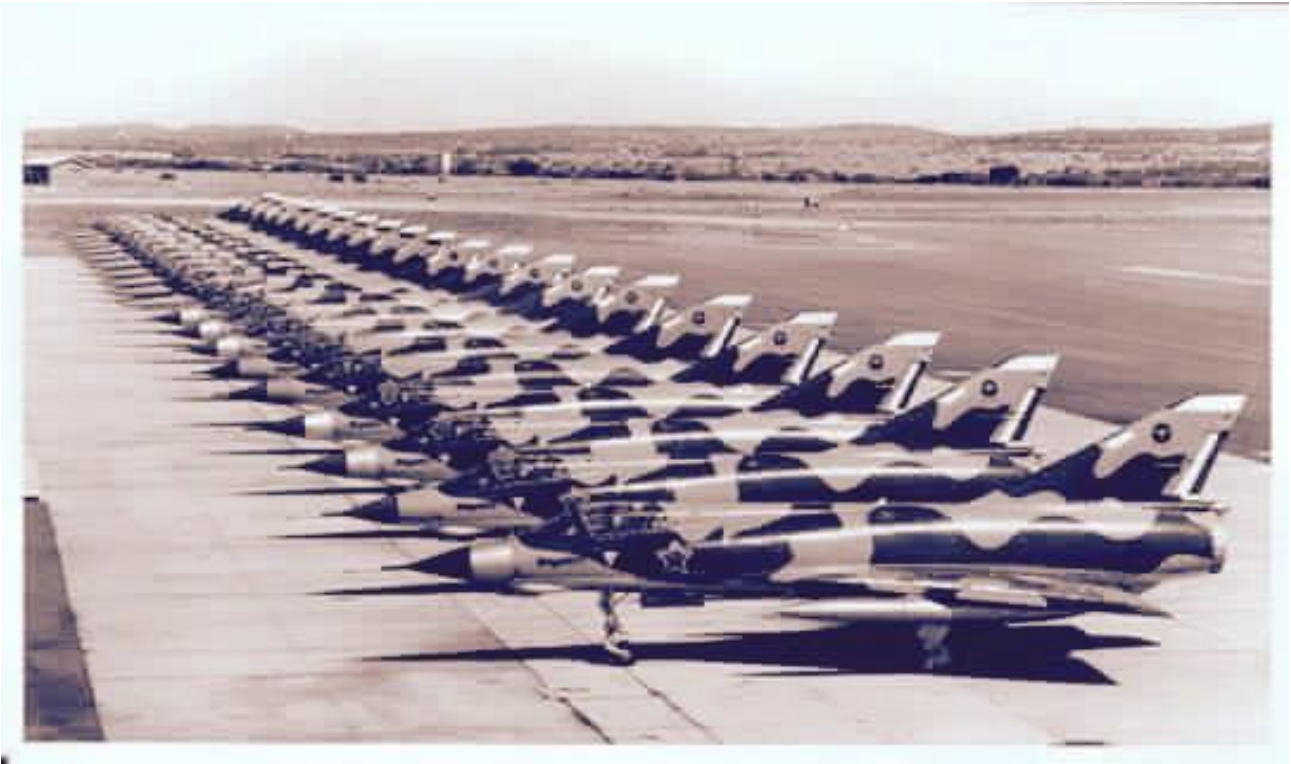
A line up of nine EZs resplendent in their new gloss hard edge buff/green camouflage. Note that six of the EZs appear to have the unpainted natural metal nose cone. The remaining aircraft are likely to be DZ or D2Zs based on the slimmer nose profiles. Note the 2 Squadron "Wasp" badge on the vertical stabilizers of the EZs. The EZ in the foreground has 500 liter RP18R wing tanks installed.
