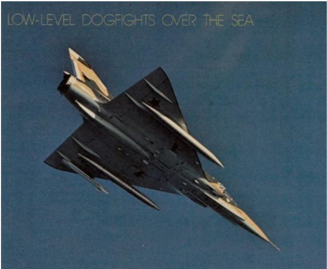
Underside photo of D2Z carrying two RP18R fuel tanks and a single AIM-9B captive round. Note the position of the Castle on the underside of the wing. It is located between the two aerodynamic fairings which cover the elevon actuators and just forward of the elevon. This location would be similar for all SAAF Mirage IIIs when carrying the Castles.
