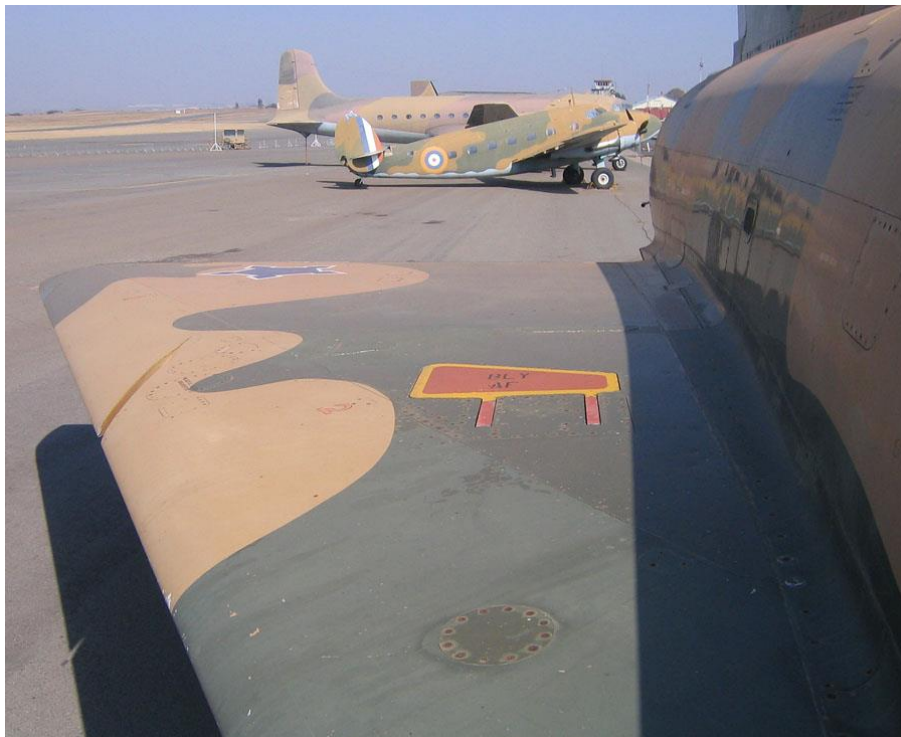
BZ #818 showing red / yellow airbrake with “BLY AF” (Keep off) stenciling.
