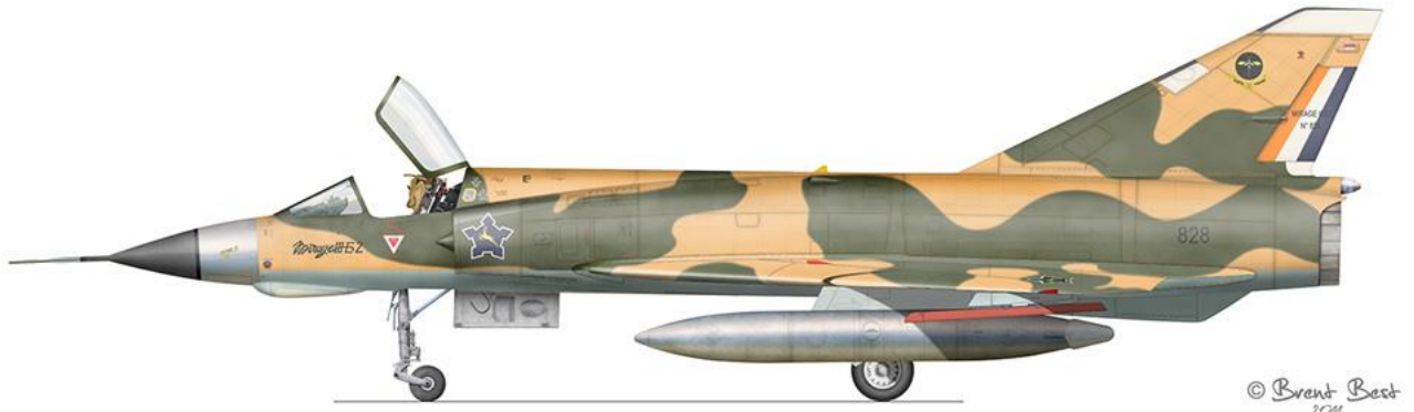
EZ #828 depicted in hard edge buff/green camouflage with full markings. 2 Squadron badge has been replaced by 3 Squadron Badge (Wasp) and the text on the rudder simplified to dispense with the "AVIONS M'DASSAULT" text, with only "MIRAGE III EZ No. 8xx" remaining. #828 is depicted with 1,300 liter RP62 wing tanks and air-to-air missile launch rails painted in red.
