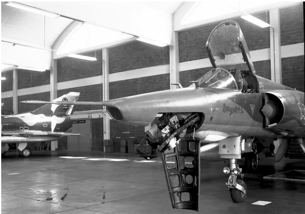
RZ painted in the NATO grey/green/silver camouflage with the nose bay door open and the camera palette in the lowered position.
