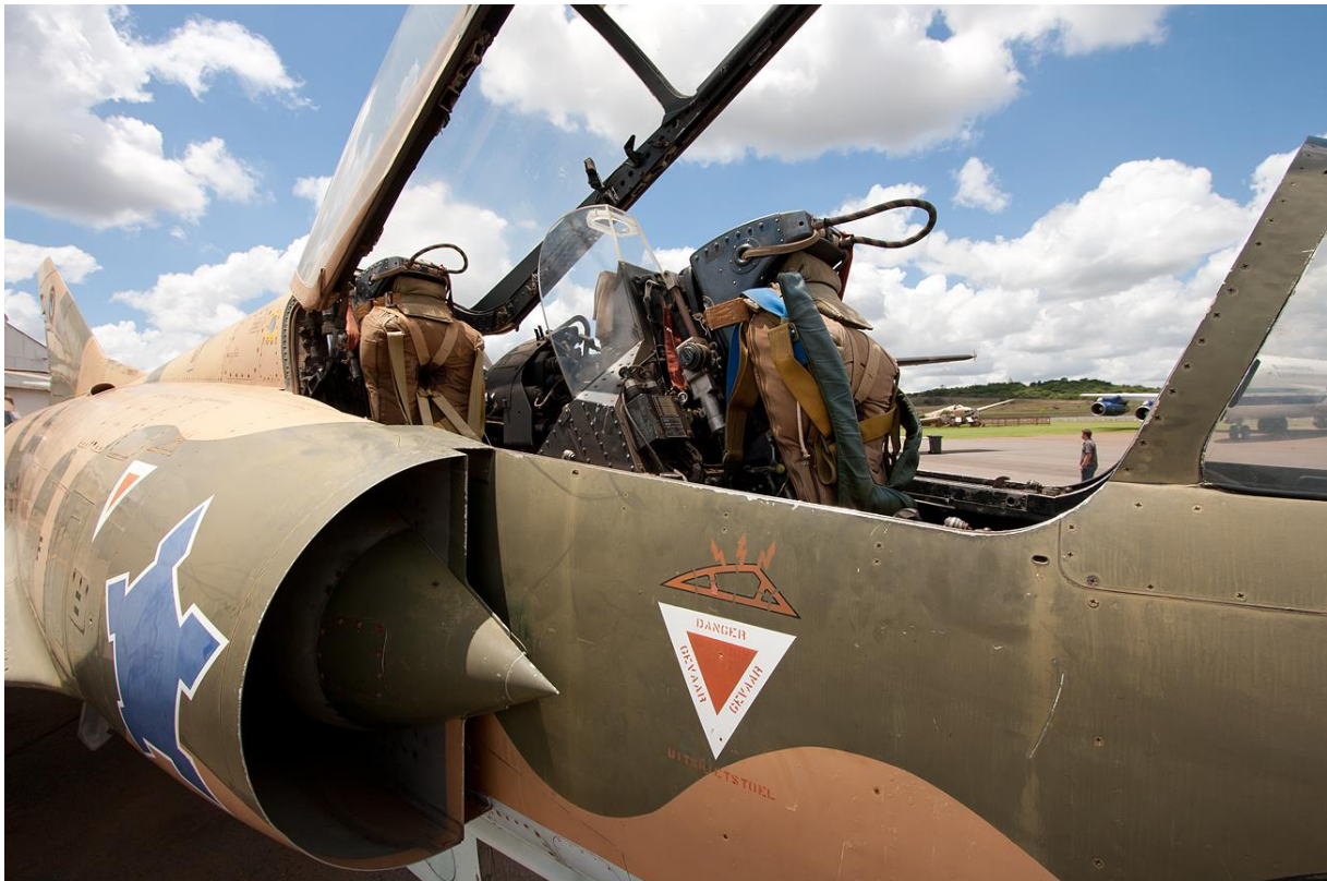
Starboard side of BZ #818. The transparent object is the blast shield which would prevent injury to the rear occupant in the case of ejection or damage to the front canopy in flight. Note how the camouflage colours wrap into the leading edges of the intakes and boundary layer splitter plate. Cockpit interior is all black as is the case for all SAAF Mirage IIIs.
