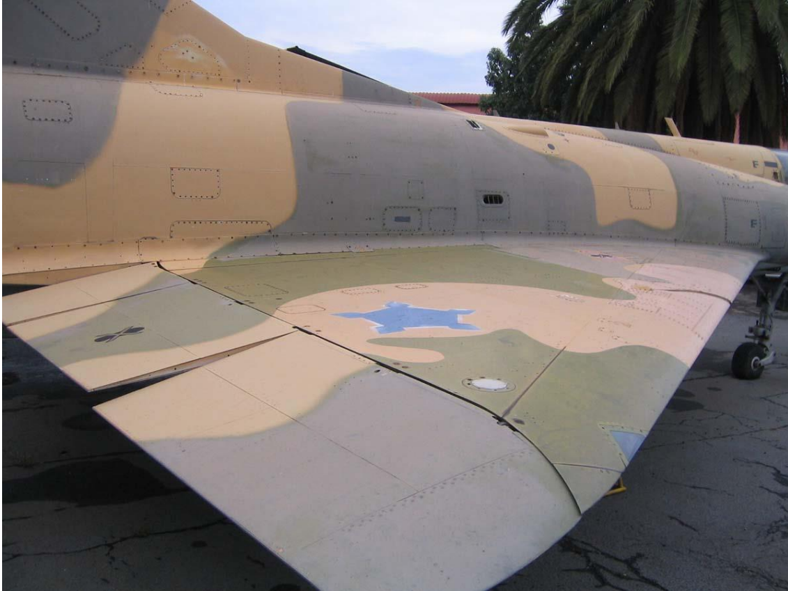
CZ #805 showing single boot and cross in black on inboard elevon only. There appears to be a similar marking on the air brake. The air brake is painted red with yellow trim. The round object near the wing tip is a blue formation light.
