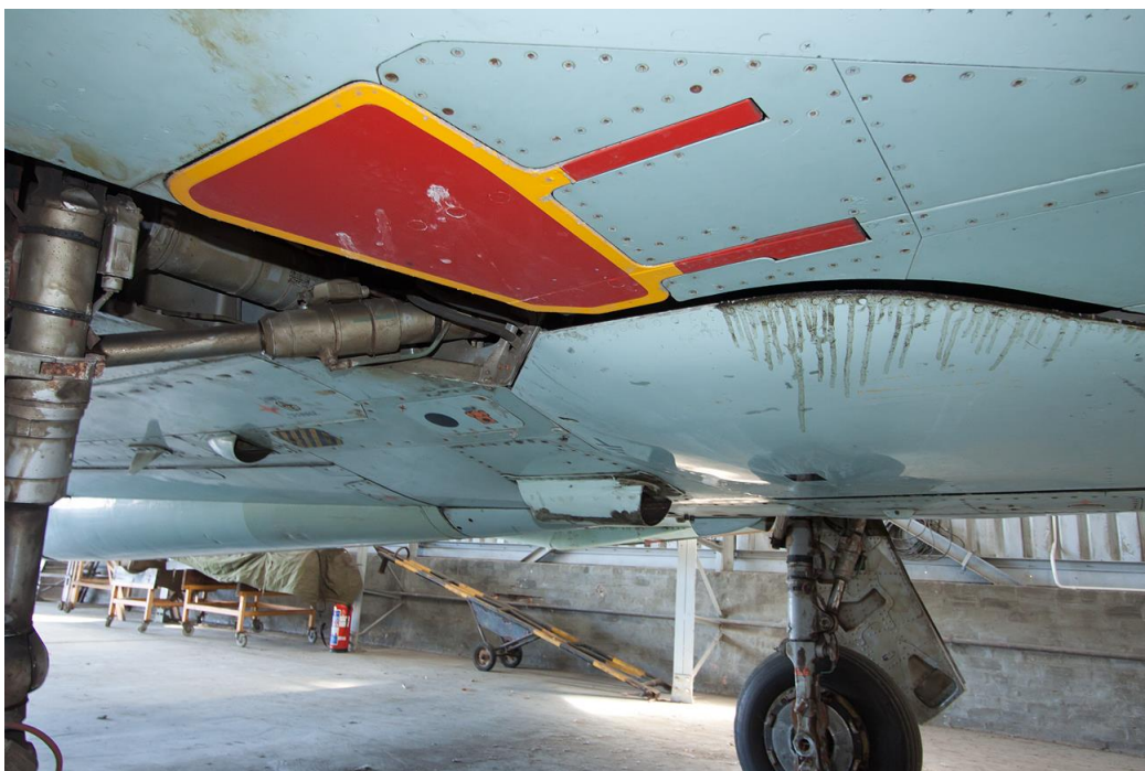
RZ #857 showing red/yellow airbrake on underside of starboard wing.
