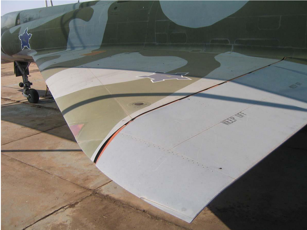
RZ #835 showing "KEEP OFF" markings on all three control surfaces on port wing.
