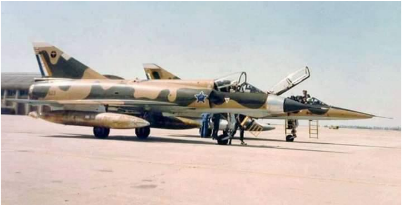
EZ #823 in hard edge buff/green camouflage with natural metal nose cone and full markings including the 3 Squadron badge on the vertical stabilizer. The wing fuel tanks are 1,300 liter RP62. Note the weathered protective orange coating on the tanks. The aircraft behind #823 is a two seat D2Z. The D2Z does not have the doppler antenna under the forward fuselage, as was the case for the DZ.
