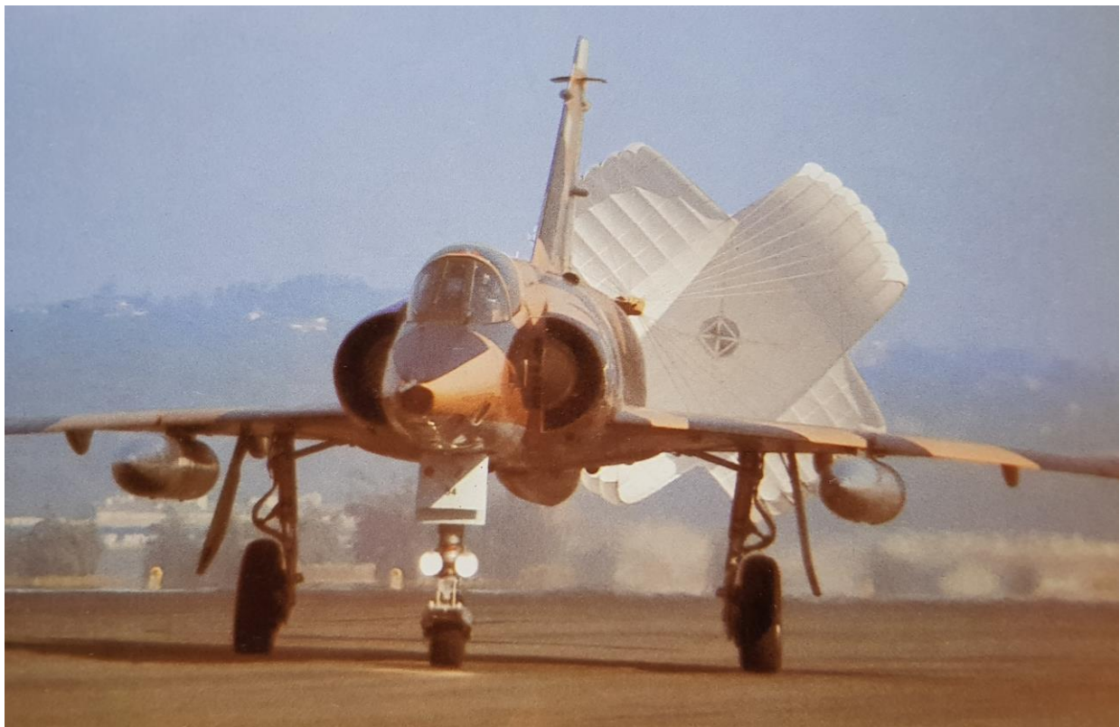
R2Z #854 trailing its drag chute. Two RP18R 500 liter tanks are on the wings. The canopy frame is painted in buff.
