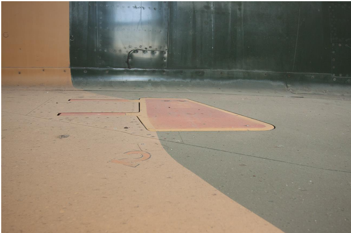
R2Z #857 showing plain red/yellow airbrakes with no "no step" markings.
