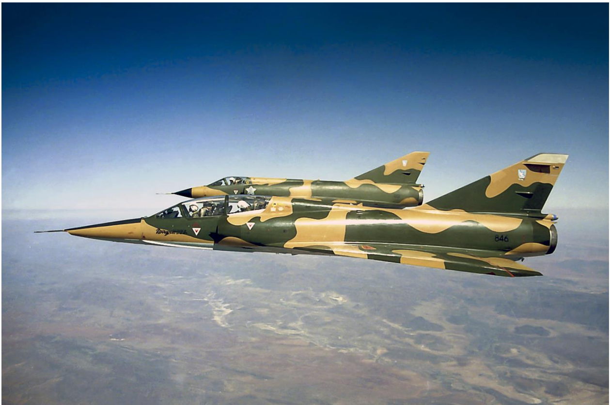
D2Z #846 in company with an EZ #819 in 1984 operating out of Pietersberg Air Base. Both aircraft have the 85 CFS squadron badge on the vertical stabilizer. They are devoid of Castles but all other markings appear to be standard. Note that the conformal antenna on the leading edge of the vertical stabilizer has been painted over but the one on the top remains in original white / light grey. Note the darker hue of the green on the intakes and the exhaust area in comparison to the adjacent fuselage areas.
