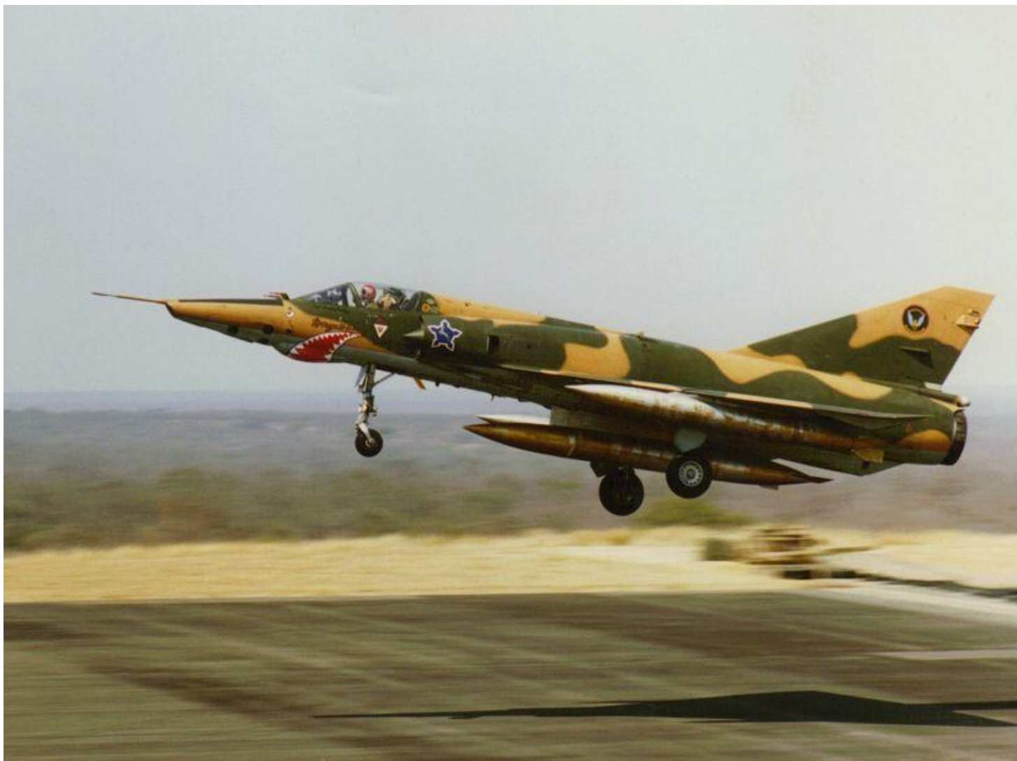
RZ #838 with teeth and eyes applied. Camouflage is the soft edge matt scheme. #838 has the centerline RP825 and two wing mounted 110G tanks installed - note the fins on the wing tanks and the heavily weathered orange protective coating the fuel tanks.
