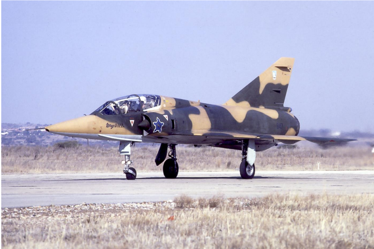
Two images of D2Z #847 in soft edge matt camouflage (original pattern) seen at Pietersburg in 1984. Note that opening section of canopy frame has been painted to match the fuselage camouflage. The antennae on the vertical stabilizer have been painted over. #847 carries the fuselage Castles and it is therefore possible that these were also applied to the wings. The 85CFS badge has been applied to the vertical stabilizer.
