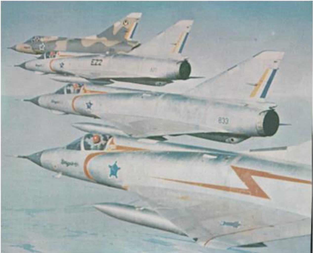
Two natural metal EZs (#820 / EZ2 and #833) displaying various combinations of markings as noted above. Both have the red trim behind the cockpit and on the intakes but do not have the red fuselage lightning bolts which were added later. The camouflaged aircraft and the aircraft in the foreground are CZs, which are identified by the fillet extension to the leading edge of the vertical stabilizer. Note that, on EZ #833, the red trim line can be seen ahead of the elevon hinge line.
