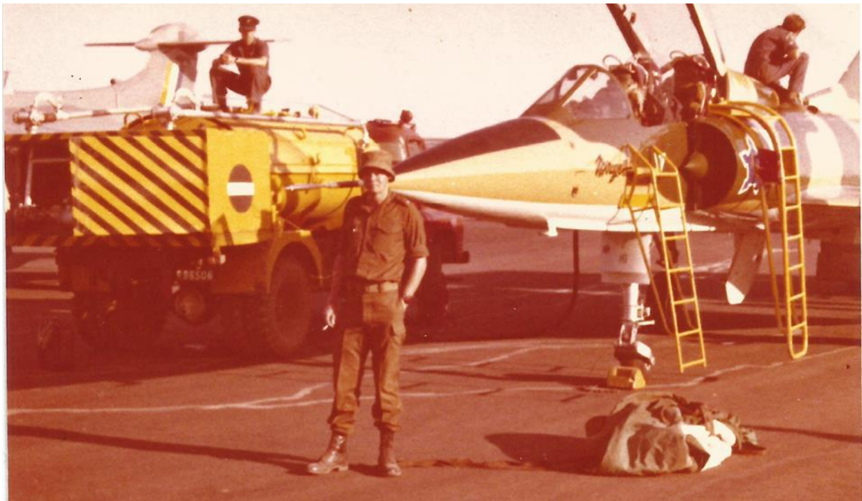
Two images of BZ #816 in the hard edge gloss buff/green camouflage scheme with black anti-glare panel on top of the nose. Note that "AVIONS M'DASSAULT" no longer appears on the rudder in the image above - only "MIRAGE III BZ N° 816" remains. Note the original white/light grey conformal dielectric panels on the vertical stabilizer.
