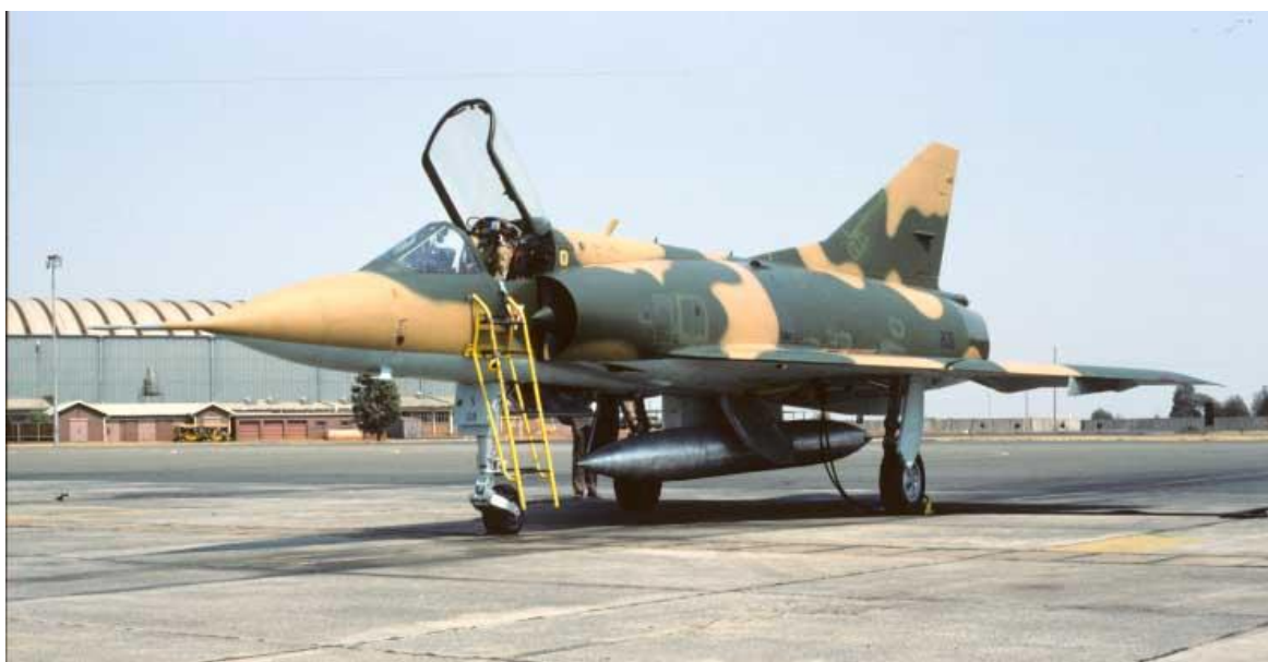
An anonymous looking CZ with a painted ballast nose cone. Note that the upper / lower camouflage demarcation is followed through to the tip of the nose. The rear portion of the pitot probe is also painted in buff.
