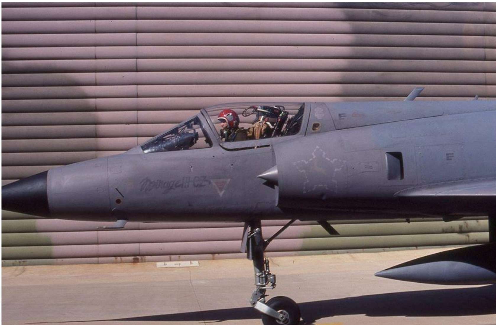
This image of an unidentified CZ demonstrates some nice marking details : low visibility Castle with dashed outline; subdued (oversprayed) stenciling, "Mirage III CZ" and ejection seat warning triangle. The aircraft is taxiing with the auxiliary intake blow-in door open. An RP825 fuel tank is located on the centerline. Interesting to note that this fuel tank has been painted in a low visibility blue/grey. The CRWS has not been fitted to this CZ as there is no round antenna on the forward fuselage. The round object just aft of the nose cone is the hole for the emergency towing / lifting tube.
