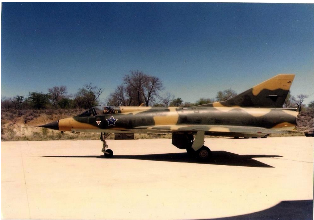
Anonymous CZ in soft edge buff/green camouflage (revised pattern). The revised pattern has the dark green covering the forward part of the vertical stabilizer strake. This area is buff on the original pattern as can be seen in the first image on this page. The green on the revised pattern wraps around onto the starboard fuselage as can be seen in the first image on the following page.
