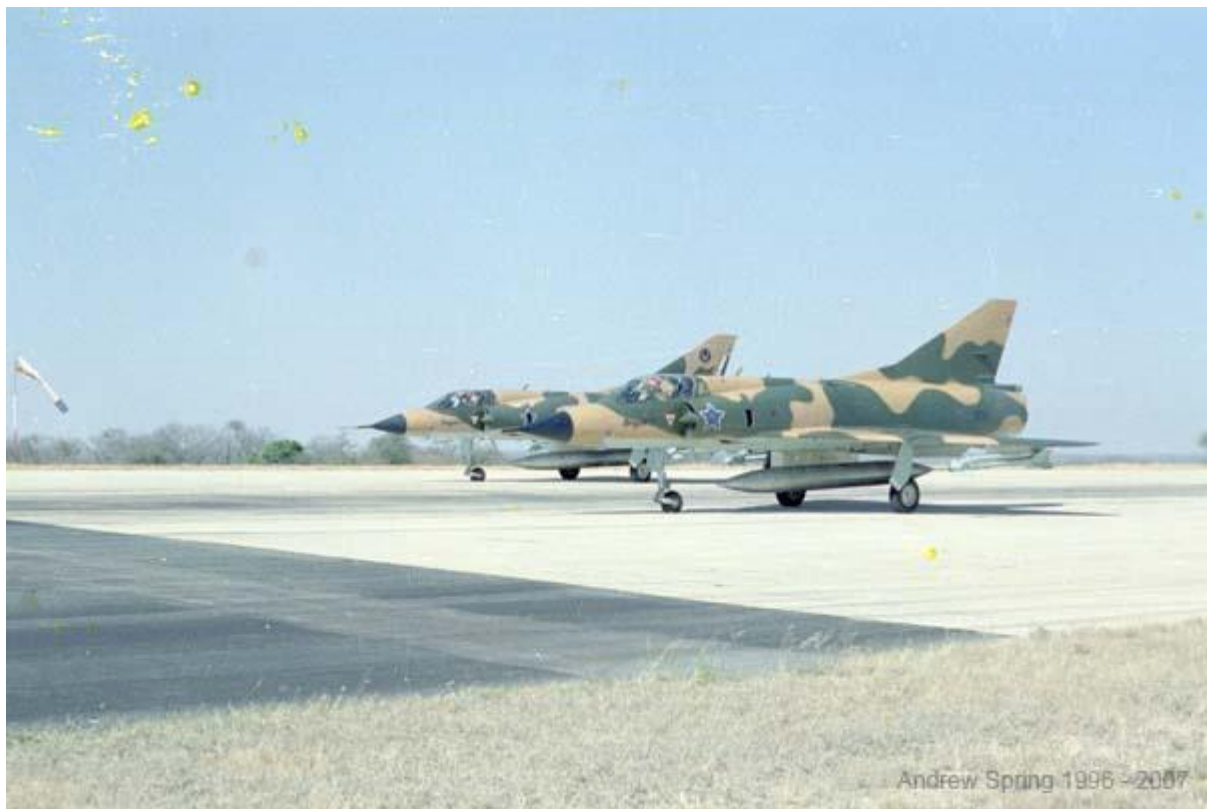
Two CZs in the later soft edge buff/green camouflage waiting to take off. Both aircraft are fitted with radar noses. The front CZ has the entire nose cone painted in buff whilst the second CZ has the camouflage running through the nose cone (buff upper, light grey lower)
