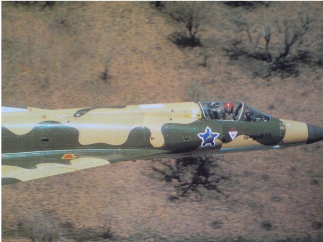
Unidentified CZ #803 in hard edge buff/green camouflage. Note that the green camouflage flows onto the nose cone and that the light blue grey underside colours follows through onto the nose cone. Note the black ring between the dark grey radome and the buff nose cone. Other interesting details are the large ejection warning triangle beneath the canopy (with the stylized canopy in red above this), the fuselage Castle on the forward part of the intakes, the red and yellow air brake, the white conformal antennae and the stenciling aft of the canopy for the canopy emergency release mechanism.
