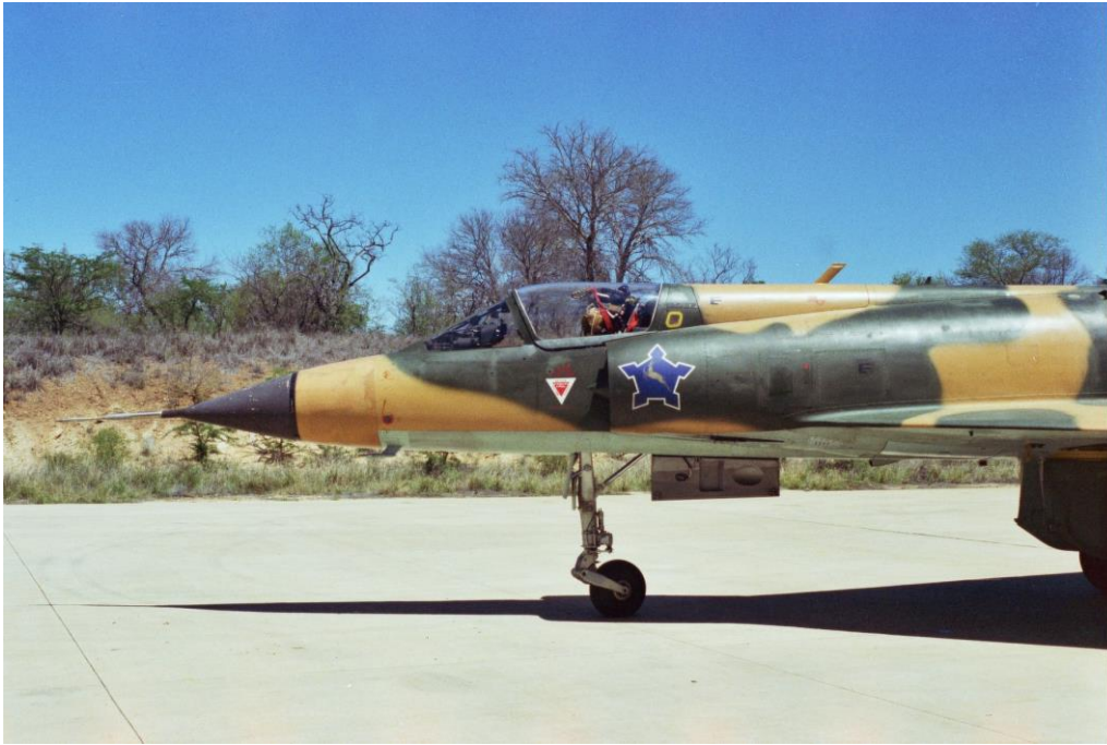
Photo of CZ forward fuselage showing some interesting detail : soft edge matt camouflage in what appears to be the original pattern; radome faded to a dark grey; distinct gloss black radome backing ring; full buff nose cone; Castle well forward on the air intake. The standard ejections eat warning triangle and stylized red canopy markings are present. The yellow shape aft of the cockpit denotes the emergency canopy release handle. Note as well the presence of the newer blade antenna on the upper fuselage. Mirage IIICZ has been removed from the forward fuselage.
