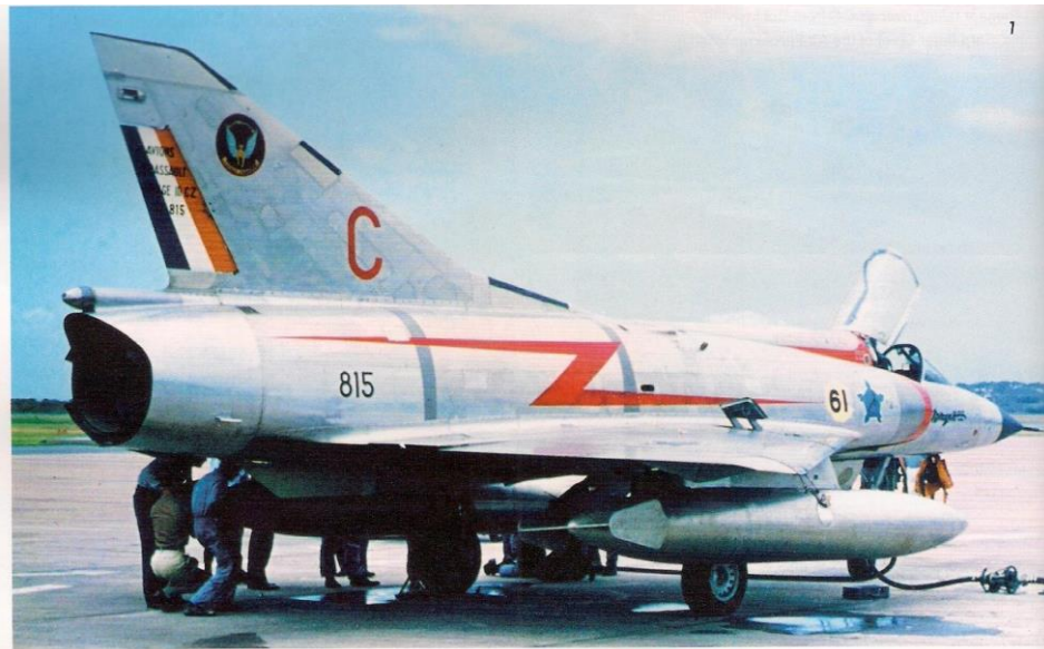
CZ #815 with a yellow circle with black 61 just aft of the fuselage national insignia. This was a temporary marking applied for an air race. The fuel tanks are the 1,300 liter RP62 subsonic type.
