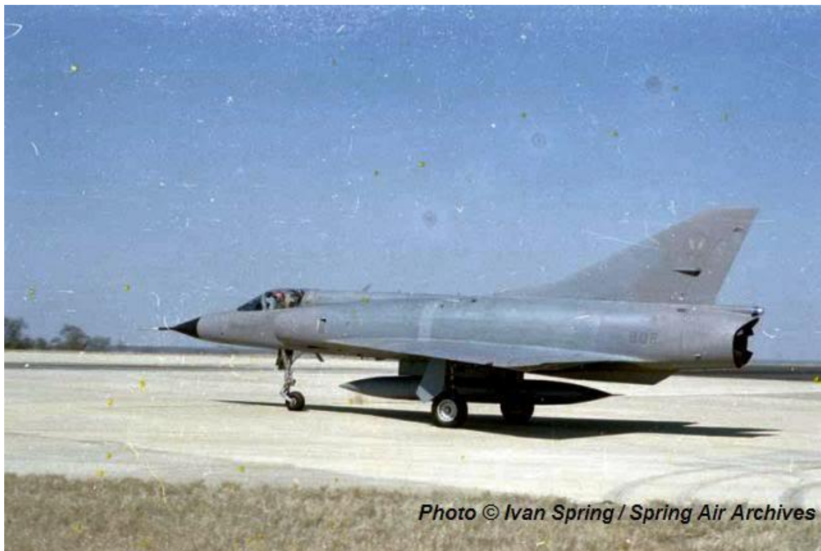
CZ #808. Fuselage Castle and 2 Squadron badge are visible. An RP825 fuel tank is located on the centerline.
