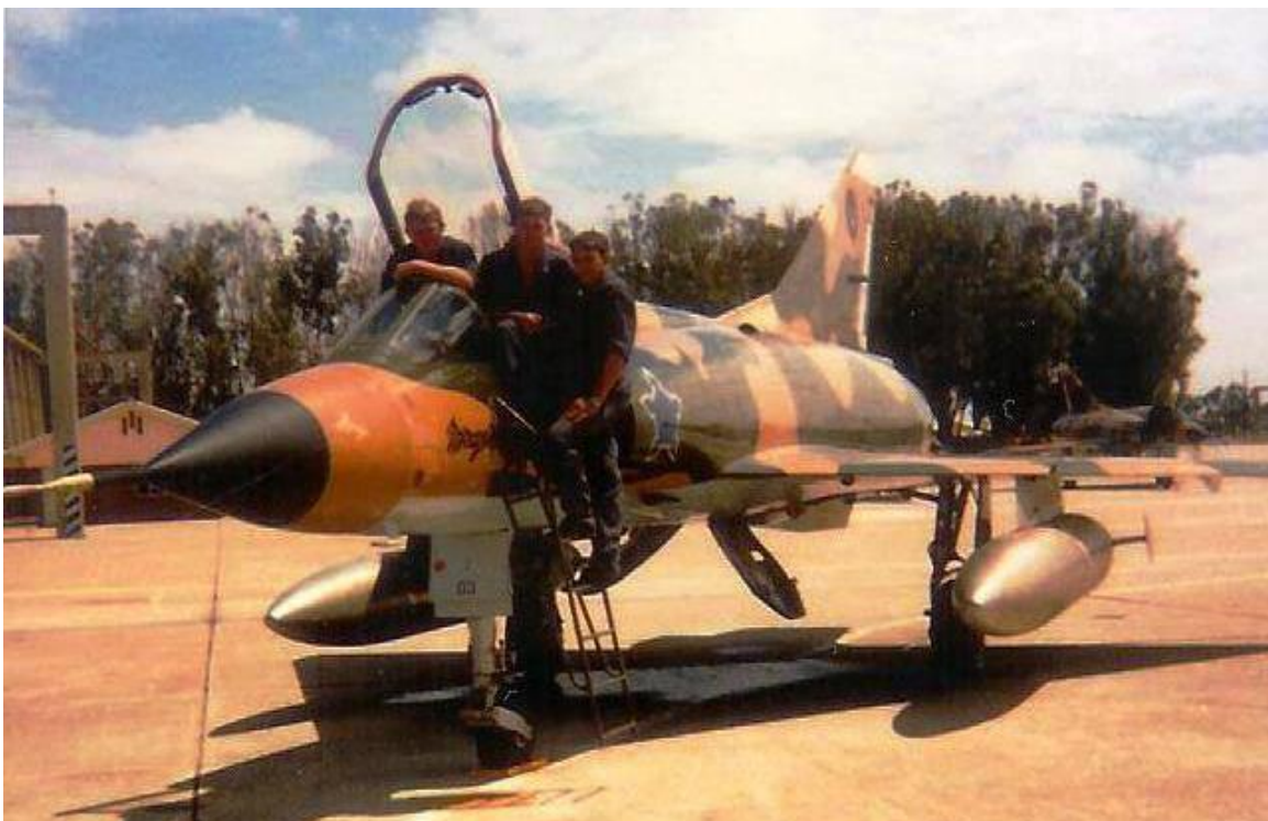
CZ #803 in hard edge buff/green camouflage and full buff nose cone which is clearly a different hue to the buff on the rest of the aircraft. #803 is fitted with 1,300 liter RP62 wing tanks. When the outboard missile pylons are not fitted, an aerodynamic fairing is installed to cover the elevon actuator.
