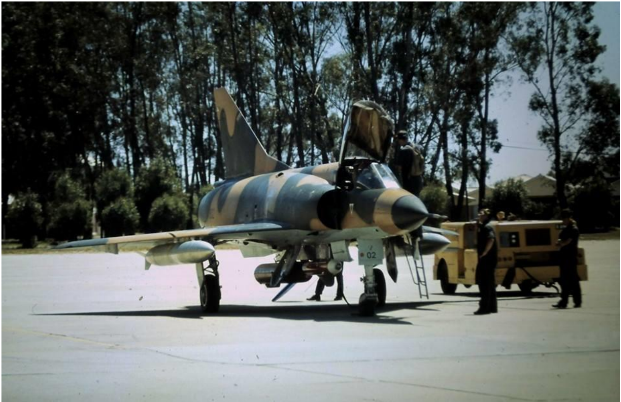
CZ #802 in soft edge buff/green camouflage (revised pattern) devoid of fuselage Castles, 2 Squadron badge or rudder flash. This aircraft is carrying what appears to be an aerial target-towing pod on the centerline. Aircraft has solid buff nose cone. The wing tanks are the 110G 500 liter type which can be used for supersonic flight. The three fins, as can be seen at the rear of the tank, allowed the 110G to be ejected in flight (unlike the RP18R tanks). The 110Gs are unpainted natural metal. The outboard wing pylons have been installed.
