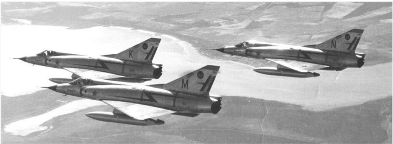
Three CZs : #'s 810 (K), 811 (M), and 812 (N) demonstrating the final natural metal markings. Note the clamshell engine exhaust arrangement, which was characteristic of the Atar 09B engine fitted to the BZ and CZ. Another distinctive feature of the BZ and CZ is the extended fillet to the lower leading edge of the vertical stabilizer. This fillet was not present on the D, D2Z, E, RZ and R2Z.
