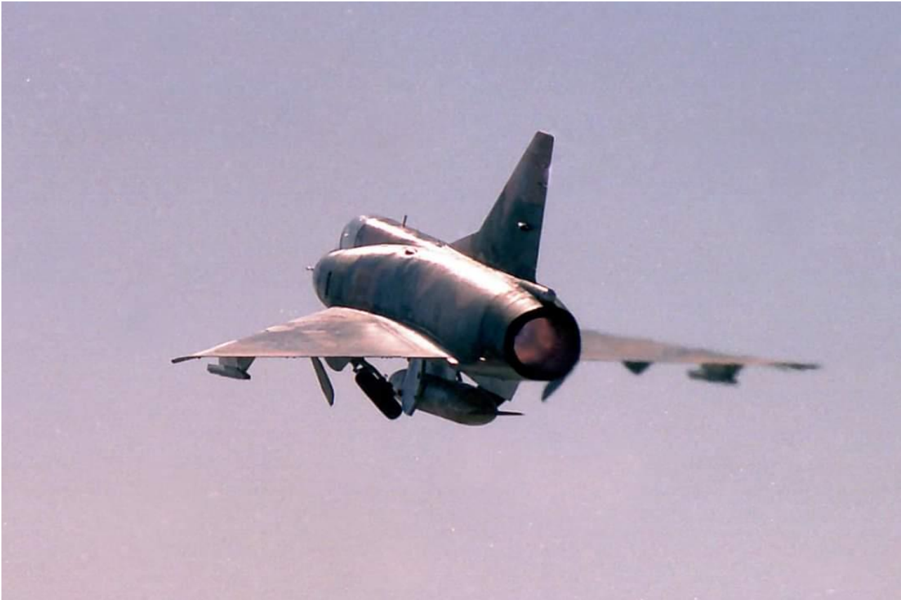
CZ fitted with centerline RP825 fuel tank and missile launchers on the wing outboard pylons.
