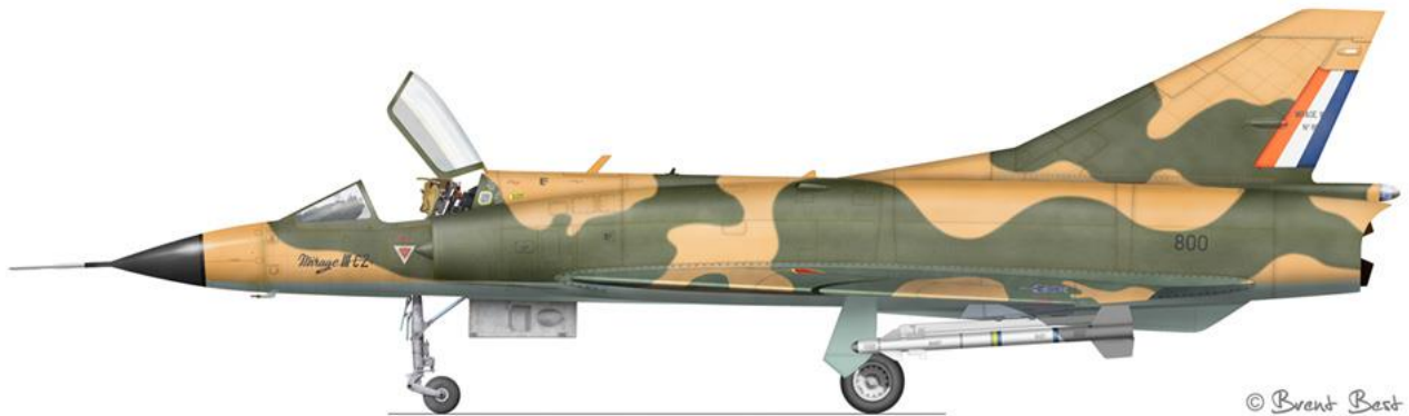
CZ #800 repainted in soft edge buff/green camouflage (original pattern) with rudder orange/white/blue flash but no Castles. Note that the Matra R550s presented in these profile images were not actually used on the CZ. The CZ used the AIM-9B and V3B missiles.
