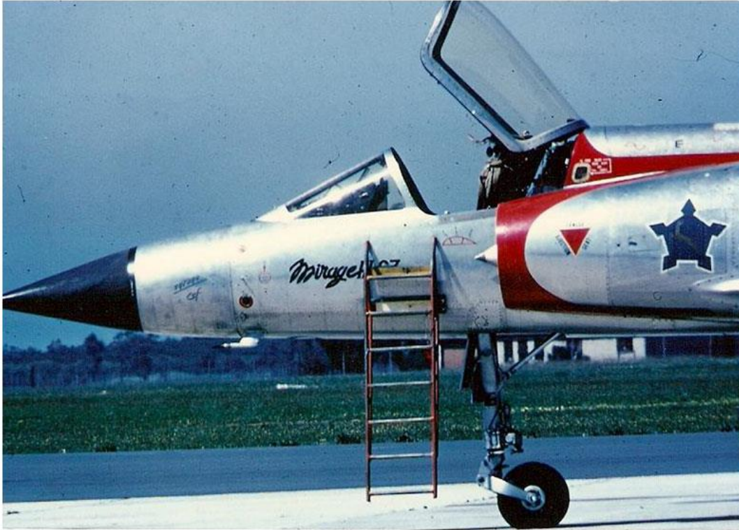
Unpainted natural metal CZ with radar installed as indicated by the black radome with unpainted natural metal nose cone. Note "Cyrano CSF" on the nose cone. Of interest is the early location of the ejection seat warning triangle on the intake. This was later moved to just beneath the cockpit ahead of the intake.
