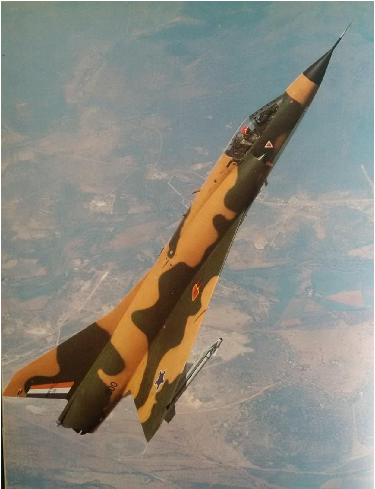
CZ #800 in soft edge buff/green camouflage (original pattern). Interesting items to note : Blue/white/orange rudder flash with text "MIRAGE III CZ / N°. 800", SAAF Castles on wings but not intakes and solid buff nose cone. All conformal antennae have been painted over. The aircraft displays standard markings and warning data around the forward fuselage. The airbrakes are in standard red with yellow edging. A "no step" boot print can be seen on the airbrake. A similar marking can be seen on the center control surface aft of the wing Castle. Mirage III CZ no longer appears on the forward fuselage. The silver round object on the upper fuselage in line with the airbrake is the starboard fuel filler cap. #800 has the newer blade antenna on the fuselage spine. The missile is a V3B.
