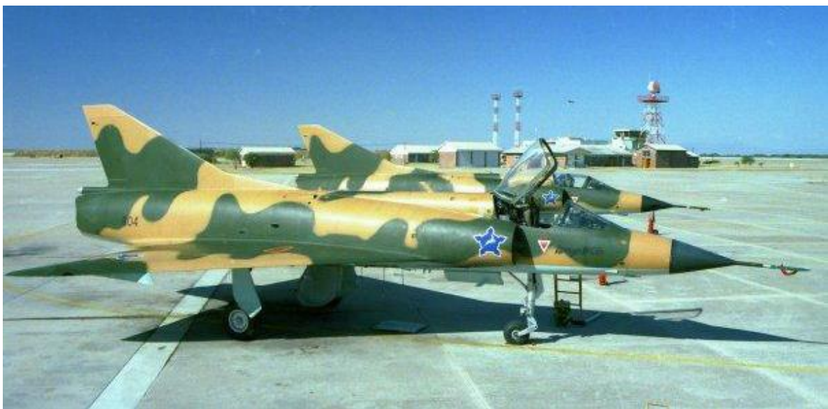
CZ #804 finished in soft edge buff/green camouflage (original pattern). Both wing and fuselage Castles are present. Mirage IIICZ can be seen on the nose of #804 but appears to be missing from the nose of the rear CZ. The airbrakes are standard red with yellow edging. Nose cone is finished in buff upper and blue lower surface. Note the blade antennae on the fuselage spine and on the nose gear door. #804 carries a missile pylon on the outboard wing hard point.
