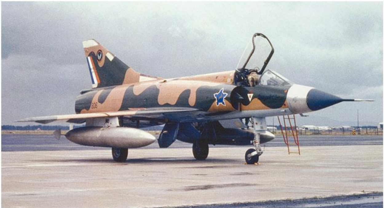
CZ #806 in hard edge buff/green camouflage and with an unpainted natural metal nose cone. Some aircraft in this configuration retained the text " Cyrano CSF " in black script on the natural metal nose cone as can be seen in this image. Note how the black radome colour carries forward onto the pitot probe. The colour of the dielectric panels looks to be cream in this image but were more than likely off-white or very light grey.
