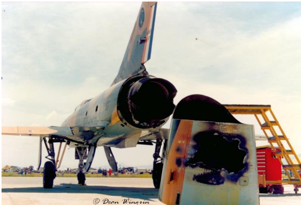
BZ #817 with damaged rear fuselage section.
