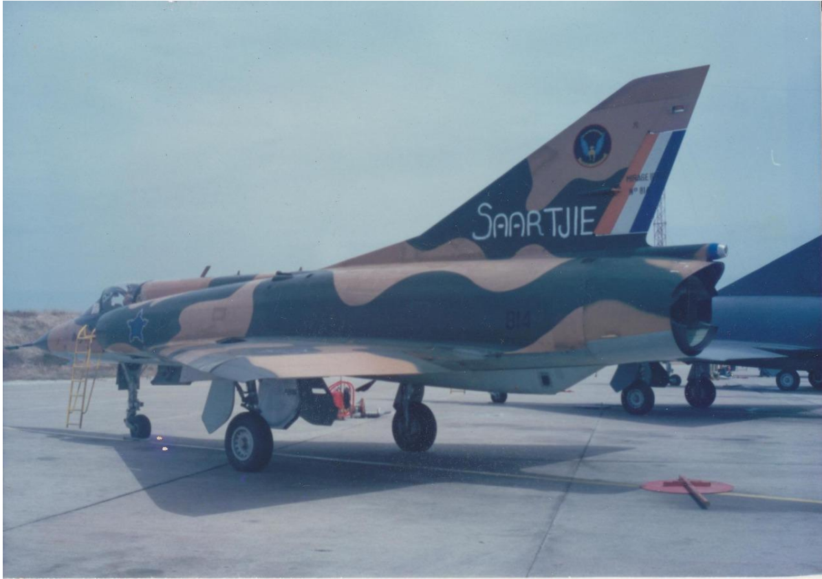
CZ #814 with "Saartjie" on the vertical stabilizer – personalized art on SAAF Mirage IIIs appears to have been a rare occurrence. #814 is in the hard-edge buff/green camouflage. However, looking closely at the rear fuselage, the section around the engine exhaust appears to be a replacement part painted in the later soft edge camouflage. Note the step in the line between upper buff and lower blue. The fuselage Castle is also located further back on the intake. The drag chute cone is natural metal with a metallic blue front section. It has clearly been used before as witnessed by the dented rear end. Note that the off-white conformal dielectric panels have all been painted over.
