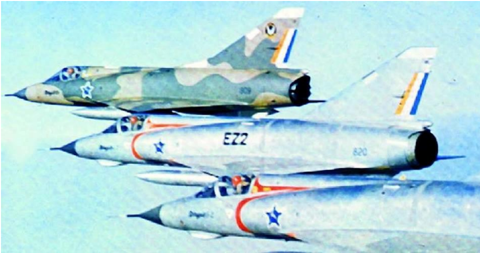
CZ #809 in the experimental dark brown / green camouflage in company with two natural metal EZs. #809 retains all the high visibility markings with the fuselage Castles located far back on the intakes. Mirage III CZ remains on the forward fuselage.
