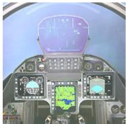
State of the art: The Gripen has an "all-glass" cockpit with no analogue instruments.
